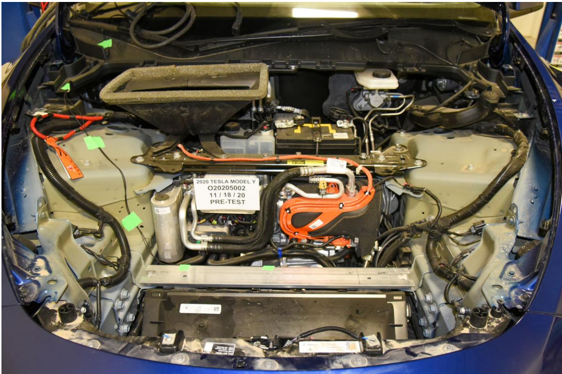
FIGURE 305-019. Pre-Impact View Propulsion Battery Venting System(s)
