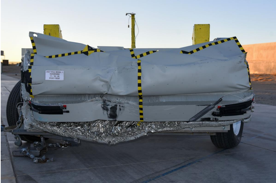
FIGURE 85. Post-Test Front View of MDB Impactor Face
