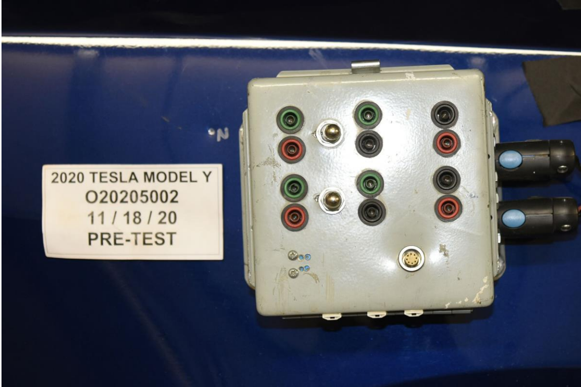
FIGURE 305-024. Pre-Impact View of Installed Test Interface Port
