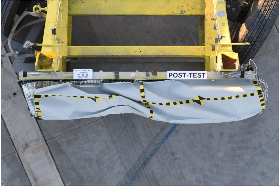
FIGURE 87. Post-Test Top View of MDB Impactor Face
