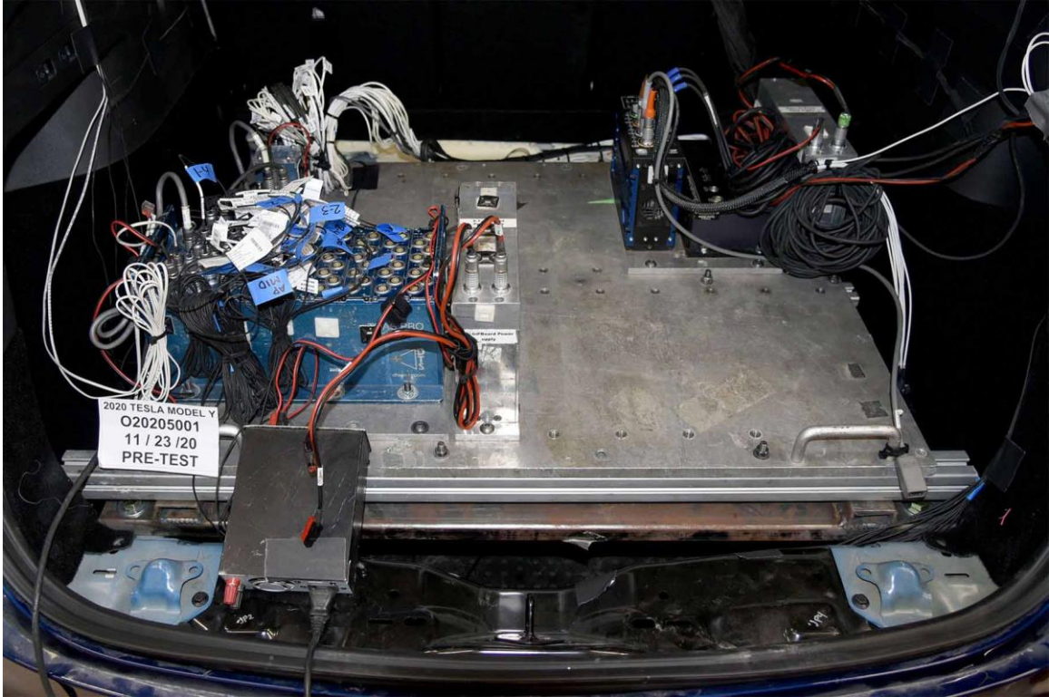
FIGURE 61. Pre-Test Ballast View
