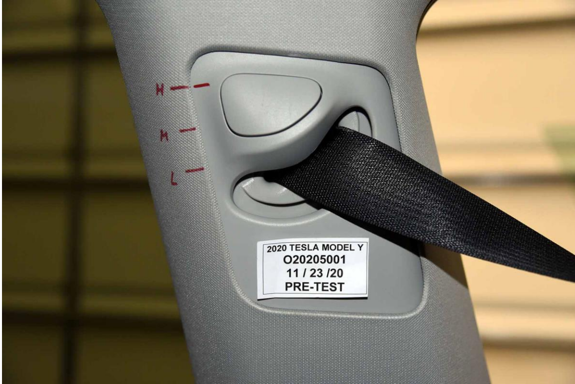
FIGURE 33. Pre-Test View of Belt Anchorage for Dummy
