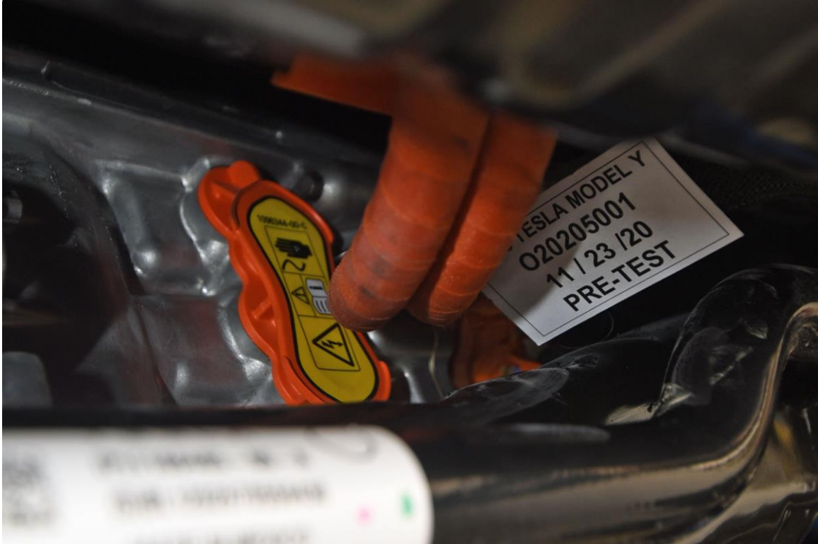
FIGURE 305-02b. Power Inverter Warning Label
