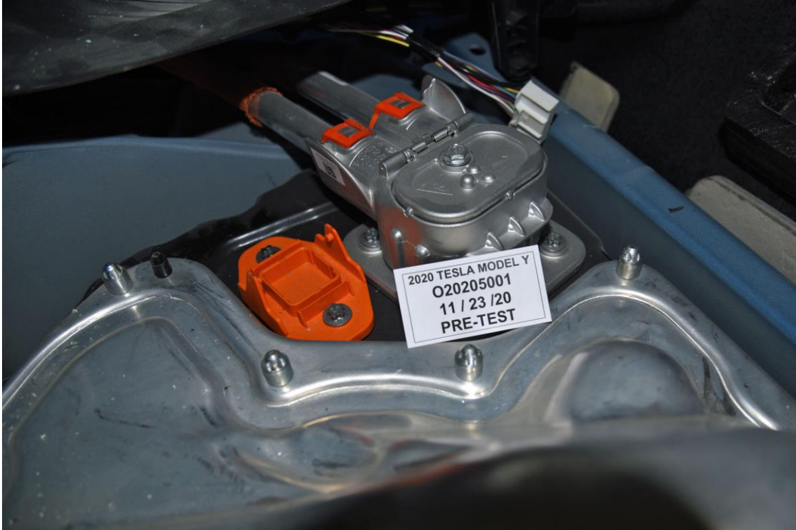
FIGURE 305-018. Pre-Impact View of High Voltage Interconnect(s)
