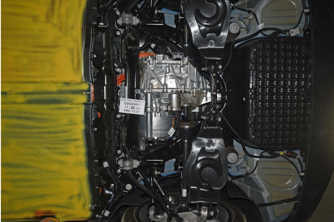
FIGURE 305-016. Pre-Impact View of Electric Propulsion Drive
