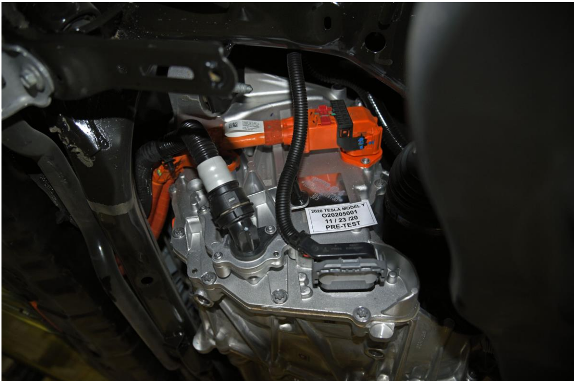
FIGURE 305-018a. Pre-Impact View of High Voltage Interconnect(s)
