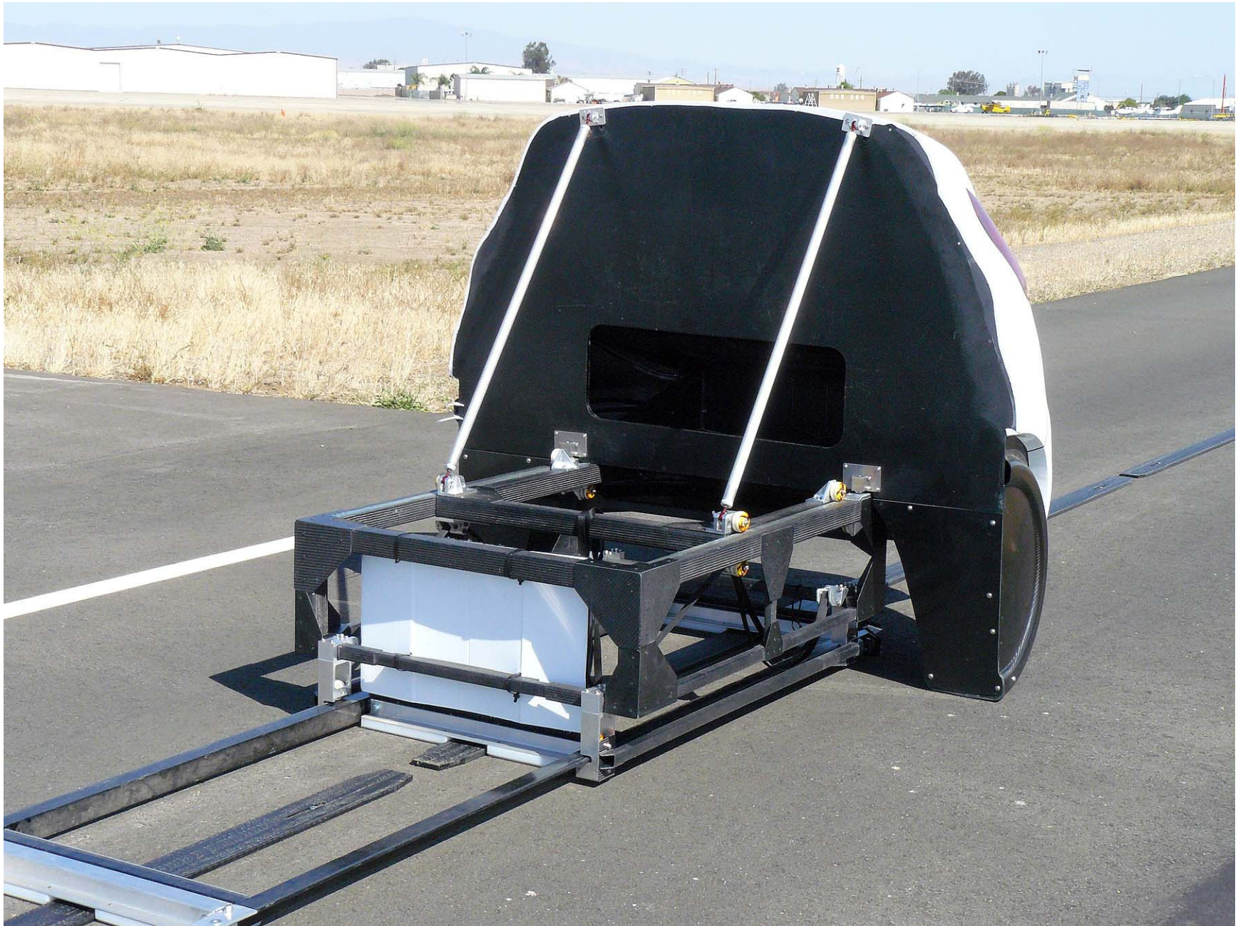
Figure A7. Load Frame/Slider of SSV
