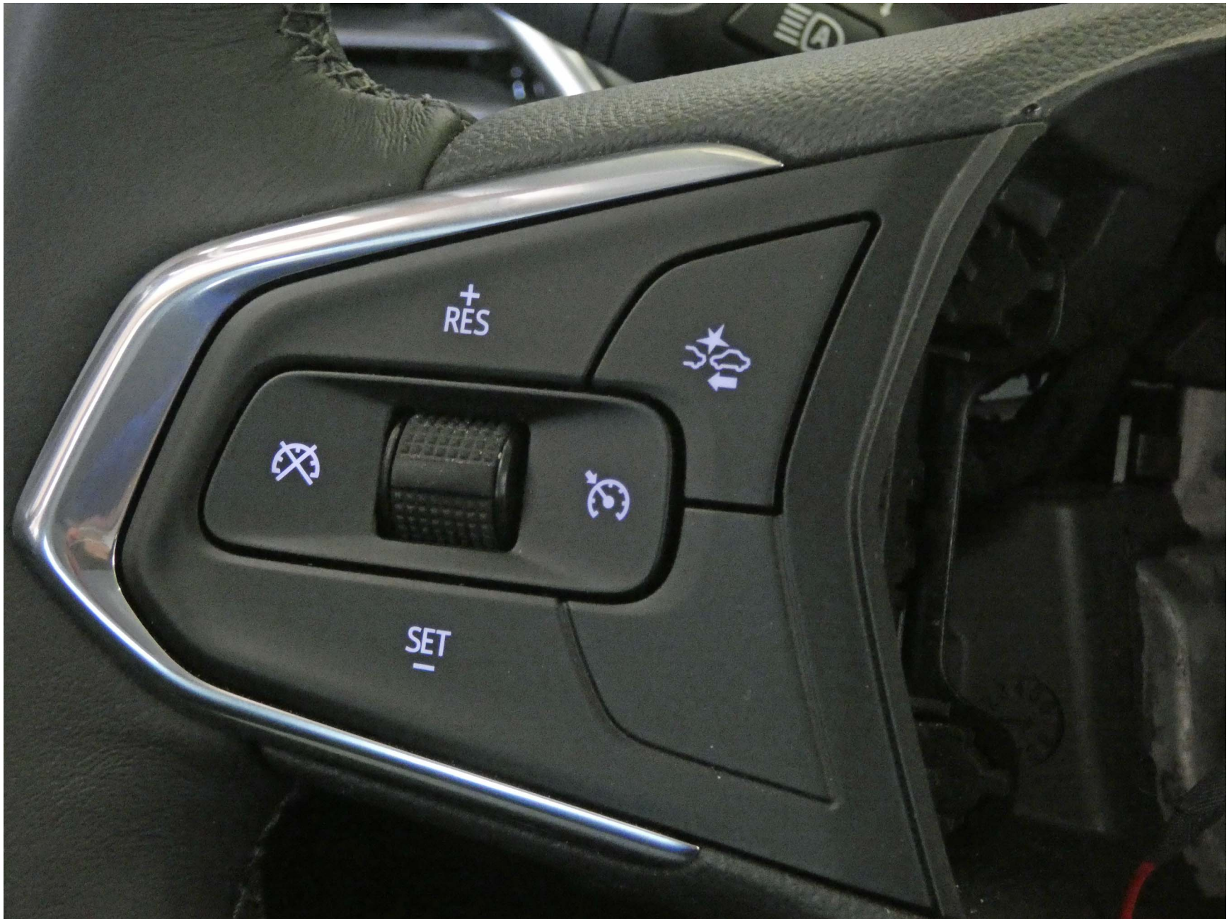
Figure A14. FCW System Range Setting Button
