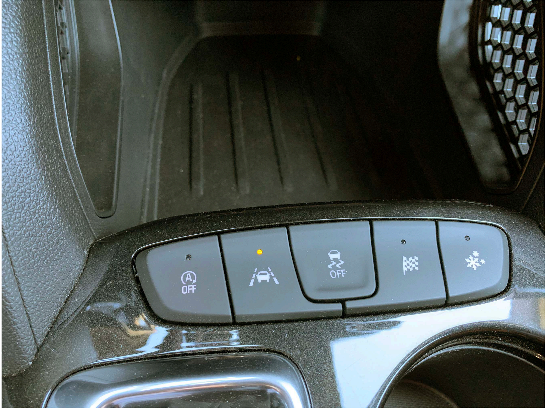
Figure A11. LDW on/off Switch
