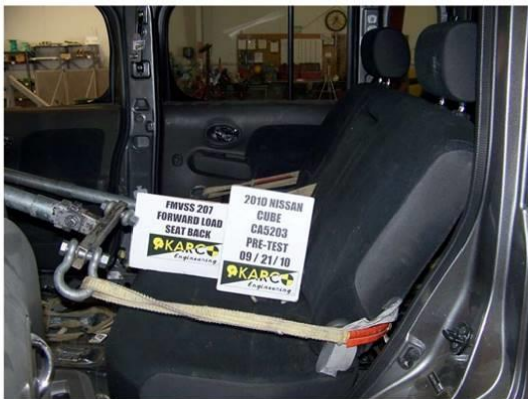
FIGURE 31. Forward Load on Seat Back, P4, Pre-Test
