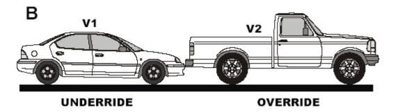
When the bumper receives measurable crush and the area above the bumper also receives measurable crush, the override/underride codes are applicable if the impact configuration applies.
