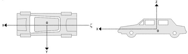
The x-axis is on the longitudinal centerline of the vehicle. This could be set up along the transmission drive shaft tunnel for a rear wheel drive vehicle or along a centerline which is equidistant from the sides of the vehicle in a front wheel drive vehicle.
