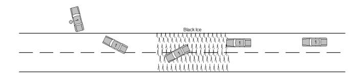
Vehicle 1 is traveling on a two lane roadway with moderate snow falling. The driver suddenly encounters black ice on the roadway, loses control, and begins to rotate counterclockwise. The driver attempts to regain control by braking and steering right, but overcorrects and the vehicle departs the right side of the roadway and strikes a pole. There were no indications of distractions identified by police on the crash report or during CISS interviews.
