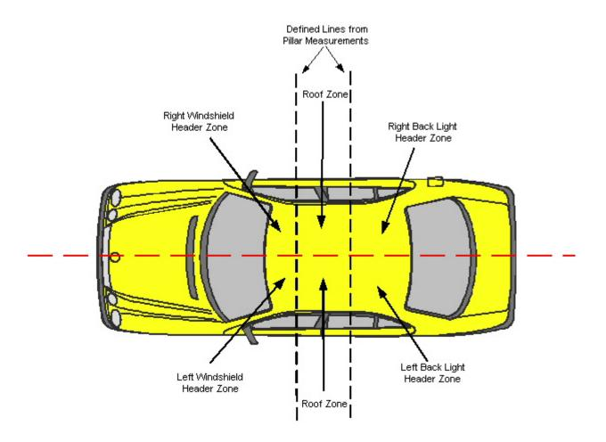
The defined zones created in the Side Plane measurement protocol should be extended onto the Top Plane. This allows for the Top Plane to be zoned as the above illustration depicts. The Roof Zone is the entire area from Windshield Header Zone to the Back Light Header Zone.
