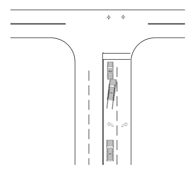
Vehicle 2 is stopped waiting to turn left in a left turn lane at an intersection controlled by a traffic signal. Vehicle 1 approaches the intersection and the driver is texting. Vehicle 1's driver looks up at the last minute and brakes and steers right leaving tire marks, but cannot avoid striking the rear of Vehicle 2. There were no indications of distractions identified by police on the crash report or during CISS interviews for the driver of Vehicle 2.
