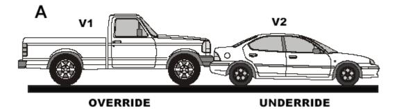
As indicated in **Situation A**, the trunk area of V2 is damaged (i.e., "crushed") while the rear bumper is relatively undisturbed. This explains the uneven damage pattern. Conversely, the front of V1 is "crushed" at bumper height only, or is crushed *uniformly* at the bumper and grille levels (i.e., an "even" damage pattern). Even though V1 may not exhibit the uneven damage pattern, it would still receive an applicable override code due to the resultant underride damage to V2.
