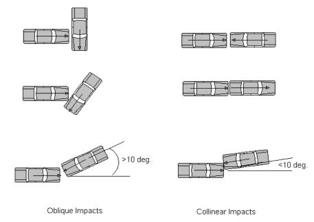
The transition between the axial and angular solutions (i.e., a velocity vector change from within ten degrees of parallel to just outside ten degrees of parallel) may sometimes produce abrupt changes in Delta V results. Therefore, the technician should remember to examine the results carefully.
