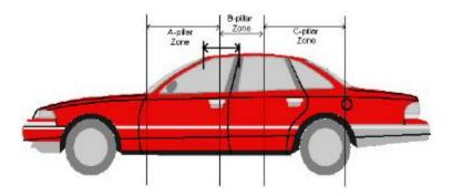
The defined zones created in the Side Plane measurement protocol should be extended onto the Top Plane. This allows for the Top Plane to be zoned as the above illustration depicts. The Roof Zone is the entire area from Windshield header Zone to the Back Light Header Zone.
