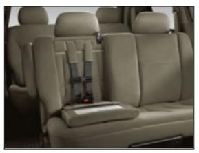
Older 5-point harness type of integrated CRS (typically seen in many older minivans
