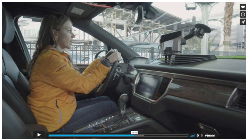
Images Aptiv driver monitoring system. The warning for inattentive drive is near the windshield. Green for paying attention and red for inattentive driving. (Vimeo)
