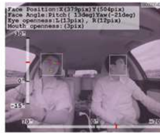
Monitoring both driver and front passenger
