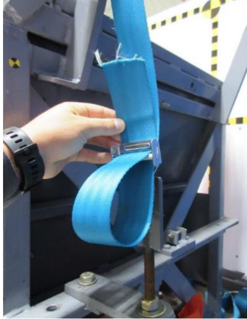
Figure 10: Loop Webbing Back Through the Rear Locking Belt Anchor
