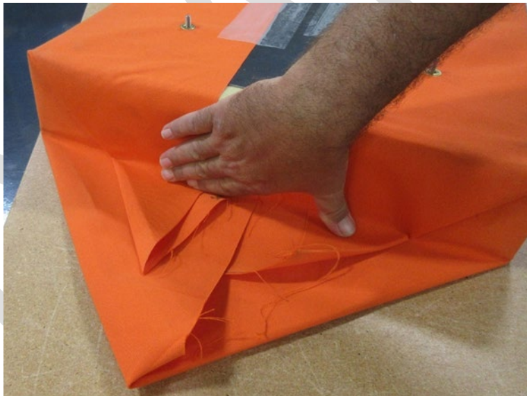
Figure D5: Top Piece of Fabric Folded Down
