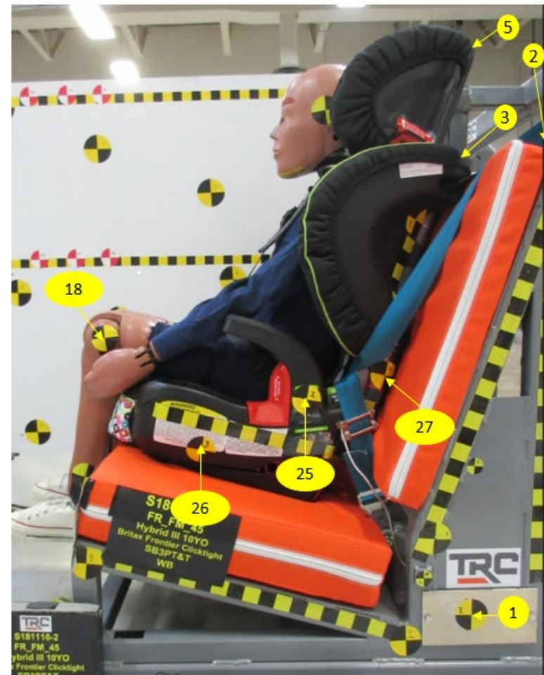
Figure E3: Target Schematic for Frontal Convertible/High Back Booster 6YO and 10YO
