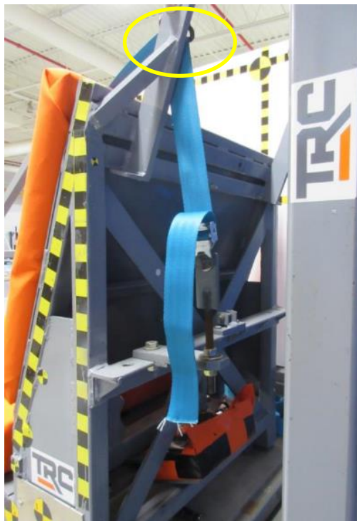
Figure 11: Slack Pulled Through the Slot
