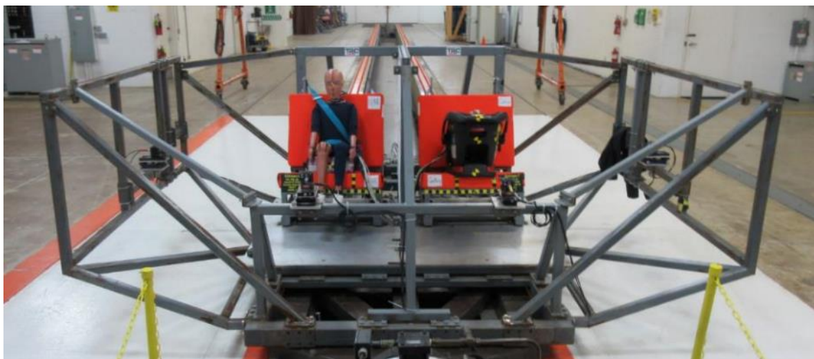
Figure 1: FMVSS No. 213 Frontal Sled Buck Assembly with Camera Wings
