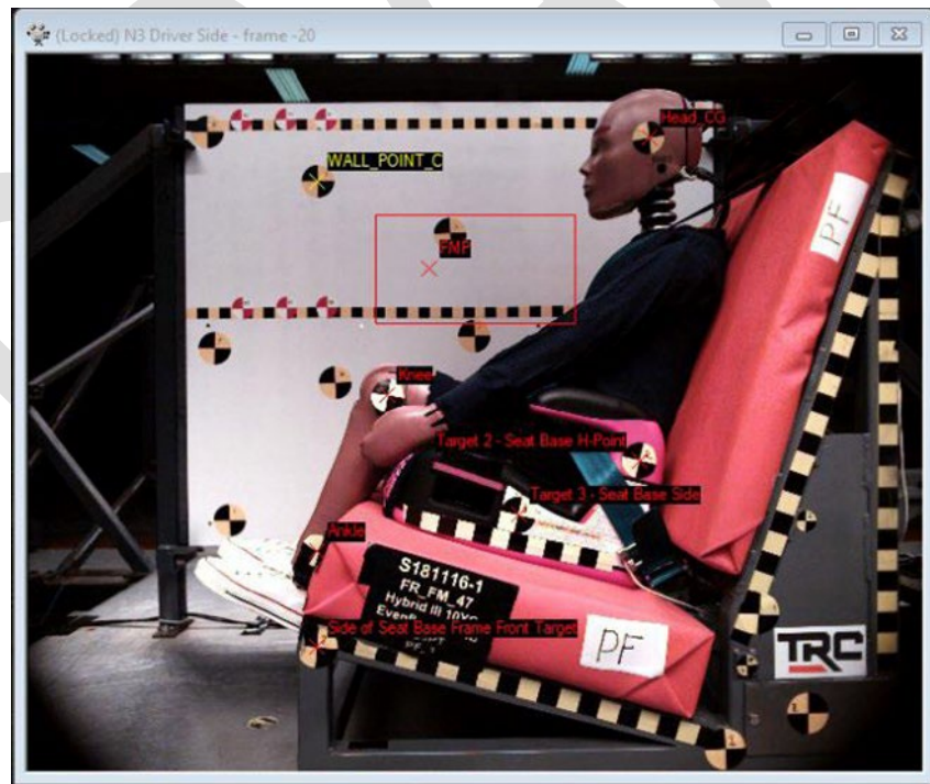
Figure B1: TEMA Analysis with Wall Targets and Additional Targets Identified
