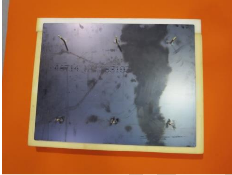
Figure D2: Foam Placed on Plate with 25 mm of Foam on Each Side
