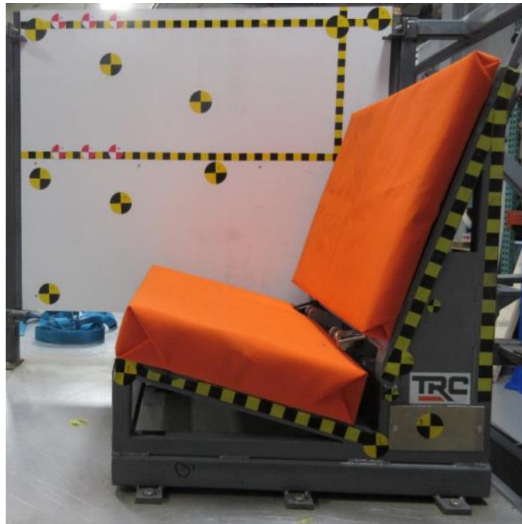
Figure 3: Seat Bench and Separation Wall Targets
