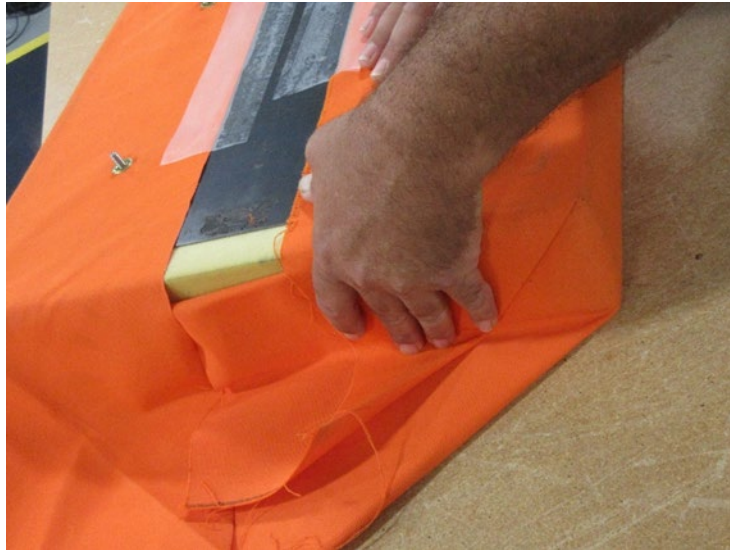
Figure D4: Fabric Pushed into Thickness of Foam
