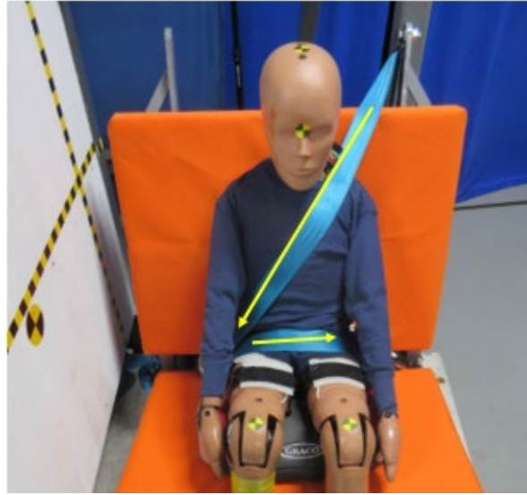
Figure 14: Belt Routed Over Shoulder, Through Inboard Anchor, and Over Lap
