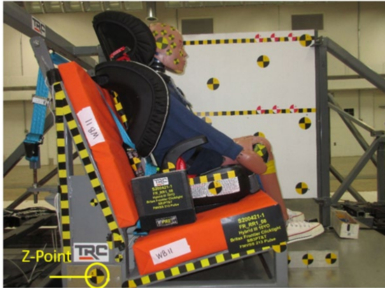
Figure 8: Z-Point Location on Sled Buck Assembly
