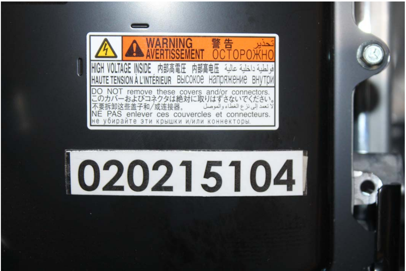
Photo No. 305-02 - Power Inverter Warning Label
