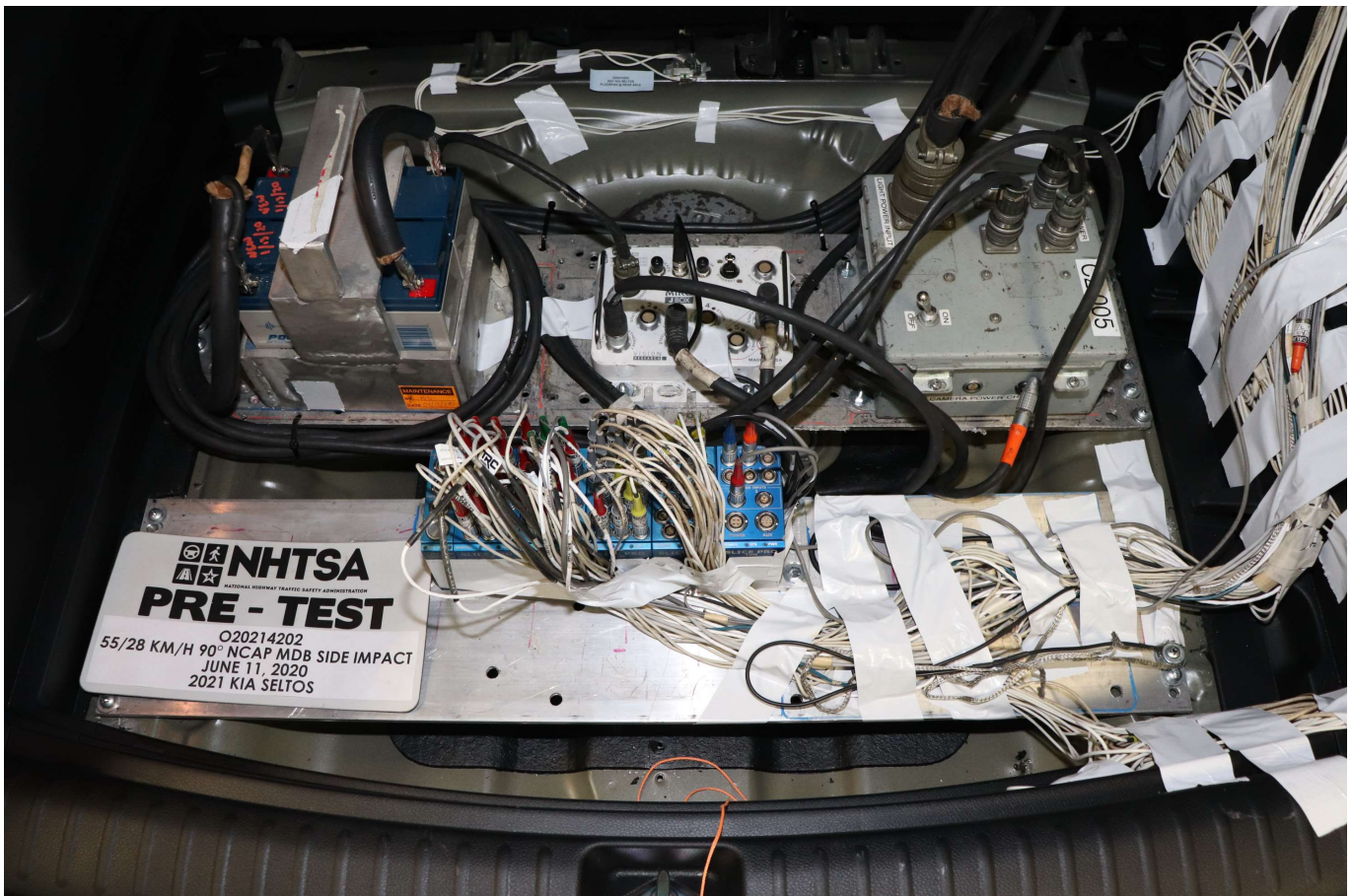
Photo No. 094 - Pre-Test Ballast View
