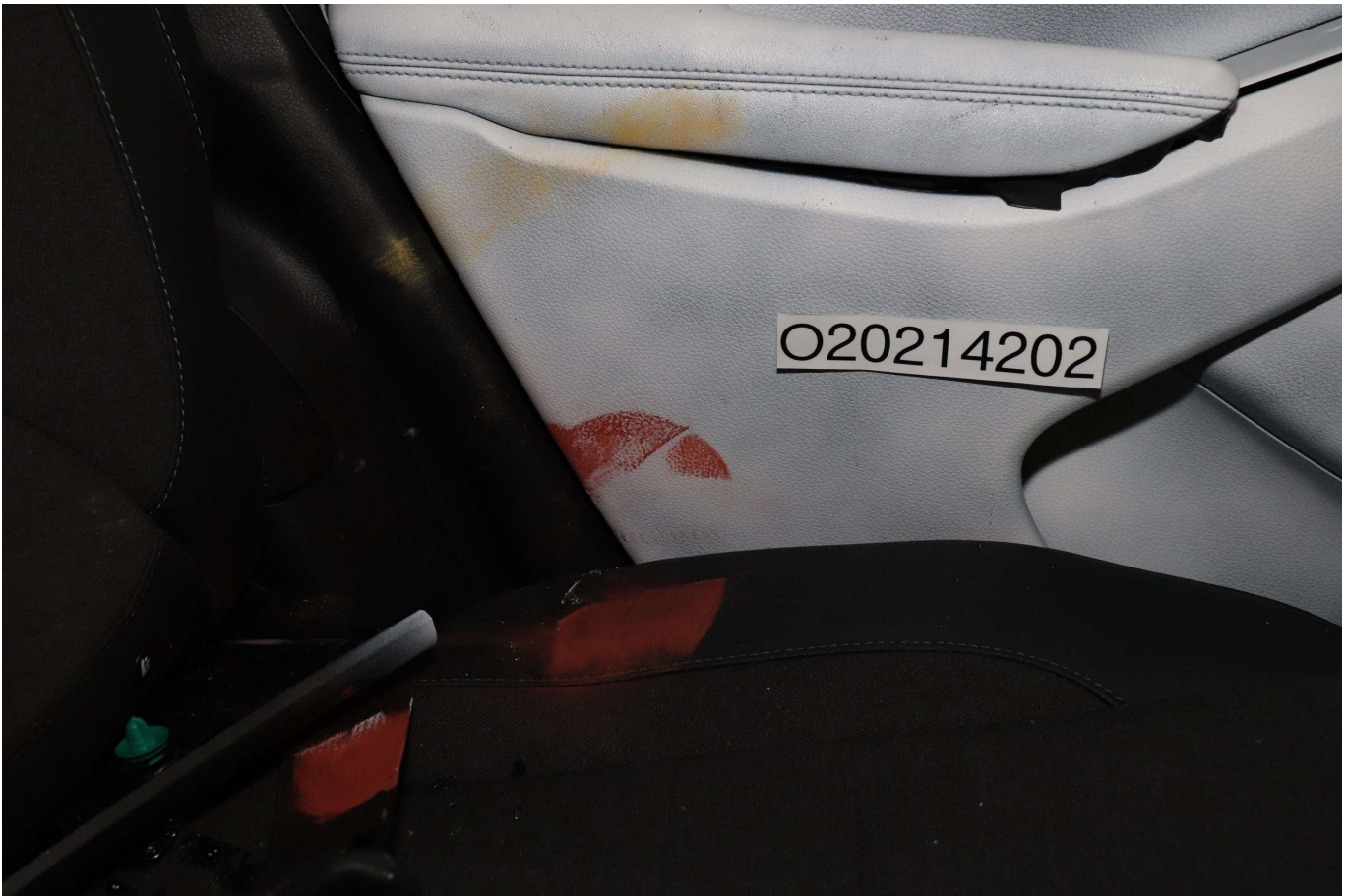
Photo No. 079 - Post-Test Rear Passenger Dummy Close-up Pelvis Contact with Vehicle Interior View
