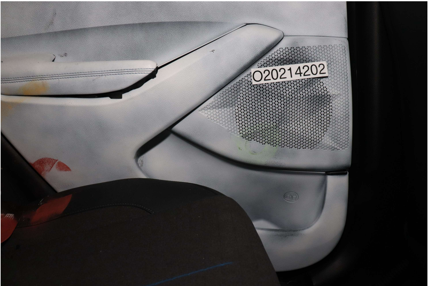
Photo No. 081 - Post-Test Rear Passenger Dummy Close-up Knee Contact View
