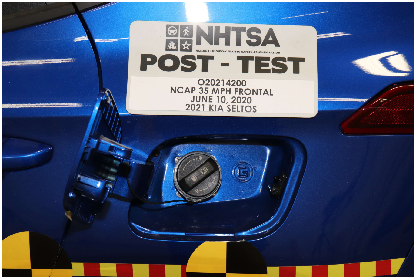
Photo No. 023 - Post-Test Fuel Filler Cap View
