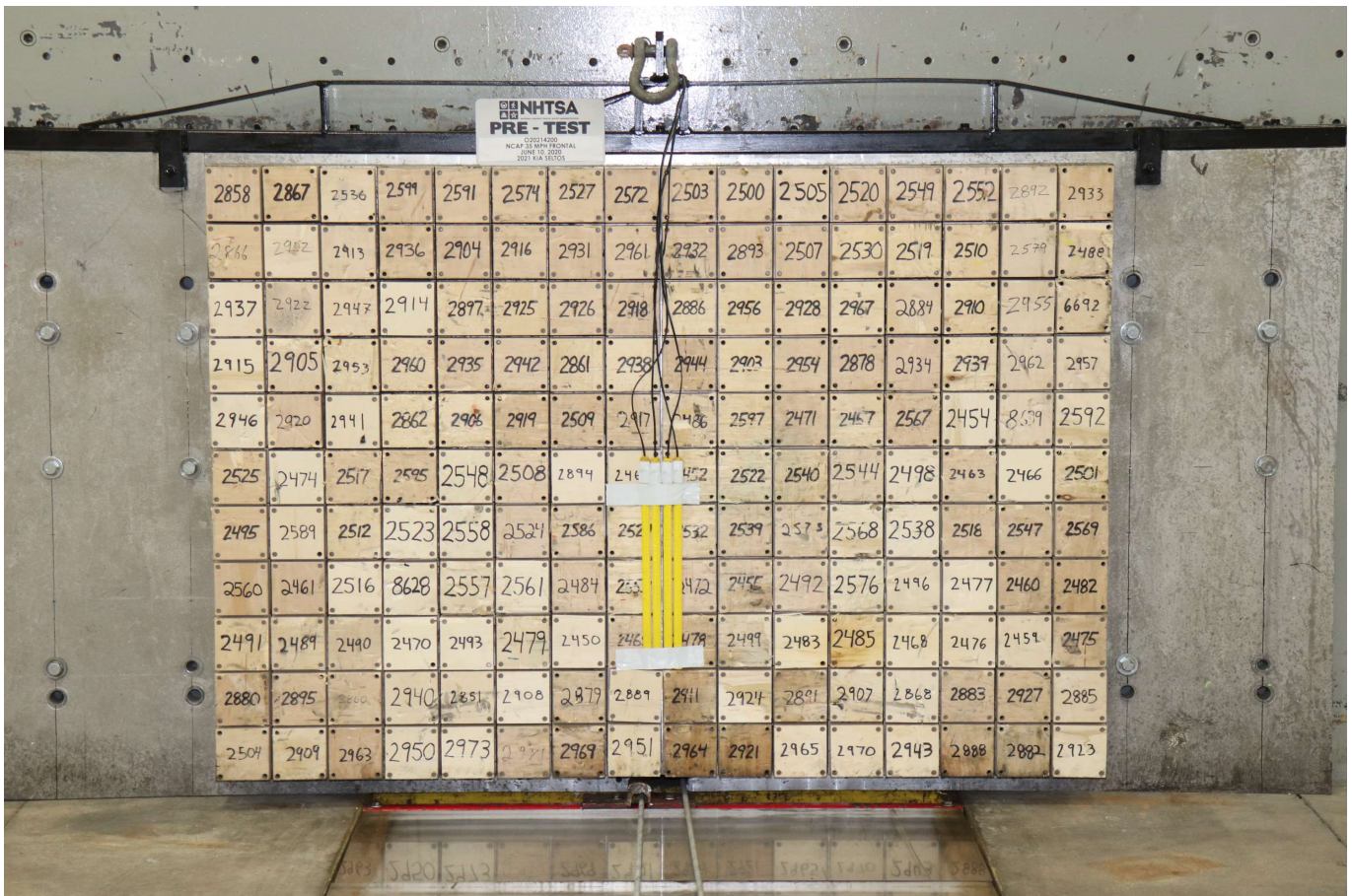
Photo No. 002 - Pre-Test Load Cell Wall
