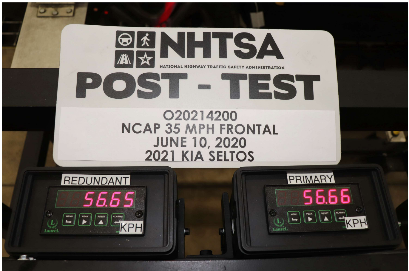
Photo No. 076 - Post-Test Speed Trap Read-Out
