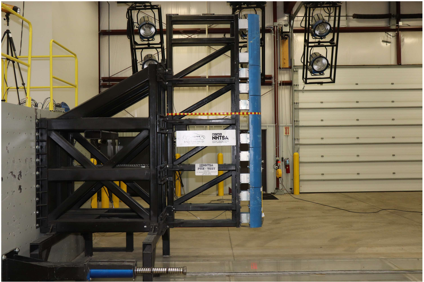
Photo No. 061 - Pre-Test Pole Barrier Side View
