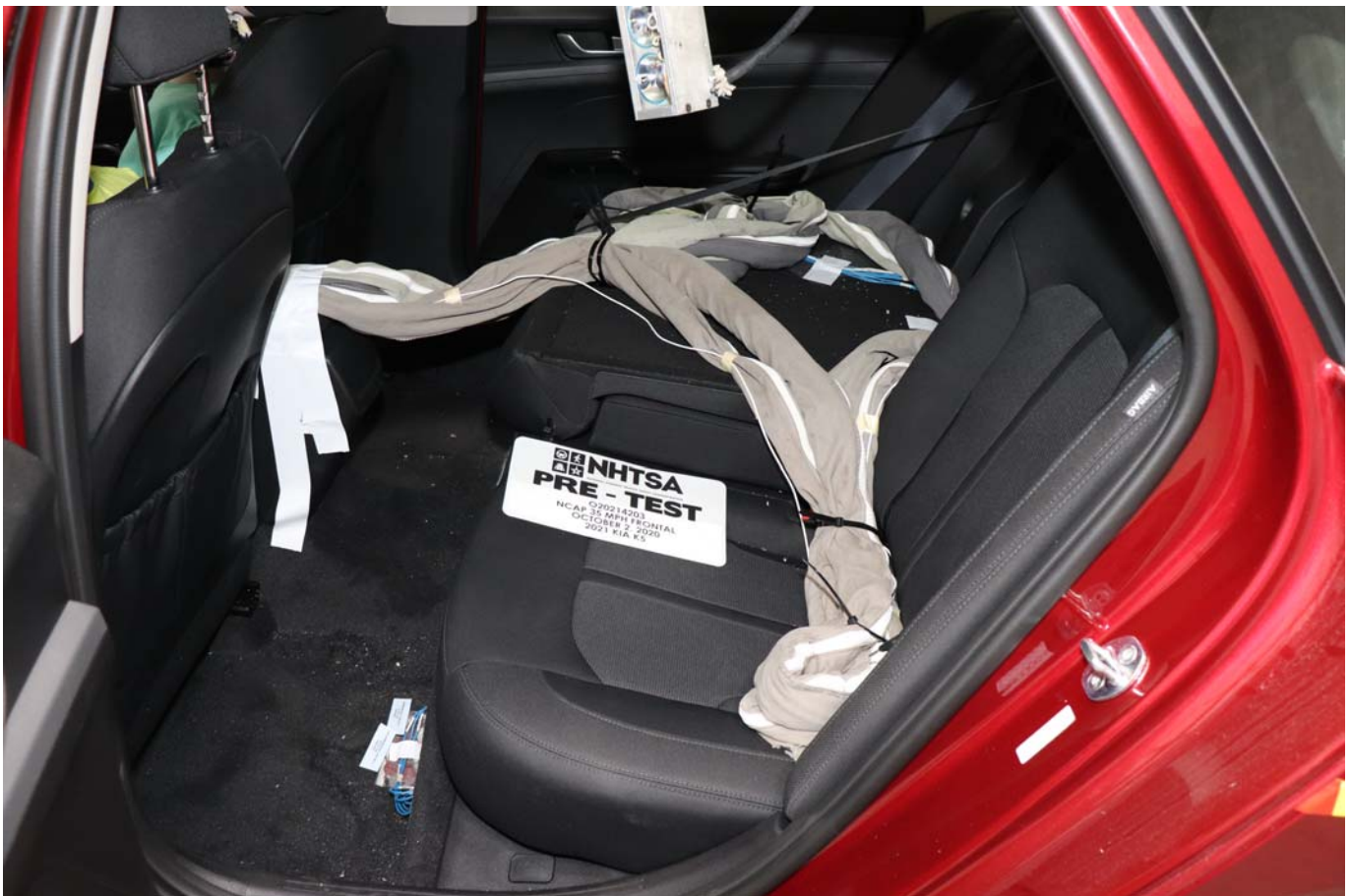
Photo No. 028 - Pre-Test Dummy Cable Routing
