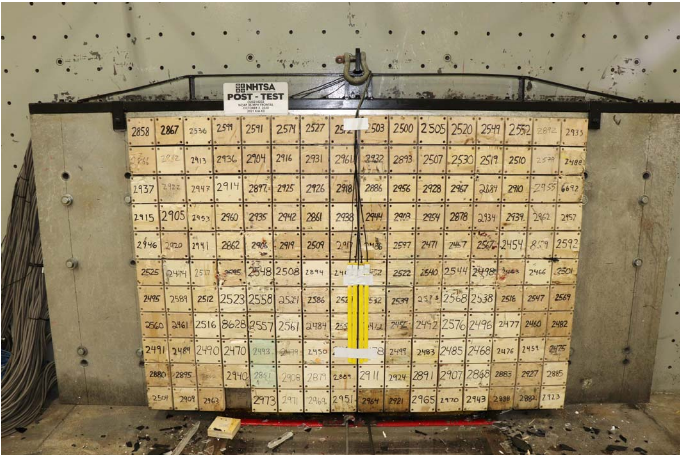
Photo No. 003 - Post-Test Load Cell Wall
