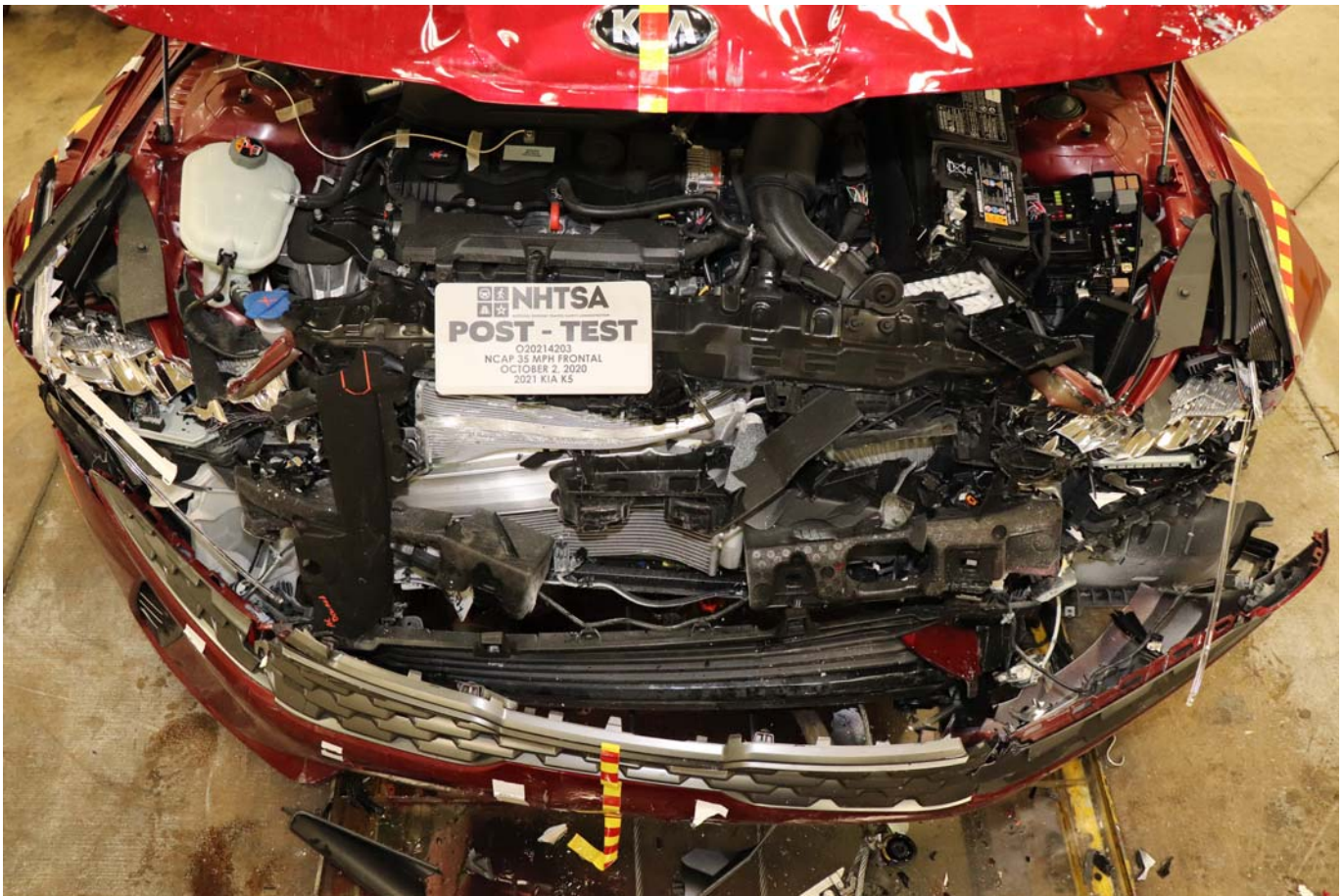
Photo No. 021 - Post-Test Engine Compartment View
