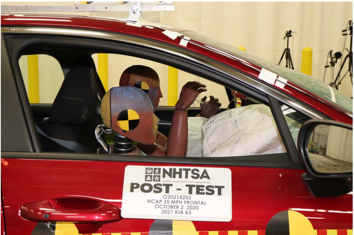
Photo No. 056 - Post-Test Passenger Dummy Window View
