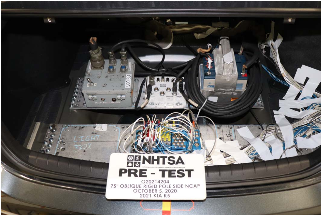
Photo No. 063 - Pre-Test Ballast View
