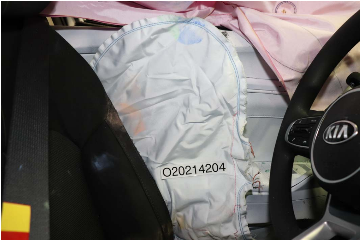
Photo No. 049 - Post-Test Dummy Close-Up Torso Contact with Side Air Bag View
