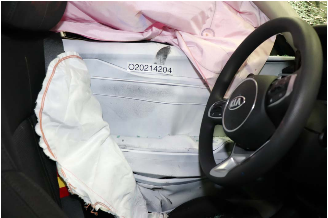
Photo No. 073 - Post-Test View of Shattered Vehicle Inner Door Panel
