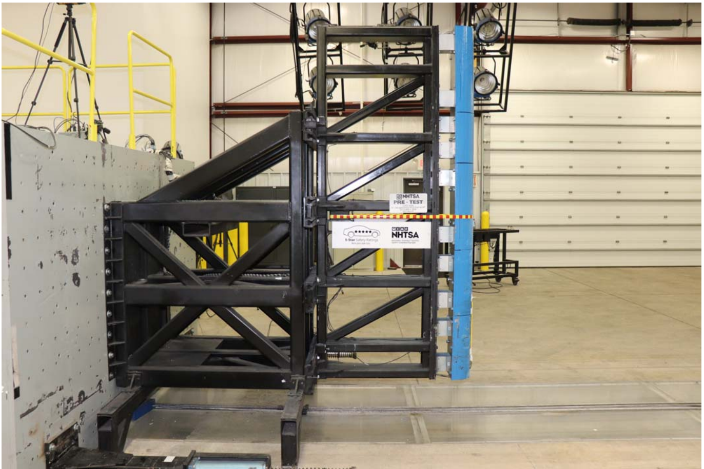
Photo No. 061 - Pre-Test Pole Barrier Side View
