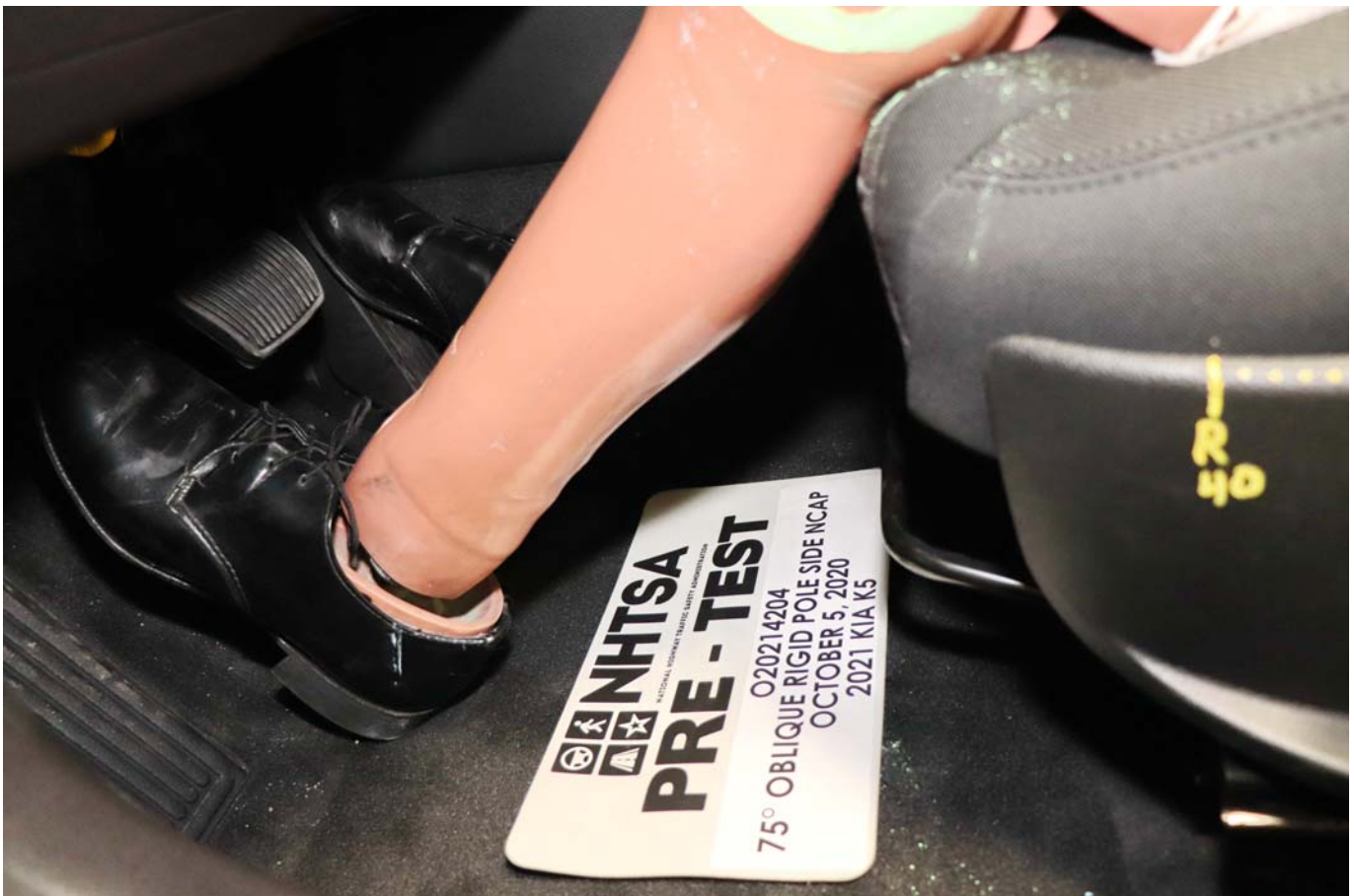
Photo No. 032 - Pre-Test Placement of Dummy Feet
