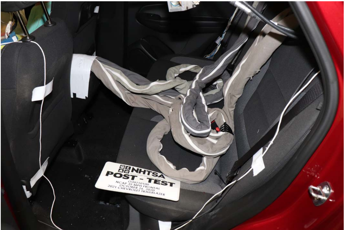
Photo No. 029 - Post-Test Dummy Cable Routing
