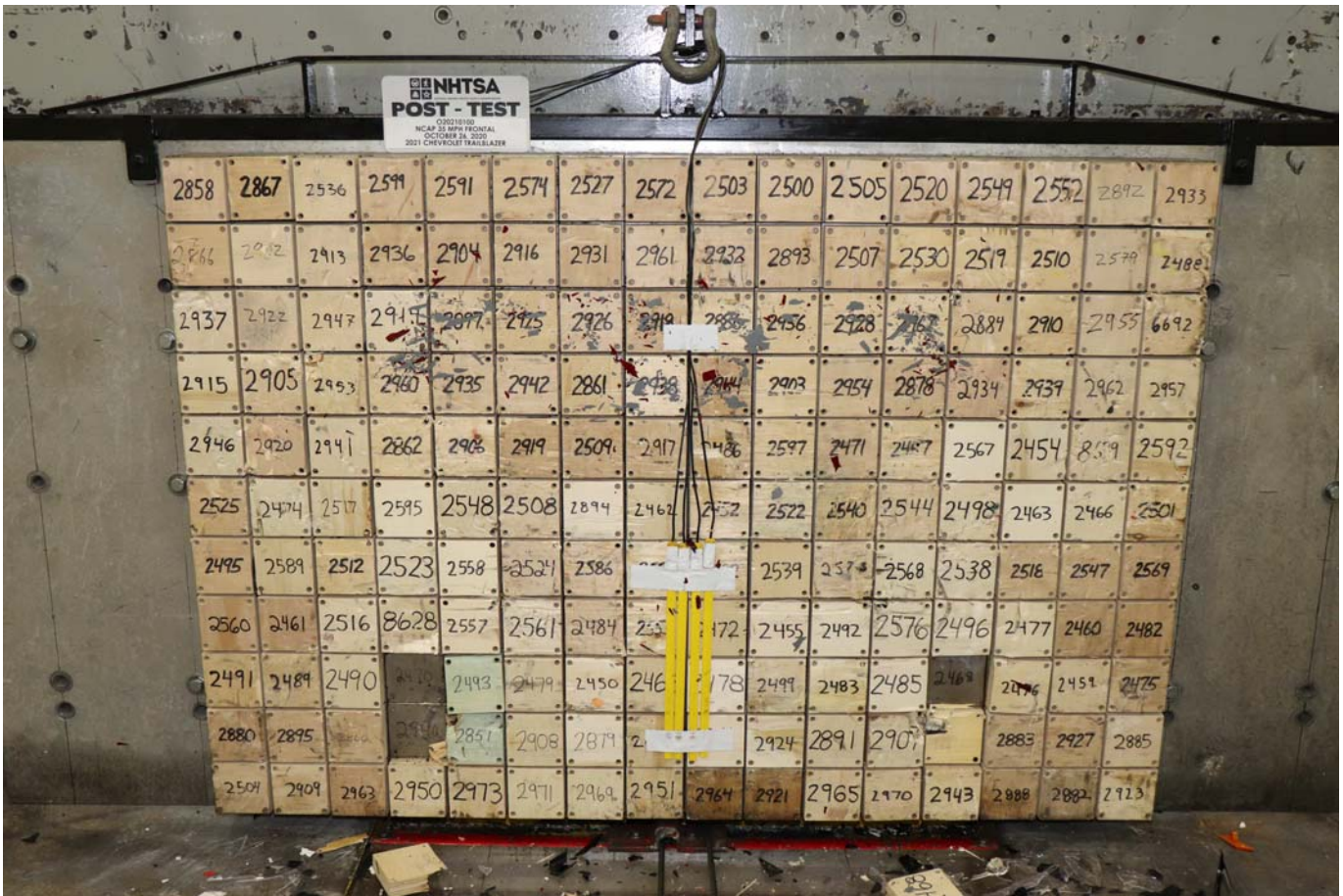
Photo No. 003 - Post-Test Load Cell Wall
