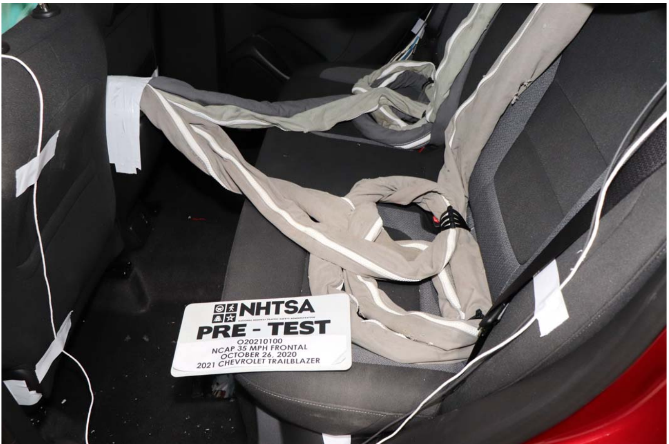
Photo No. 028 - Pre-Test Dummy Cable Routing
