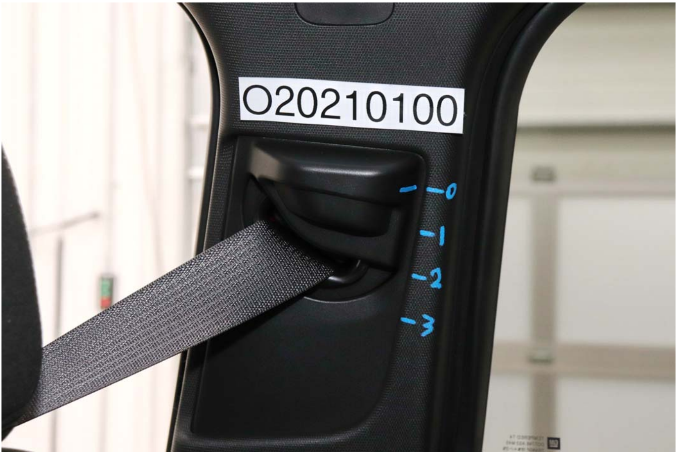
Photo No. 061 - Pre-Test View of Belt Anchorage for Passenger Dummy
