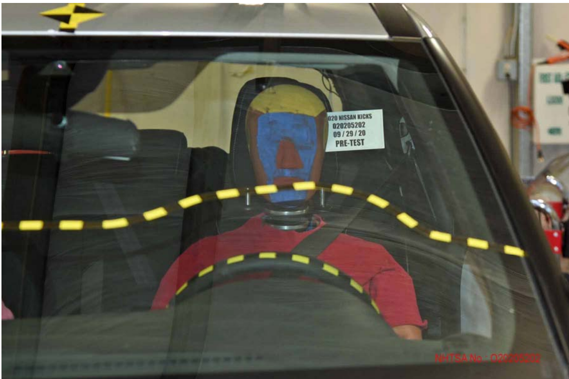
FIGURE 30. Pre-Test Driver Dummy Front View
