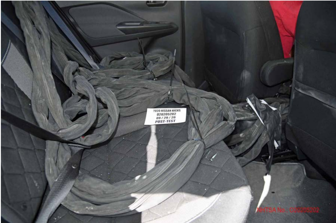
FIGURE 29. Post-Test Dummy Cable Routing
