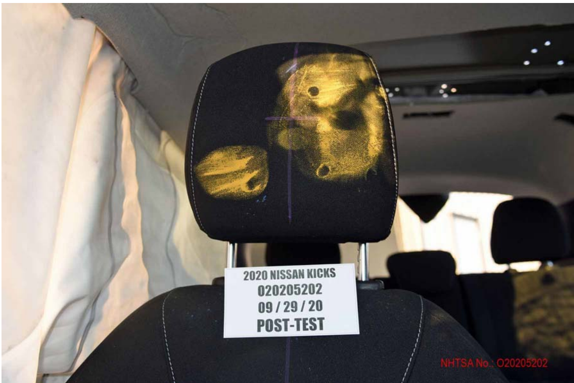
FIGURE 73. Post-Test Passenger Dummy Contact with Headrest
