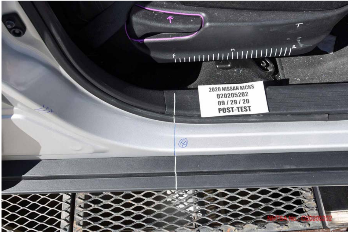
FIGURE 60. Post-Test Passenger's Seat Fore-Aft Markings
