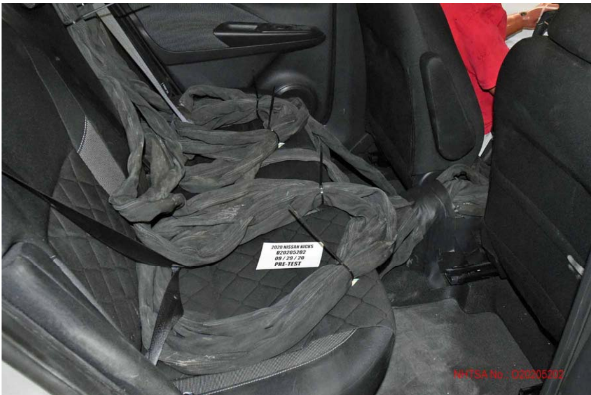
FIGURE 28. Pre-Test Dummy Cable Routing
