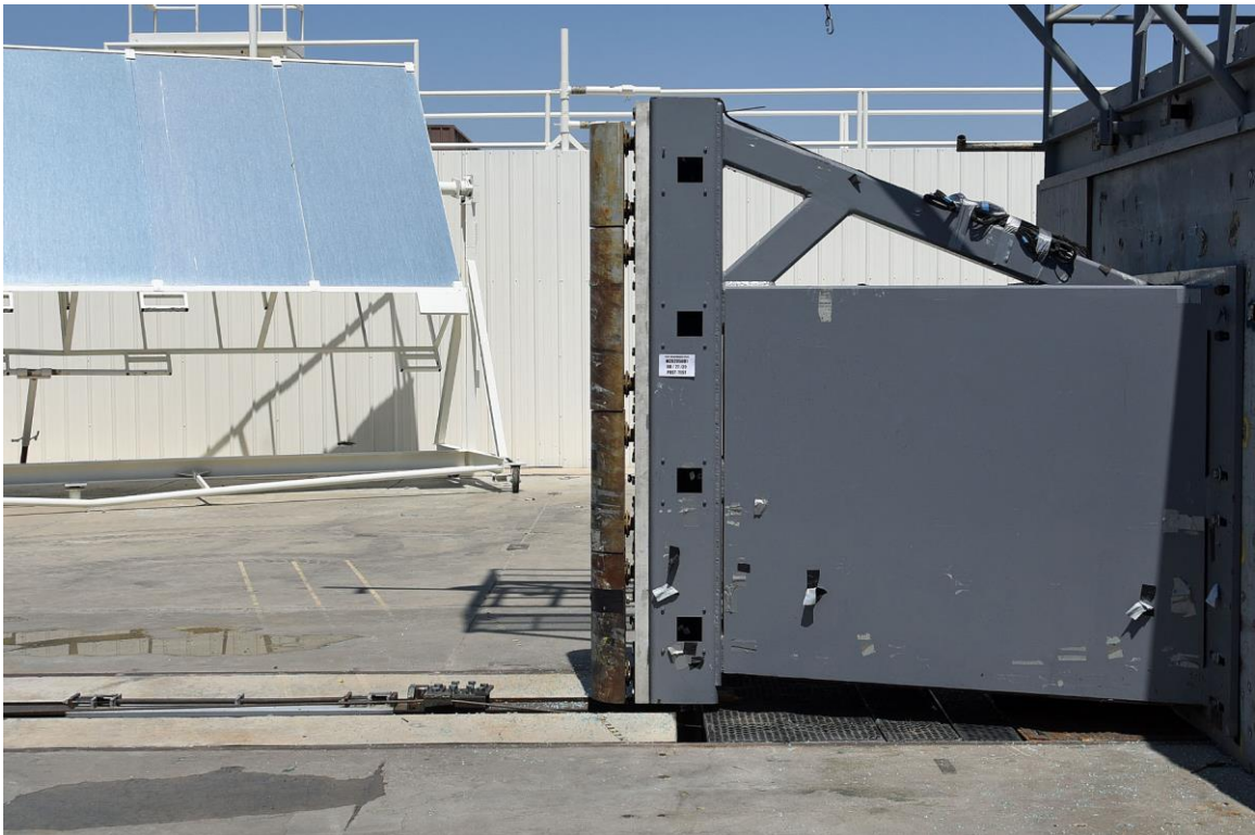
FIGURE 60. Post-Test Pole Barrier Side View
