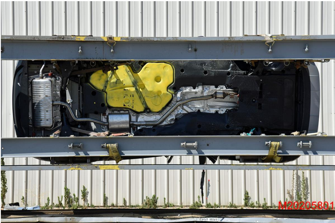
FIGURE 66. FMVSS No. 301 Static Rollover 270 Degrees
