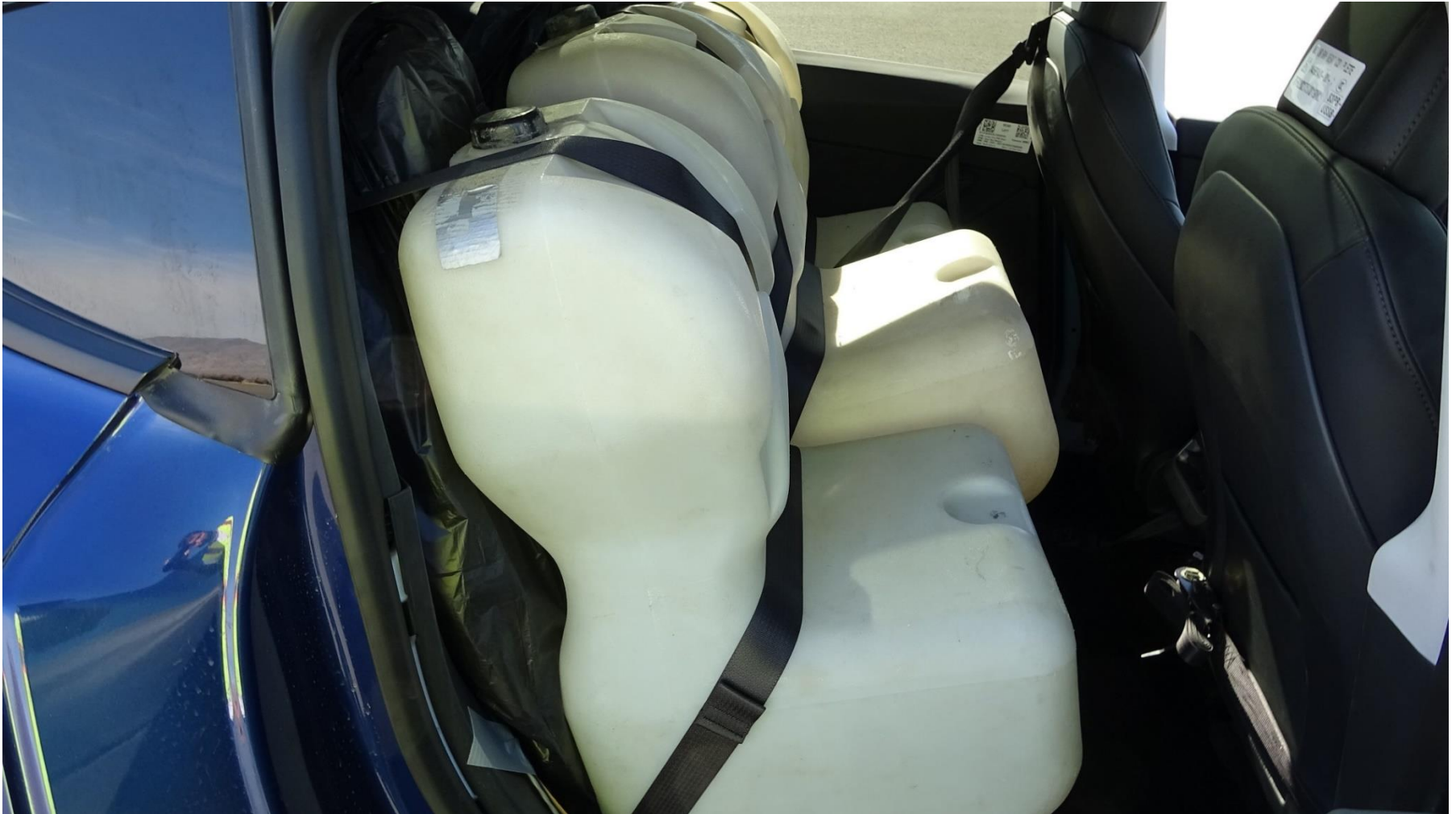
Figure A10. Ballast Condition
