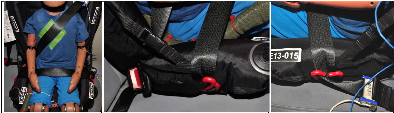
FIGURE 5 PRE-TEST POSITION OF HYBRID III 6 - YEAR-OLD PLACED ON THE GOBOOSTER® IN THE FORD FIESTA
