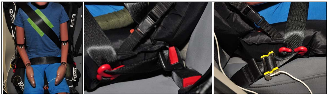
FIGURE 6 PRE-TEST POSITION OF HYBRID III 10 - YEAR-OLD PLACED ON THE GOBOOSTER® IN THE FORD FIESTA
