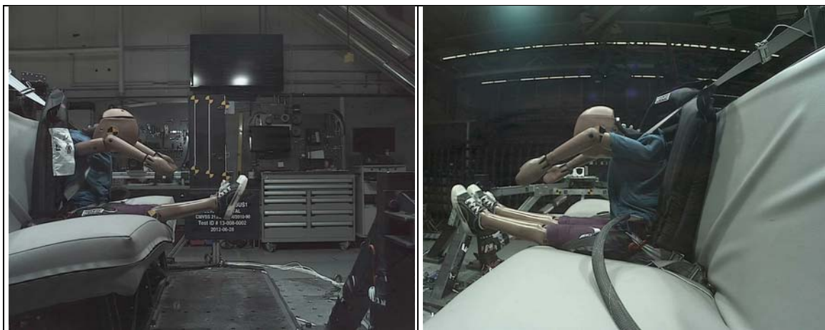
FIGURE 13 MOTION OF HYBRID III 6-YEAR-OLD AND THE GOBOOSTER DURING THE CMVSS 213 COMPLIANCE TEST.
