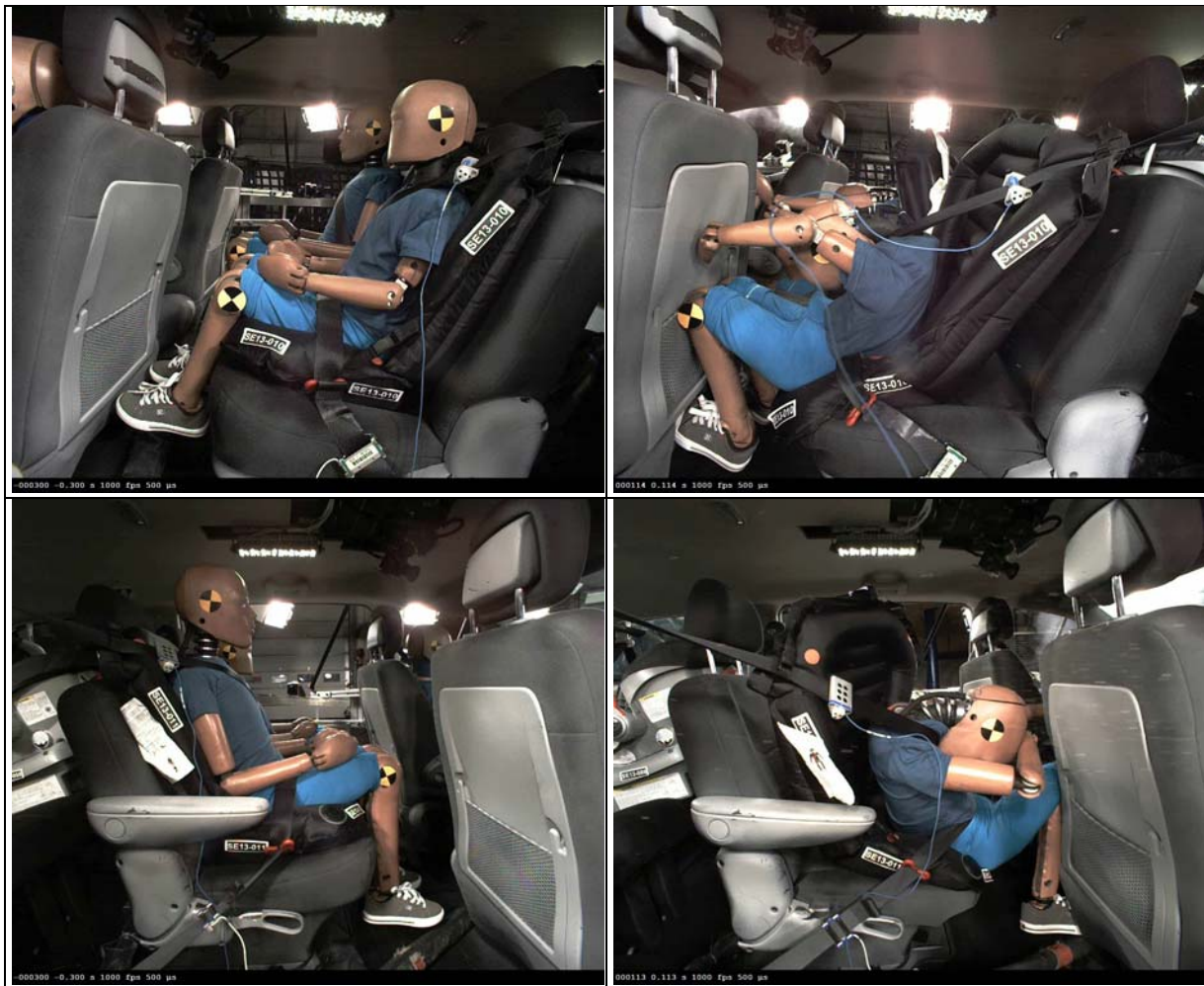
FIGURE 9 FREEZE FRAME IMAGES OF 6-YEAR-OLD PRIOR TO IMPACT (TOP LEFT) AND AT MAXIMUM EXCURSION (TOP RIGHT); 10-YEAR-OLD PRIOR TO IMPACT (BOTTOM LEFT) AND AT MAXIMUM EXCURSION (BOTTOM RIGHT) DURING FFRB TEST AT 40 KM/H.
