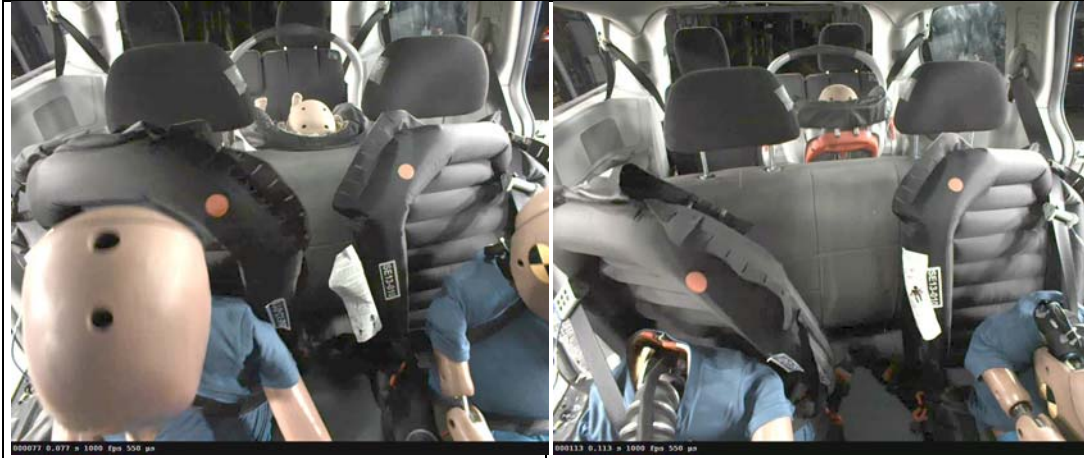
FIGURE 10 FRONTAL VIEWS OBTAINED DURING FORWARD EXCURSION SHOWING SHOULDER BELT LOADING OF THE NECK AND INBOARD AXILLAE FOR BOTH THE 6 AND 10-YEAR-OLD ATDS.
