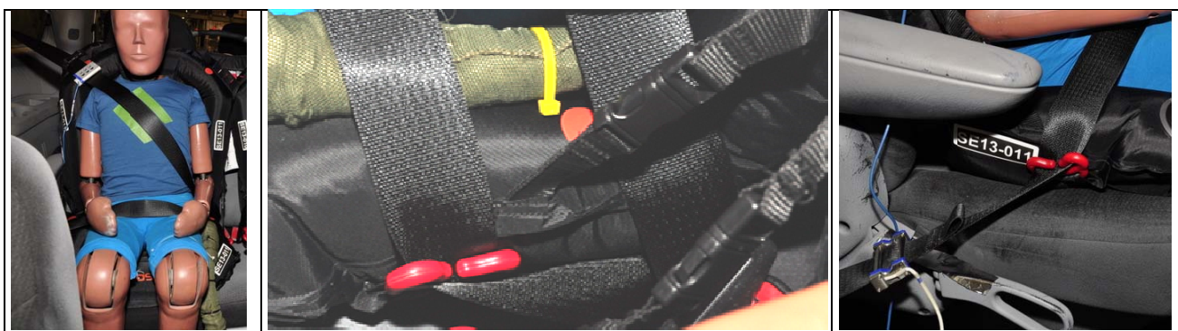
FIGURE 3 PRE-TEST POSITION OF HYBRID III 10 - YEAR-OLD PLACED ON THE GOBOOSTER® IN DODGE GRAND CARAVAN
