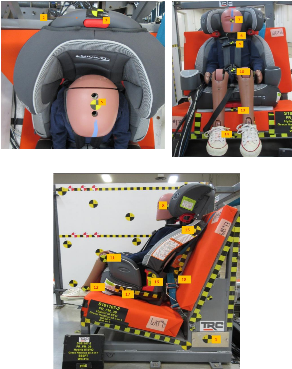
Figure 8 – FARO measurement locations for forward-facing CRS
