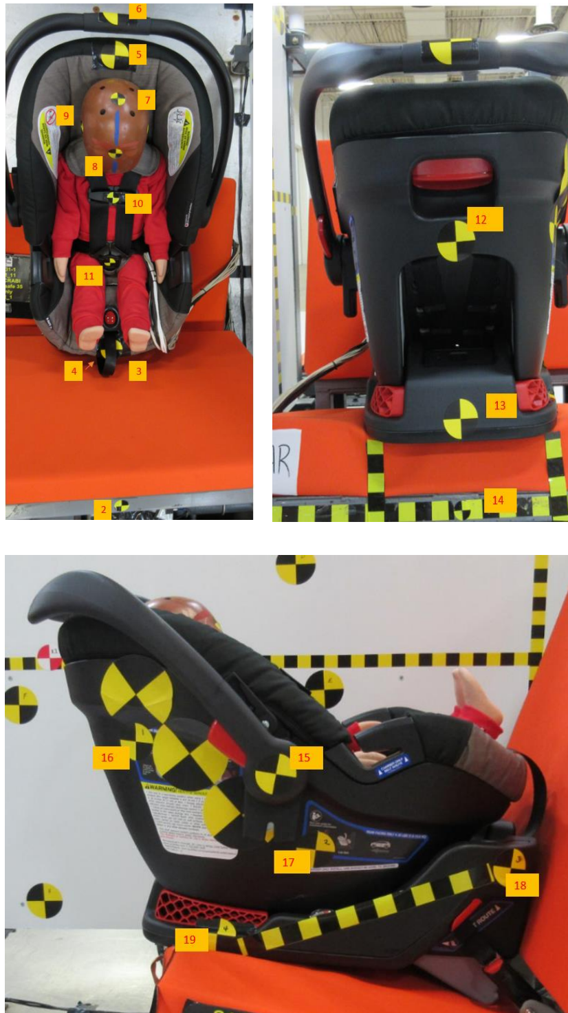
Figure 9 – FARO arm measurement locations for rear-facing CRS.
