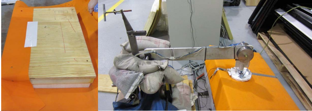
Figure 15: Foam and Plywood Wrapped in ECE R44 Material
