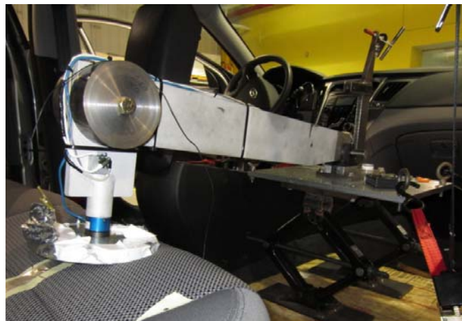
Step 3: Measure the angle of the pendulum arm when it makes first contact with the seat
