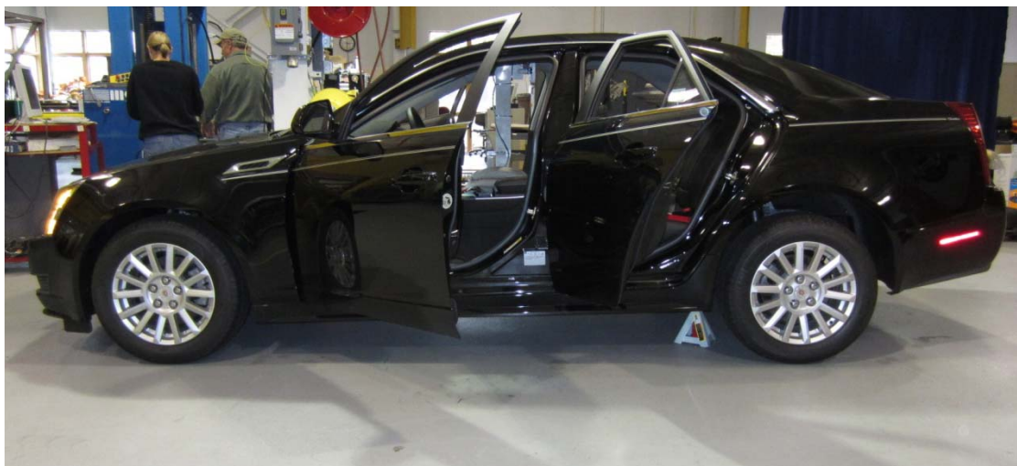
Step 1: Place jack stands under the rear of the vehicle to isolate shock absorbers
