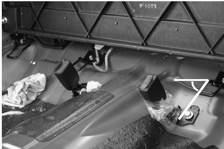
Photo No. 8: Lower Anchor Angle
