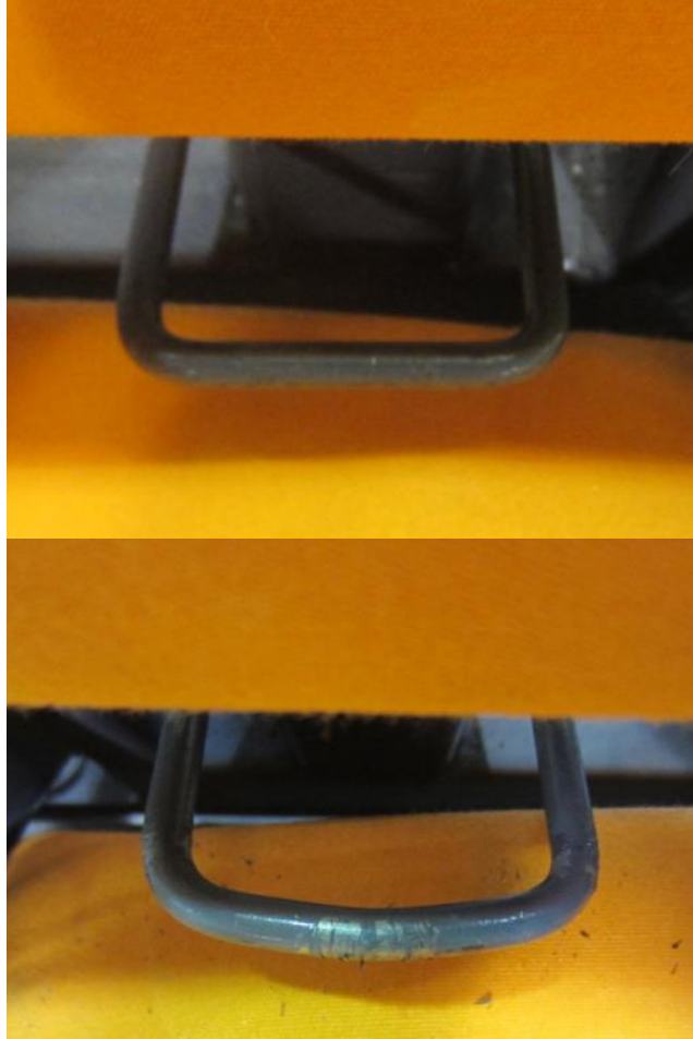
Figure 7: Original Anchorage Shape (above), Deformed Anchorage (below)
