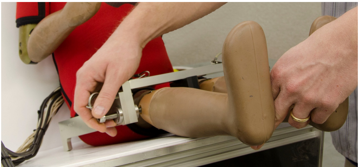
Figure 88. Pull feet apart while tightening bolt on positioning tool
