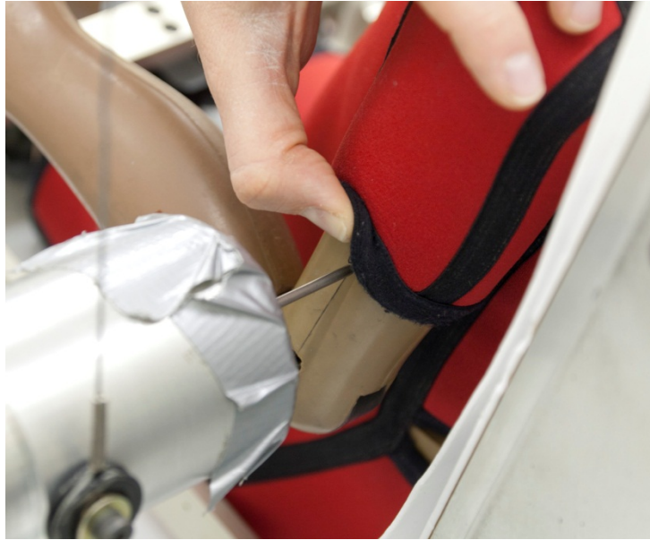
Figure 97. Setting arm to contact position
