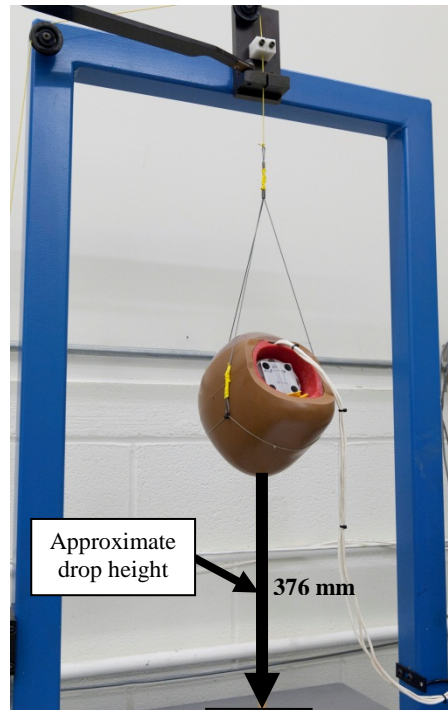
Figure 7. Initial suspension of the head using approximate drop height
