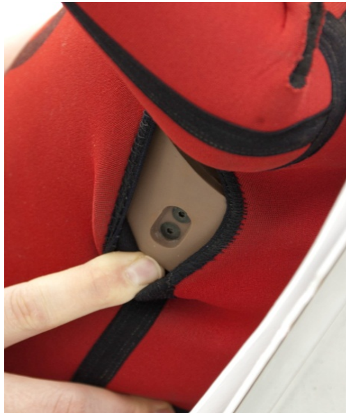
Figure 91. Positioning probe to impact point on thorax
