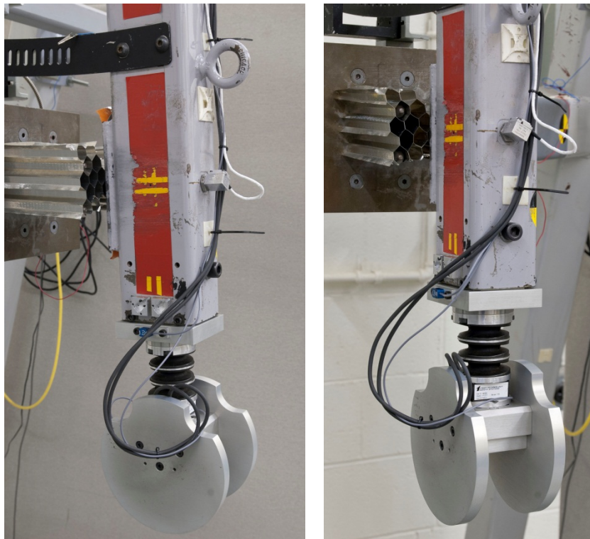
Figure 44. Install hexcell to pendulum
