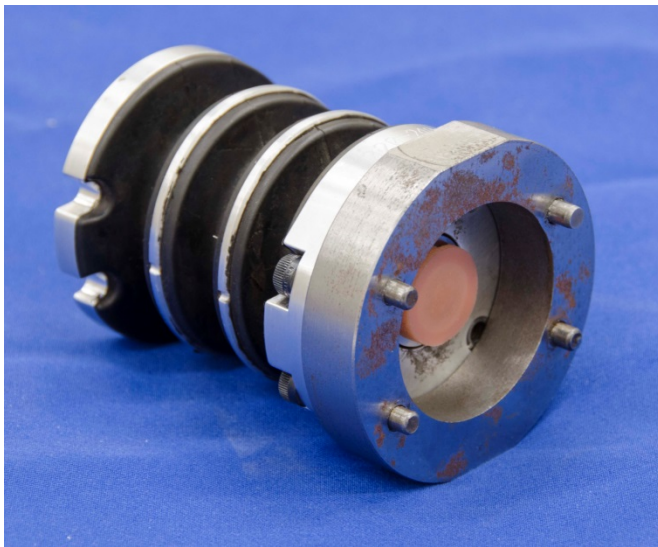
Figure 45. Assemble neck adapter plate assembly to lower neck
