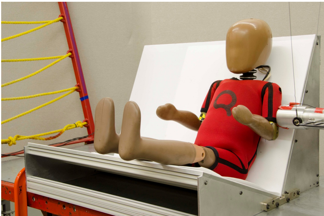
Figure 99. Final setup for Q3s thorax with arm qualification test
