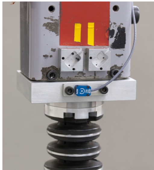
Figure 32. Install ARS to pendulum
