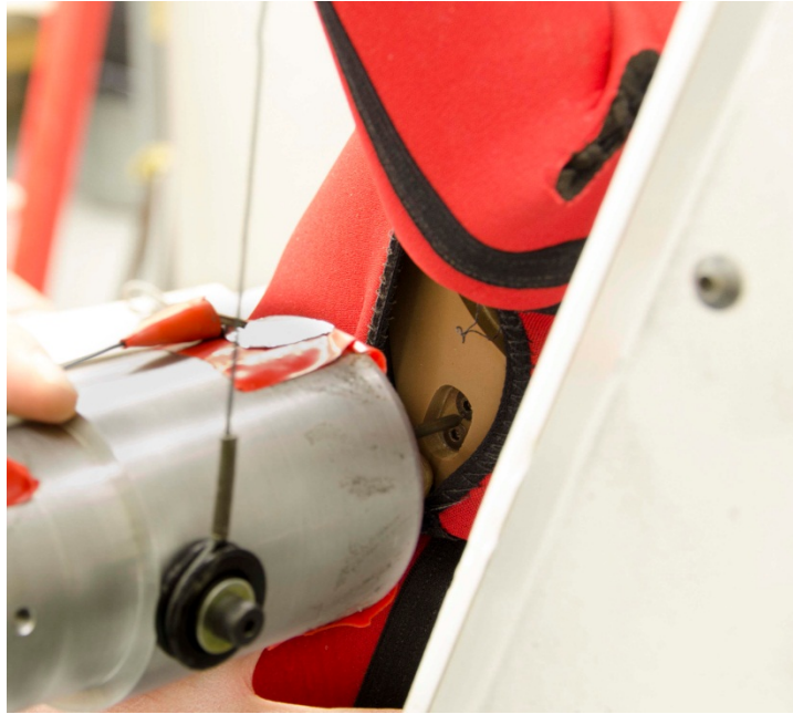
Figure 93. Align pointer between IRTRACC bolts
