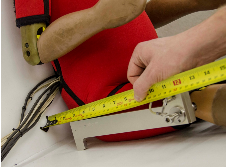
Figure 112. Squaring the dummy to the seat using the Q3s positioning tool
