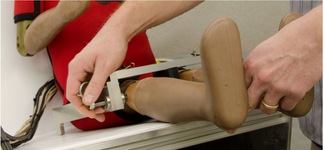
Figure 128. Pull feet apart while tightening bolt on positioning tool
