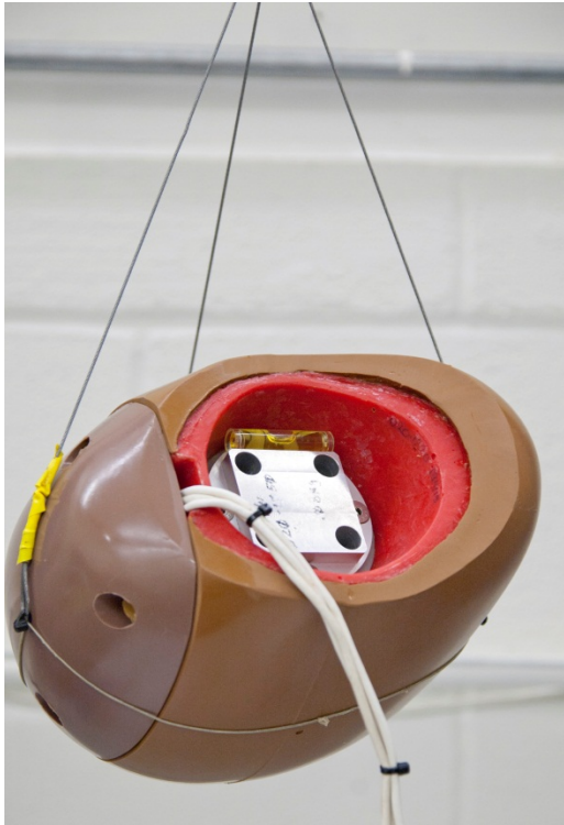
Figure 10. Harness routing for lateral head drop impact
