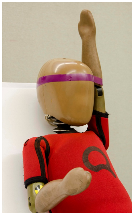
Figure 127. Tape the impact side arm to the head for pelvis tests
