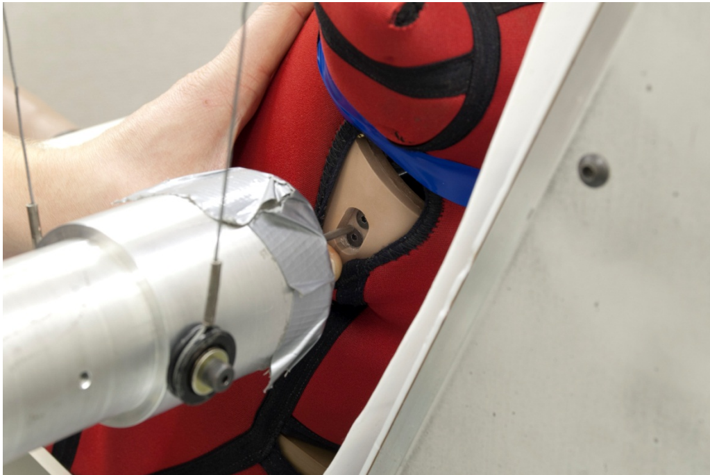
Figure 114. Align pointer between IRTRACC bolts
