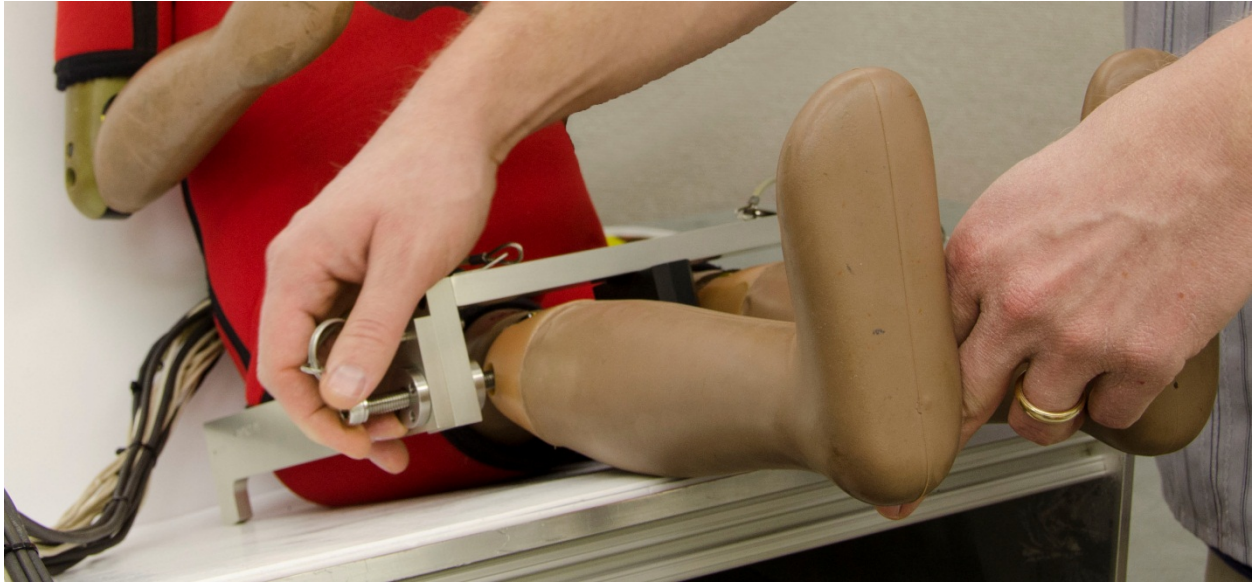
Figure 110. Pull feet apart while tightening bolt on positioning tool
