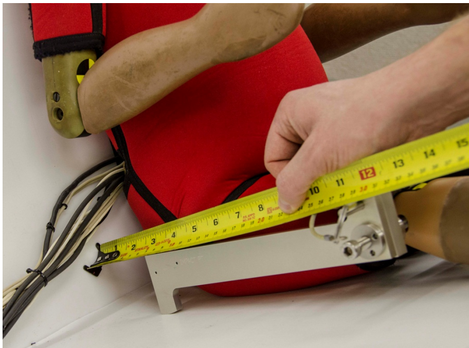
Figure 90. Squaring the dummy to the seat using the Q3s positioning tool
