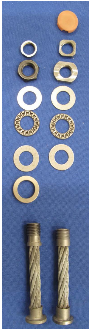
Fig. B1. NPRM cable design (left); Final Rule cable design (right). Note that the revised design eliminates one washer and uses thinner nuts to achieve a lower total stack height
