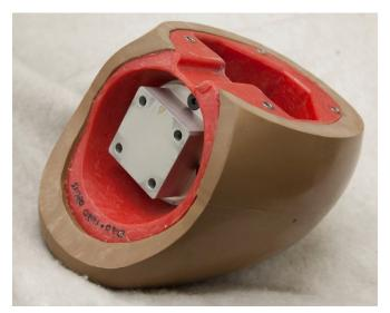
Figure 15. Head removed from neck
