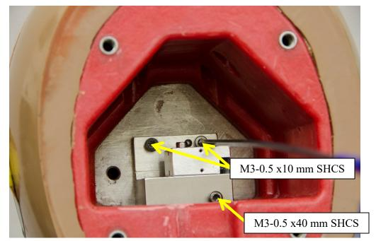
Figure 11. Remove angular rate sensor bracket assembly
