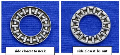
Figure 31. Details of neck thrust bearing
