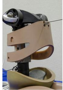
Figure 130. Secure the ribcage assembly at the sternum prior to mounting IR-TRACC
