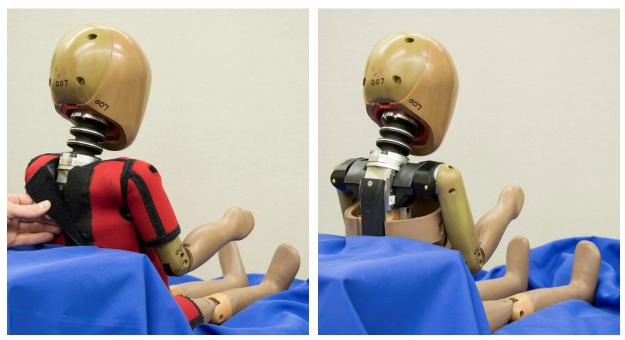
Figure 3. Remove suit to begin disassembly
