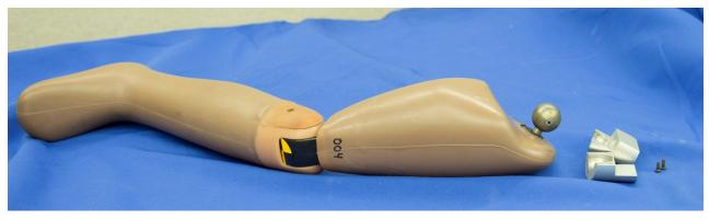
Figure 46. Hip joint assembly removed from leg
