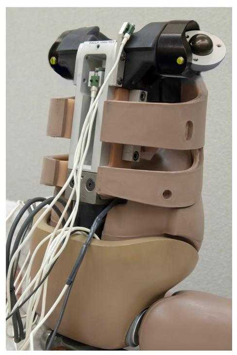
2. Route the wiring for the T1 and upper pine accelerometers along the posterior thoracic spine (Figure 160).
