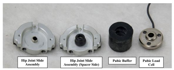
Figure 141. Parts needed for pubic load cell assembly
