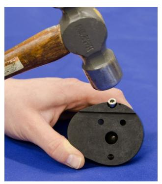
Figure 58. Using a hammer to remove shoulder ball
