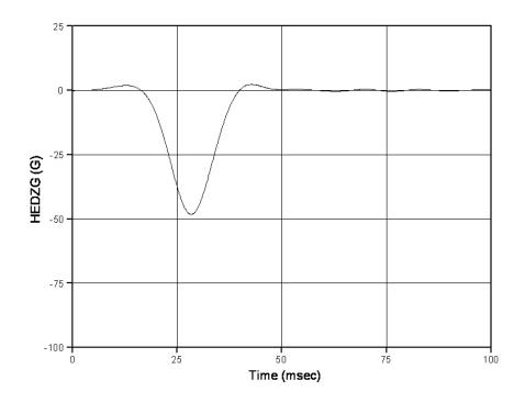
Figure C- 3. Polarity of Z axis accelerometer data channel
