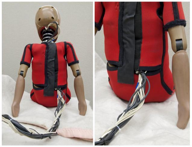
Figure 166. Wiring bundles after installation of suit
