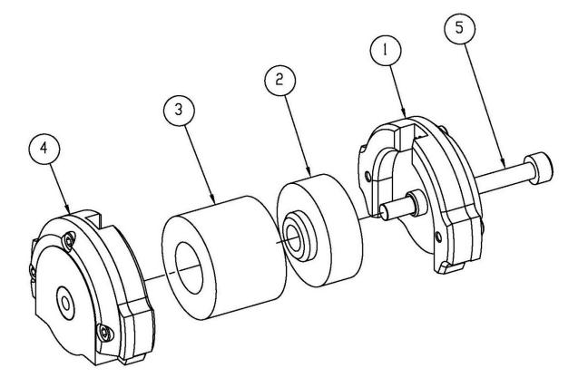
Figure 80. Pubic load cell assembly – exploded view
