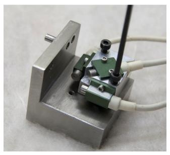
Figure 106. Secure accelerometer mounting block to instrumentation bracket
