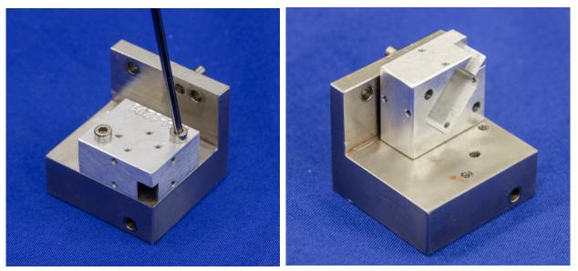
Figure 13. Remove the accelerometer/ARS mounting block from the instrumentation bracket
