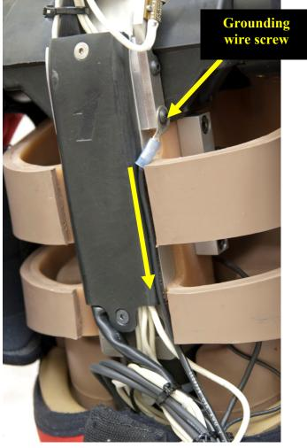
Figure 157. Installing grounding wire
