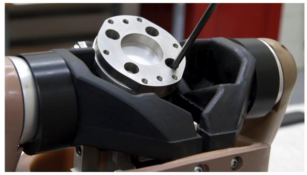
Figure 117. Install lower neck load cell to torso
