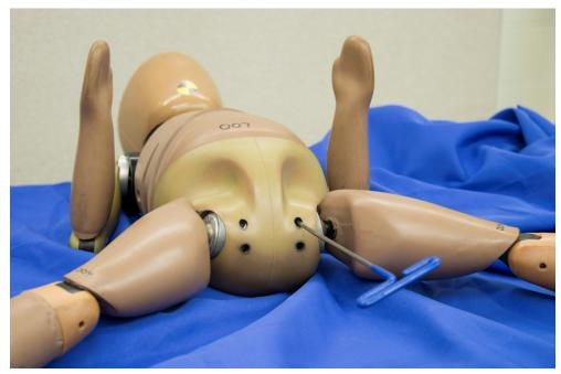
Figure 43. Remove SHCS from pelvis
