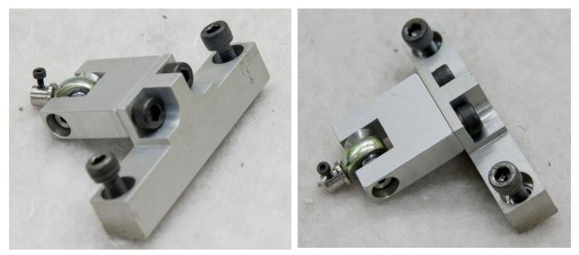
Figure 64. IR-TRACC bracket 1 removed from thorax
