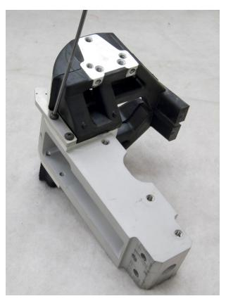
Figure 70. Remove accelerometer adaptor assembly from thoracic spine
