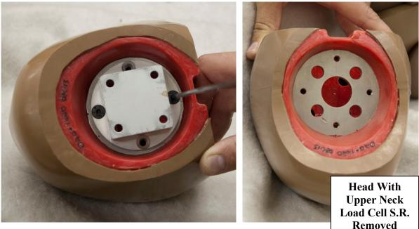
Figure 16. Remove upper neck load cell structural replacement
