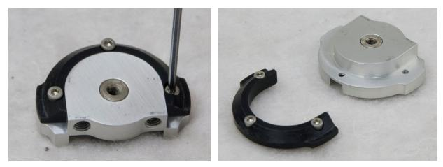
Figure 99. Remove hip joint slide spacer from hip joint slide assembly
