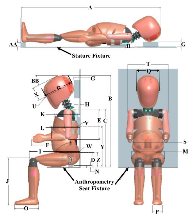
Figure 167. External dimensions of the Q3s dummy
