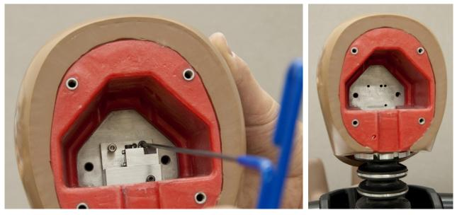
Figure 8. Uninstall instrumentation bracket from the head
