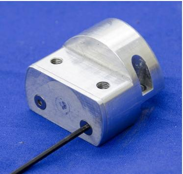
Figure 86. Remove spring retainer plate
