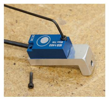
Figure 137. Install tilt sensor to bracket
