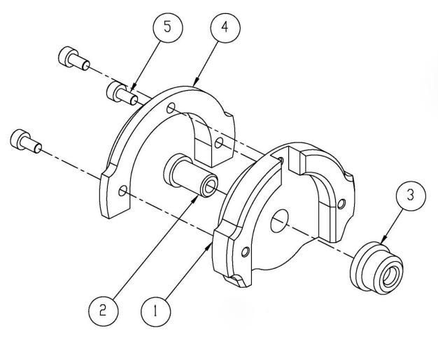
Figure 82. Hip joint slide assembly (spacer side) components
