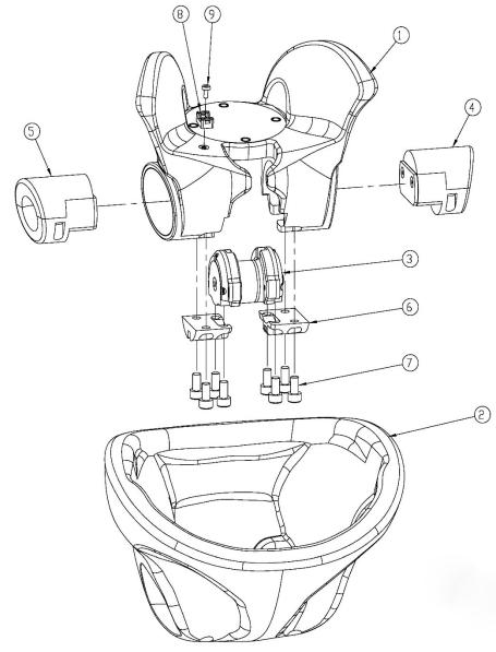
Figure 78. Pelvis assembly – exploded view
