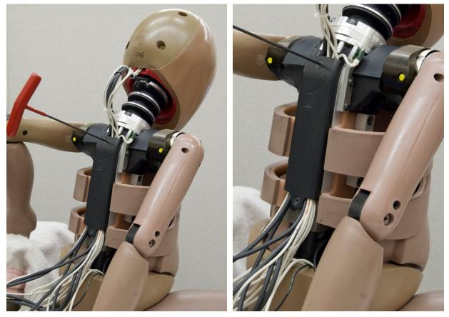
Figure 164. Installing cable guide to thoracic spine
