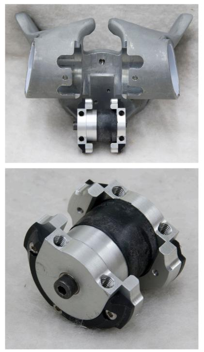
Figure 97. Pubic load cell assembly after removal from machined pelvis
