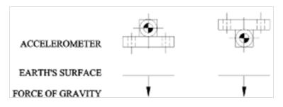
Figure C- 4. Accelerometer perpendicular to gravity in two orientations 180° apart
