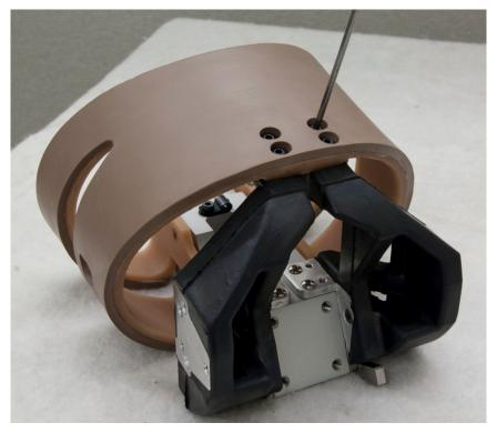
Figure 68. Remove molded shoulder assembly from ribcage assembly
