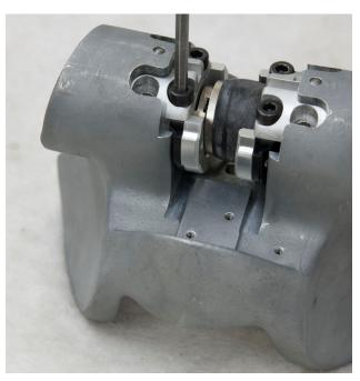
Figure 148. Install non-struck side hip joint cover
