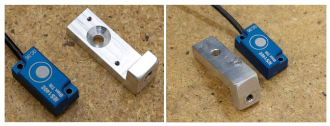
Figure 136. Tilt sensor and bracket for Q3s
