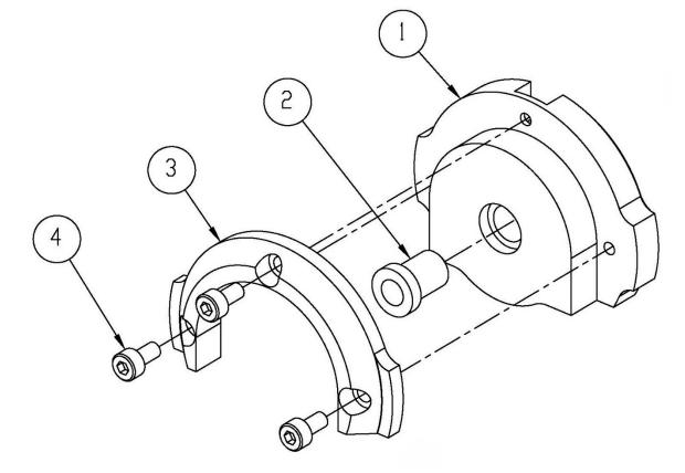
Figure 81. Hip joint slide assembly – exploded view
