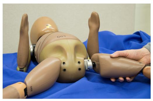
Figure 44. Separate leg from pelvis
