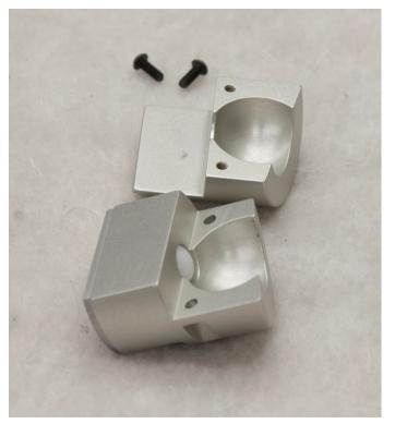
Figure 85. Hip joint after separating from leg
