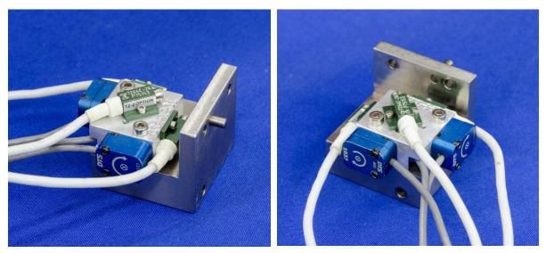
Figure 111. Accelerometer/ARS mount installed to bracket
