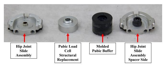
Figure 98. Pubic load cell assembly
