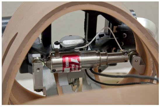
Figure 135. IR-TRACC installed in Q3s thorax
