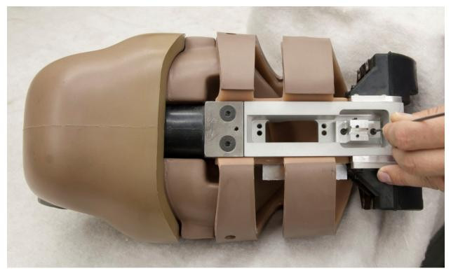
Figure 60. Remove upper spine accelerometer mounting bracket
