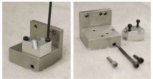
Figure 10. Removing accelerometer block from instrumentation bracket assembly
