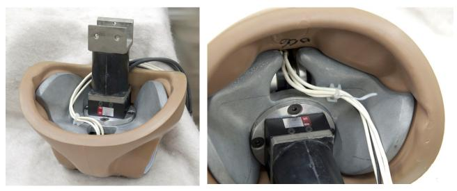
Figure 163. Pelvic wiring with pelvis skin installed
