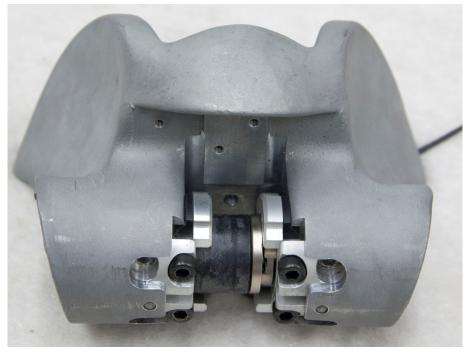
Figure 150. Pubic load cell installed in Q3s pelvis
