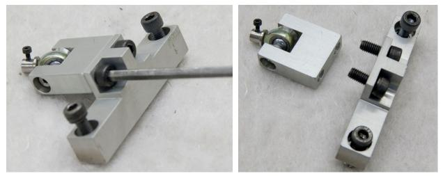
Figure 65. Disassemble IR-TRACC bracket 2 from IR-TRACC bracket 1
