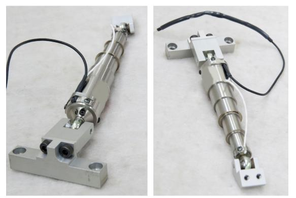
Figure 129. IR-TRACC assembly configured for installation in thorax
