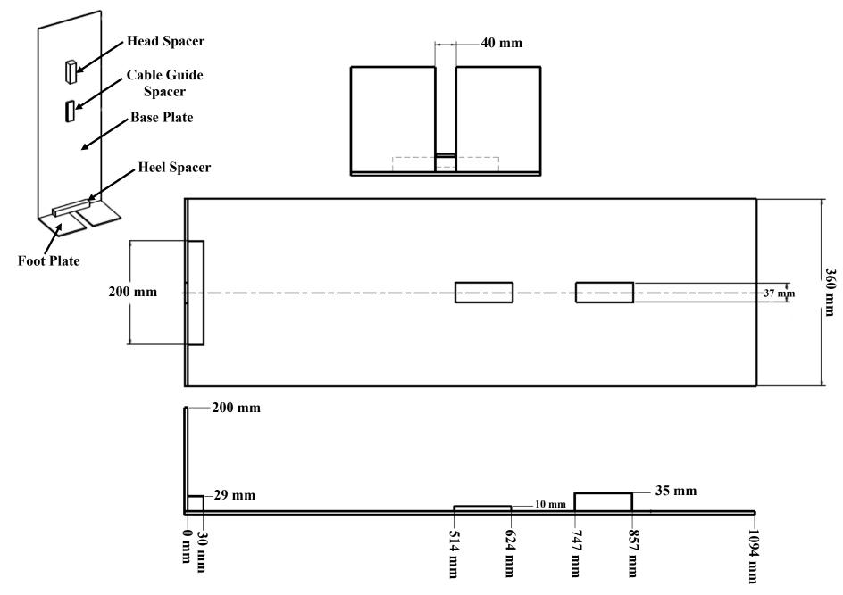
Figure 168. Stature measurement fixture details
