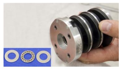
Figure 30. Remove thrust bearing washers and thrust bearing
