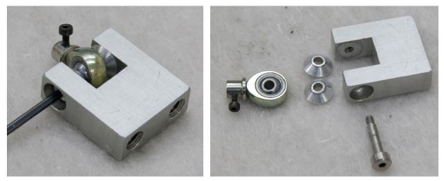
Figure 66. Remove the rod end mount from IR-TRACC bracket 2
