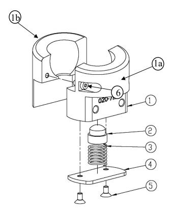
Figure 79. Hip joint assembly – exploded view
