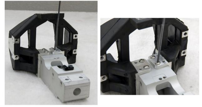
Figure 72. Remove the molded shoulder assembly from the thoracic spine
