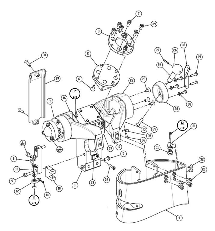
Figure 49. Upper torso assembly – exploded view
