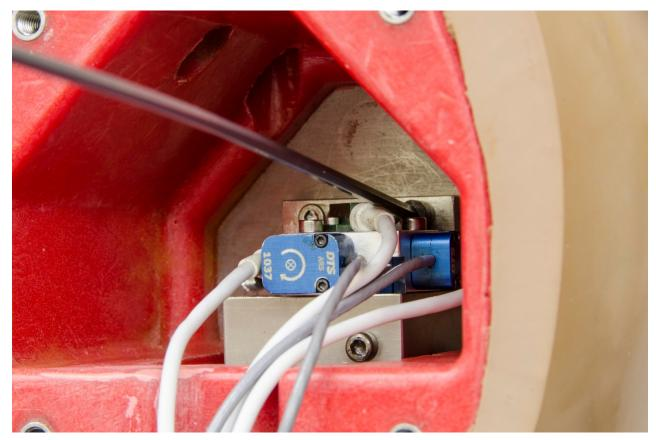
Figure 113. Install instrumentation bracket into head
