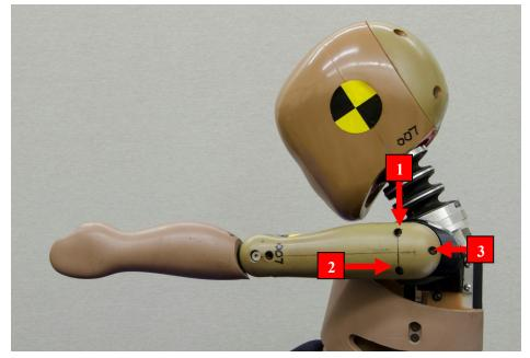
Figure B- 1. Setting shoulder torque
