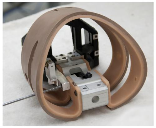
Figure 63. Remove IR-TRACC bracket 1 from thorax
