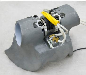
Figure 161. Pelvis accelerometer cable routing
