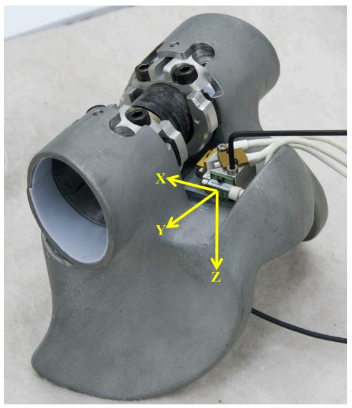
Figure 152. Install pelvis accelerometer block into machined pelvis
