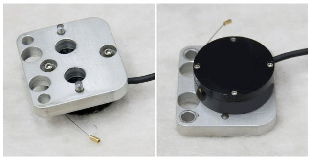
Figure 119. Install string potentiometer to mounting bracket
