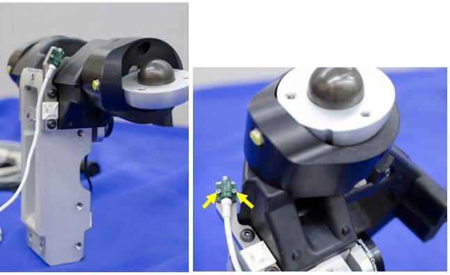
Figure 128. T1 accelerometer installed
