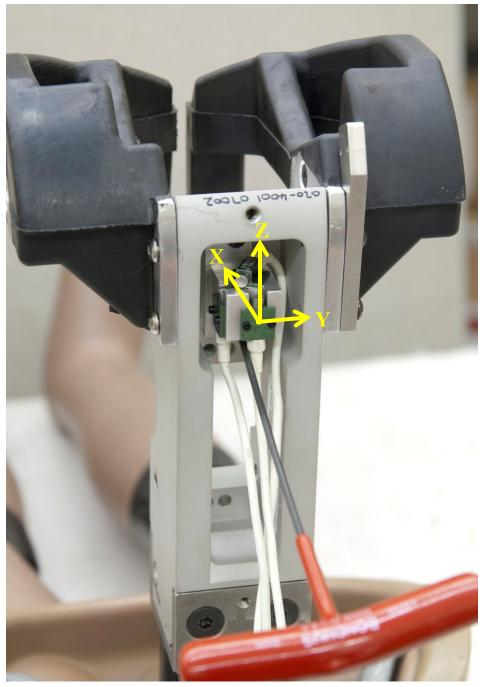
Figure 126. Install upper spine accelerometers into thoracic spine
