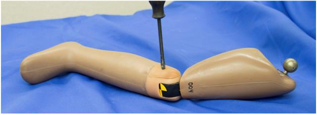
Figure 47. Remove stop screw at knee
