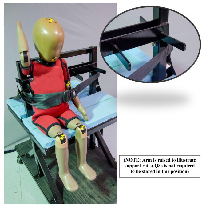
Figure G- 3. Q3s storage chair showing details of thorax support rails
