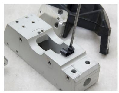
19. Remove the nylon loop clamp cable holder which secures the IR-TRACC and shoulder stringpot instrumentation cables by taking out the M4-0.7 x 16mm SHCS (Figure 74).
