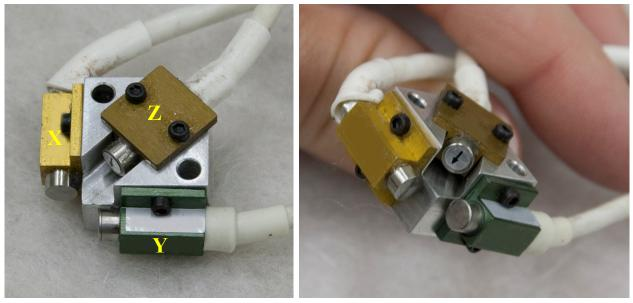
Figure 151. Install pelvis accelerometers to block
