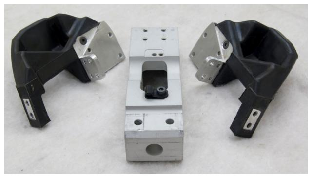
Figure 73. Left and right molded shoulder assemblies separated from thoracic spine
