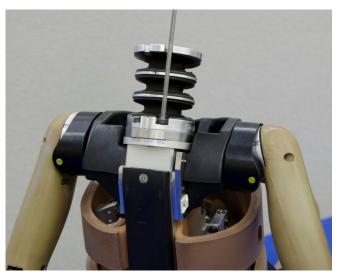
Figure 20. Remove screws from rear base of neck
