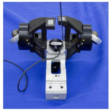
Figure 122. Secure stringpot assembly to thoracic spine
