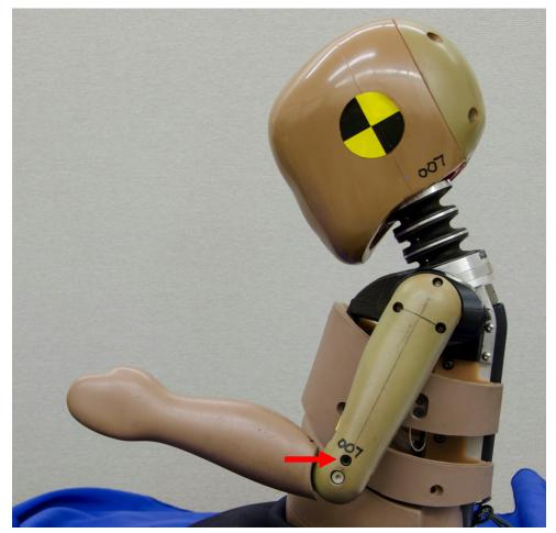
Figure B- 2. Setting elbow torque
