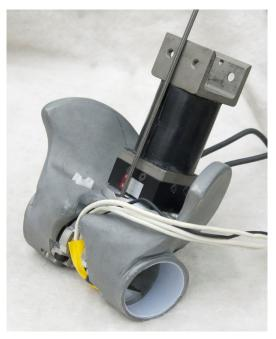
Figure 155. Install lumbar load cell to machined pelvis
