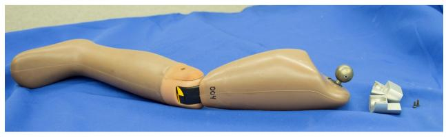
Figure 84. Hip joint assembly removed from leg
