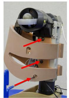
Figure 132. Install 3 BHCS to thoracic spine on impact side
