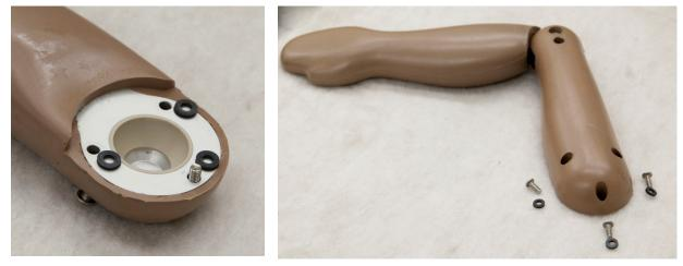
Figure 37. Arm removed from Q3s showing Viton® washers at shoulder
