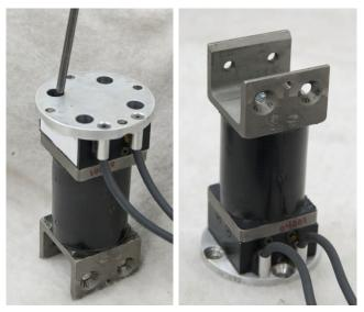
Figure 154. Install lumbar load cell to the bottom
