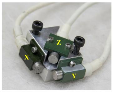
Figure 105. Install accelerometers to triaxial block
