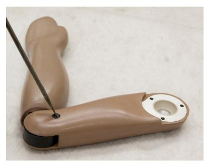
Figure 38. Remove stop screw at elbow
