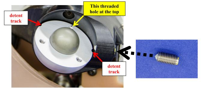
Figure 75. Aligning the shoulder ball retaining ring for proper installation of the shoulder
