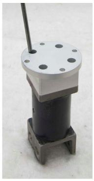
Figure 92. Remove lumbar load cell structural replacement
