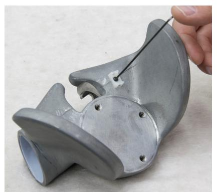
Figure 100. Remove #4 cable tie mount from machined pelvis
