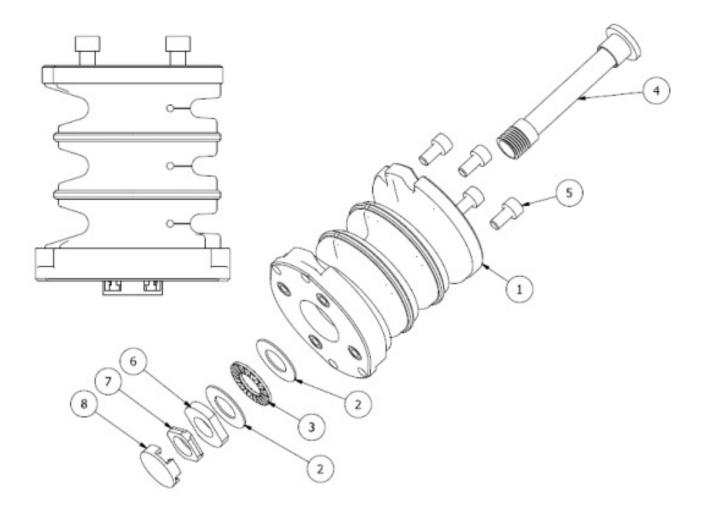
Figure 17. Neck assembly – exploded view
