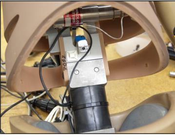
Figure 140. Tilt sensor installed into Q3s thorax
