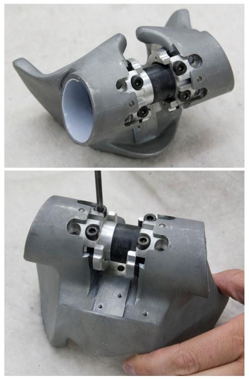
Figure 94. Begin disassembly of pubic load cell assembly from machined
