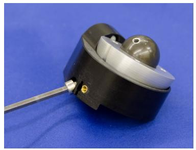
Figure 57. Remove shoulder ball from shoulder cup
