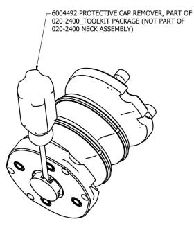
Figure 18. Protective cap remover from neck assembly toolkit
