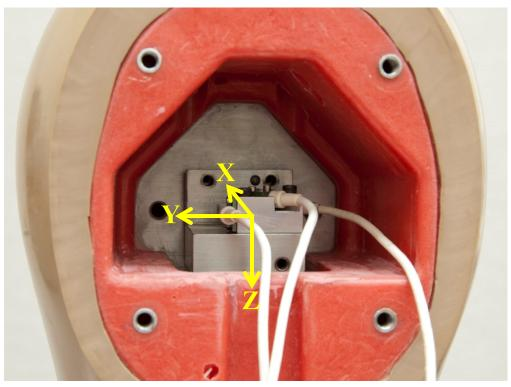
Figure 109. Head accelerometers installed in head
