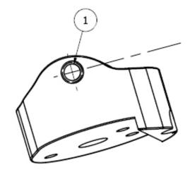
Figure 52. Q3s shoulder cup showing location of ball plunger
