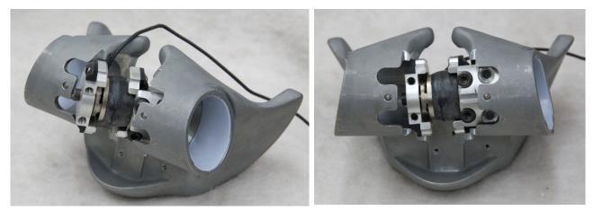
Figure 147. Insert compressed pubic assembly into machined pelvis
