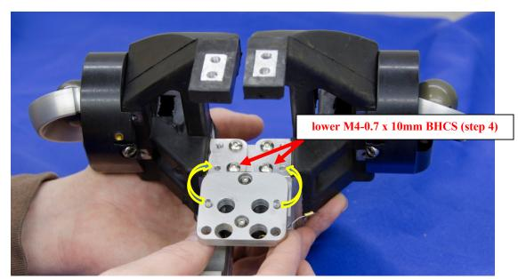
Figure 120. Install shoulder stringpot bracket alignment pins into locator holes
