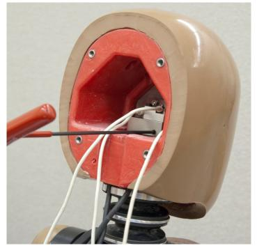
Figure 108. Installing M3-0.5 x 40mm SHCS to lower portion of instrumentation bracket 76
