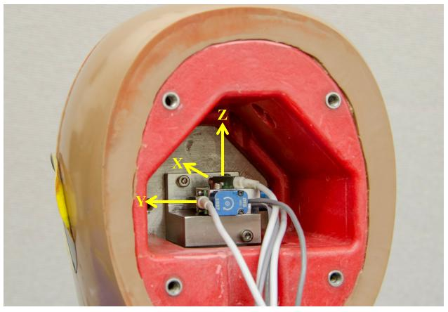
Figure 114. ARS assembly installed in head
