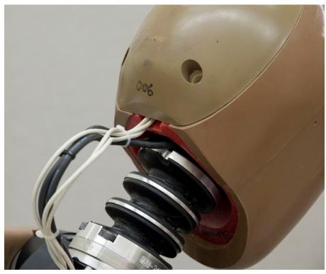
Figure 158. Cable routing for head and neck
