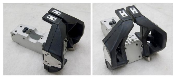
Figure 69. Molded shoulder assembly separated from ribcage assembly
