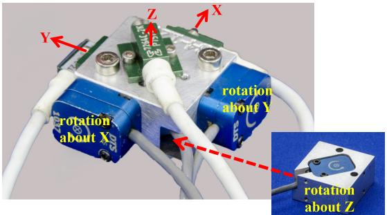
Figure 110. Mount ARS transducers and accelerometers to accel/ARS mount
