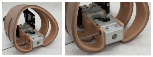
Figure 67. Remove screws which attach ribcage assembly to thoracic spine
