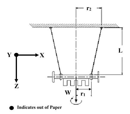
Figure D-1. Assembly for determining probe moment of inertia
