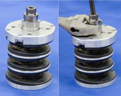
Figure 25. Uninstall cable lock nut
