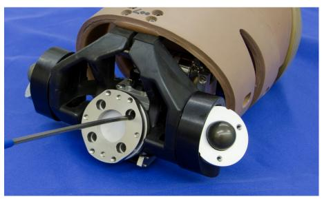
Figure 53. Remove neck/torso interface plate
