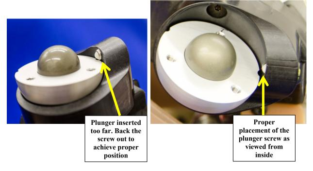
Figure 76. Screwing the spring-loaded screw into the shoulder detent
