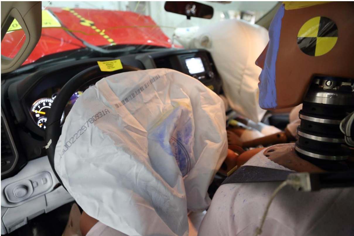
049 Post-Test Driver Dummy Contact with Airbag
