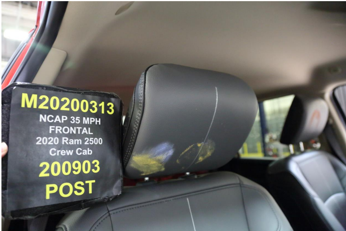
073 Post-Test Passenger Dummy Contact with Headrest
