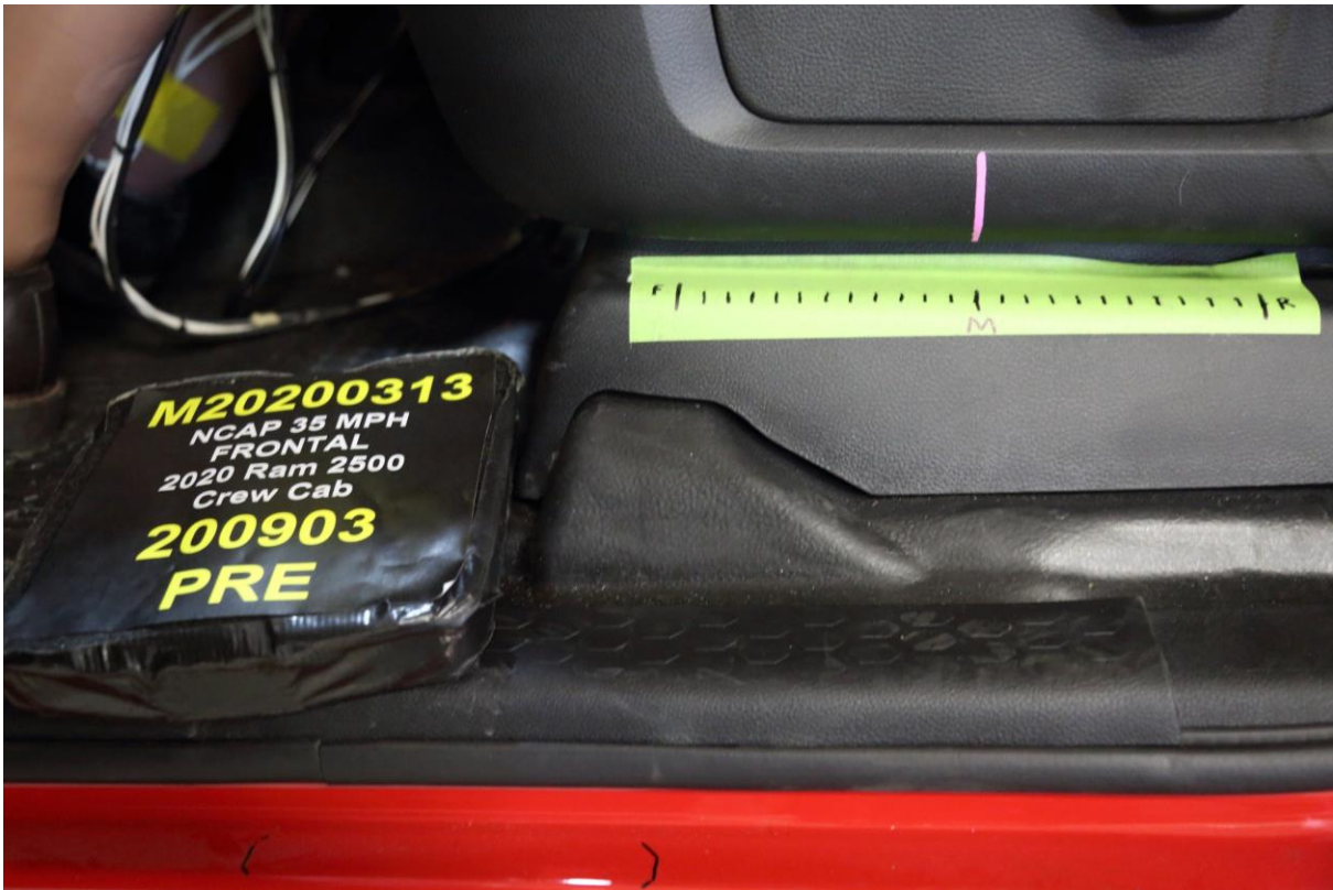
036 Pre-Test Driver's Seat Fore-Aft Markings
