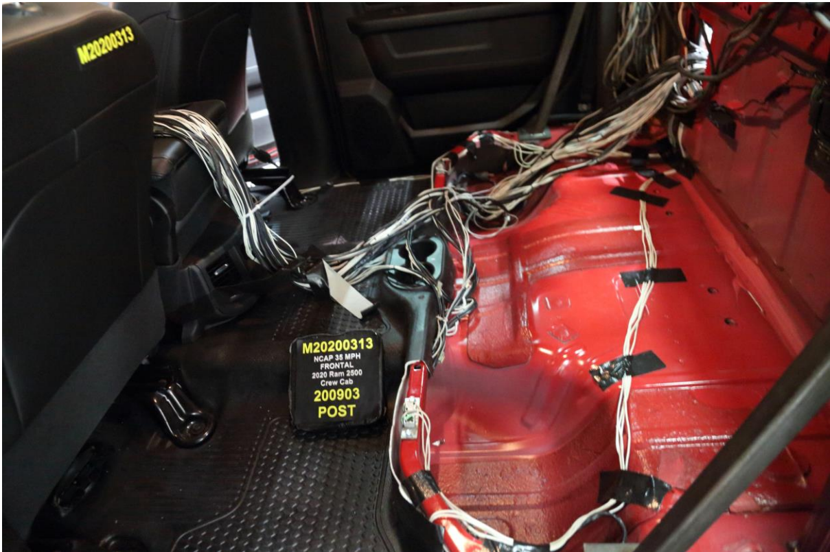
029 Post-Test Dummy Cable Routing
