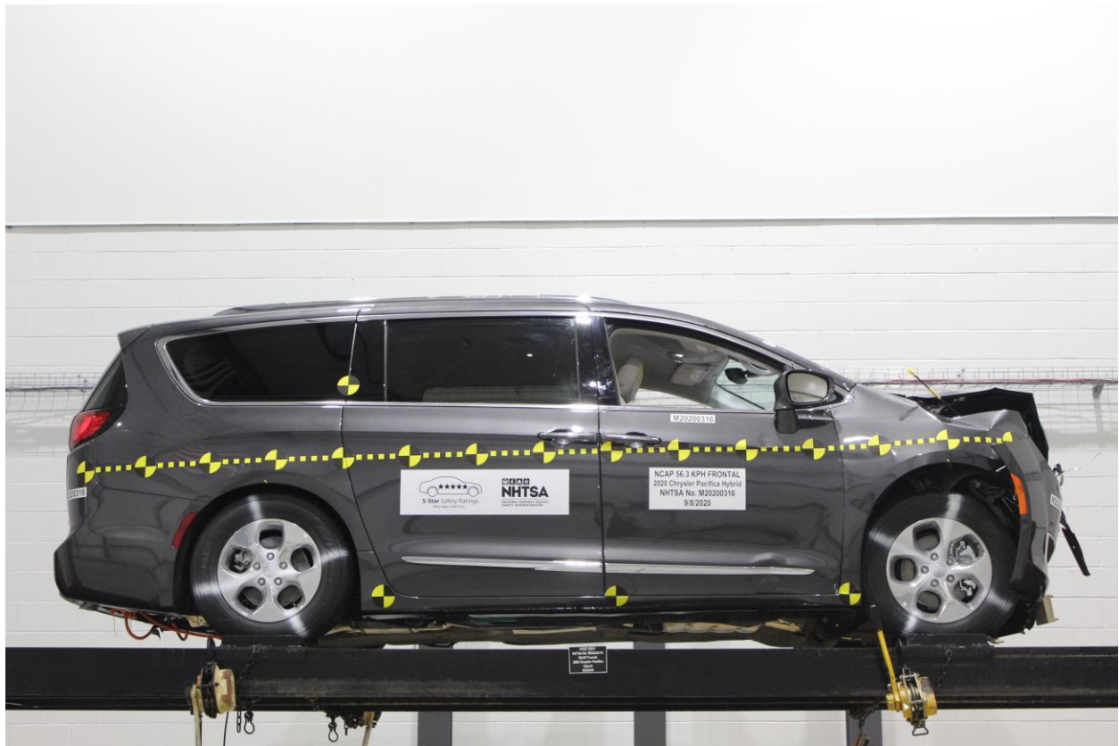
Figure A-77: Vehicle at 0° on Static Rollover Device
