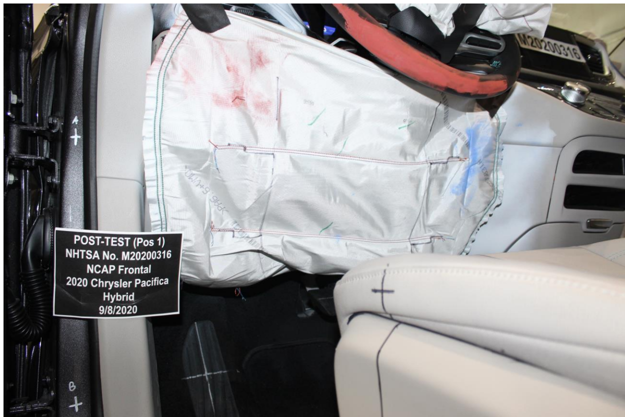
Figure A-45: Post-Test Driver's Side Knee Bolster
