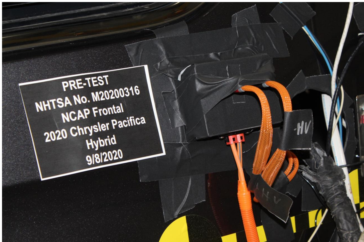
Figure 305-24: Pre-Impact View of Installed Test Interface Port
