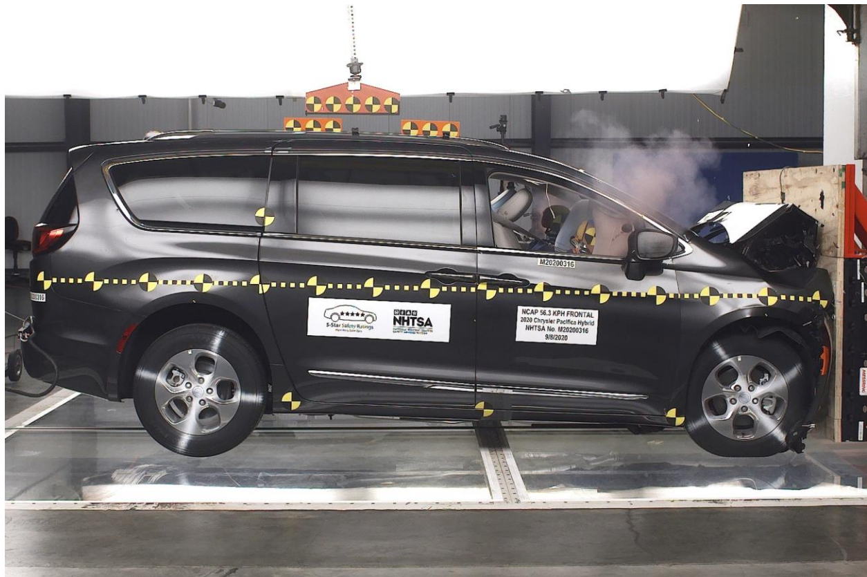
Figure A-82: 2020 Chrysler Pacifica Frontal Impact Event
