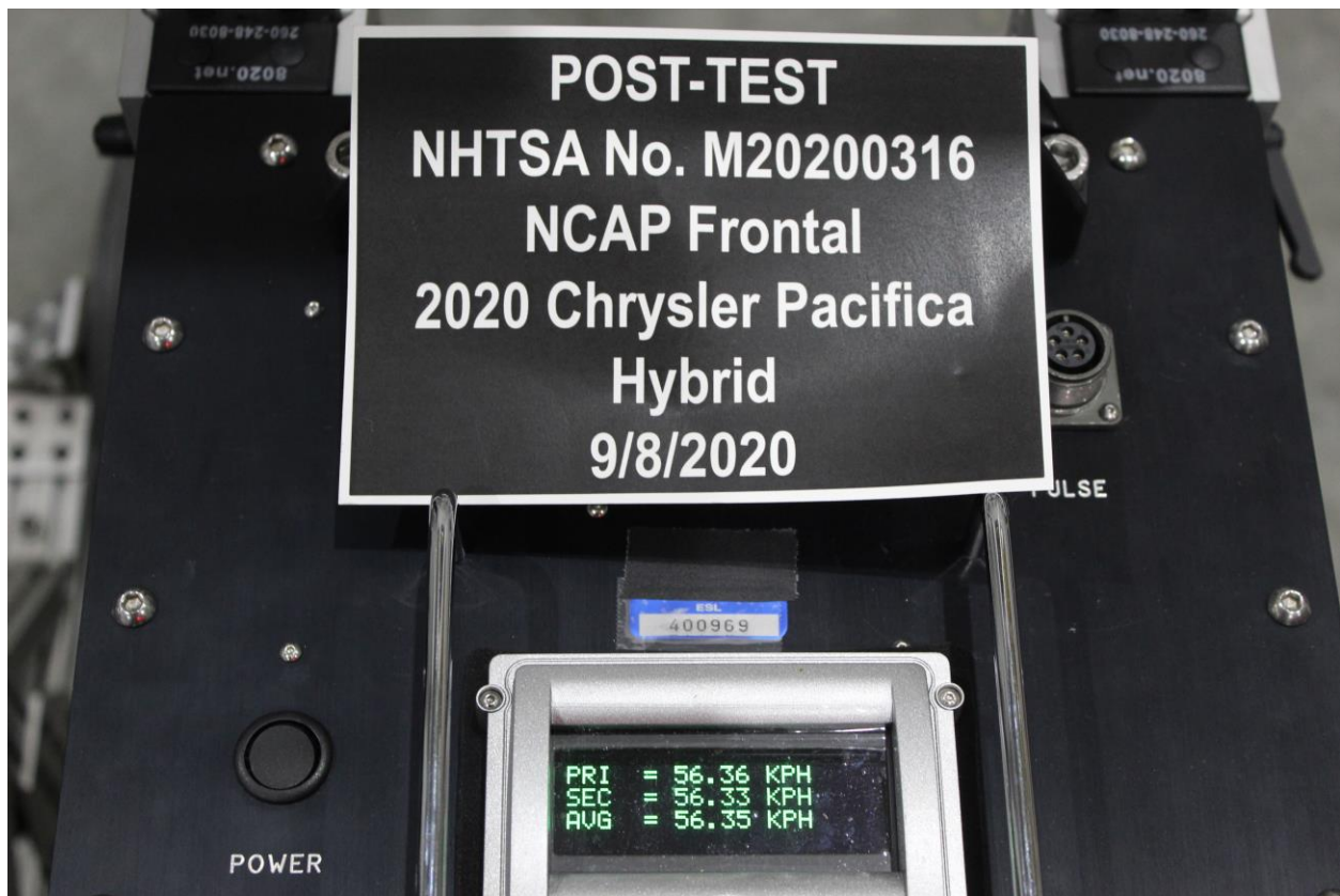
Figure A-76: Post-Test Speed Trap Read-Out
