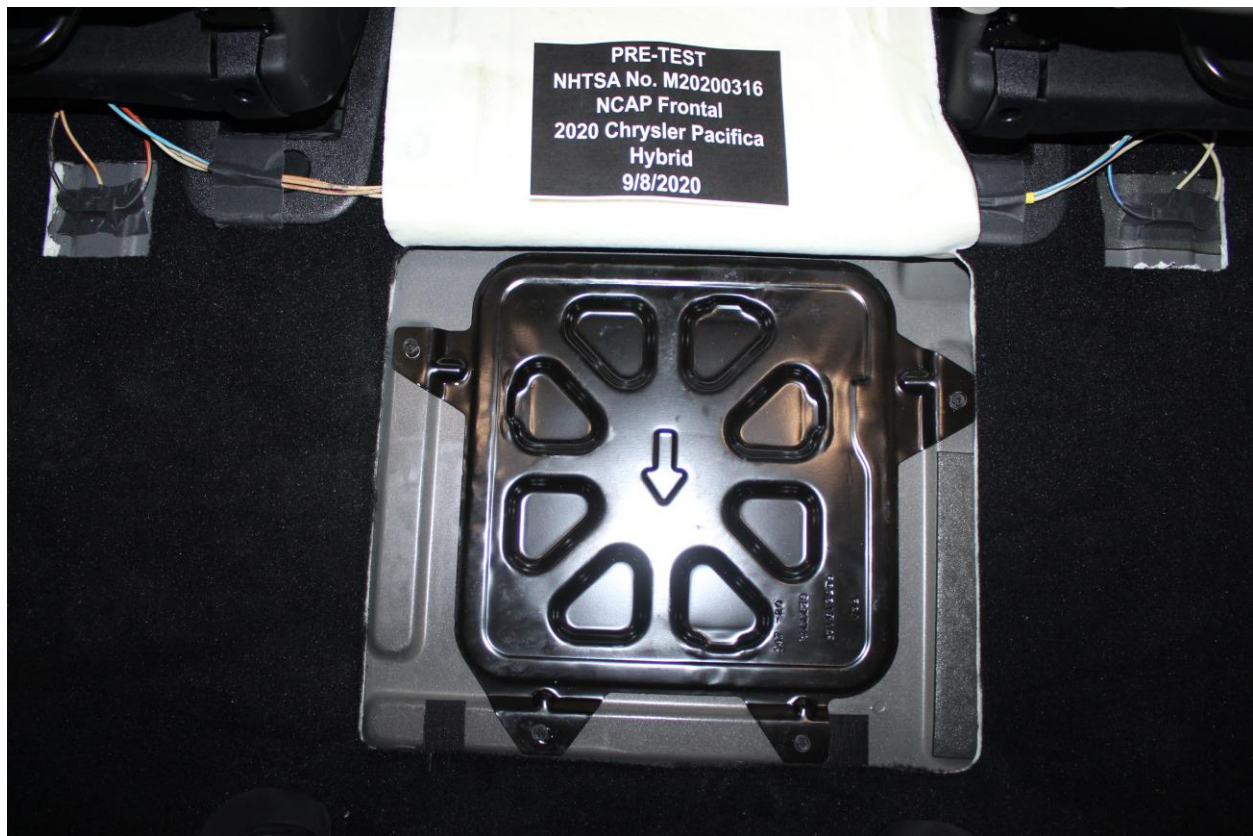
Figure 305-8: Manual High Voltage Service Disconnect Removed Location
