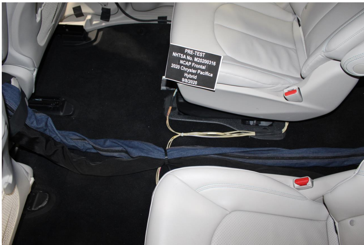
Figure A-28: Pre-Test Dummy Cable Routing
