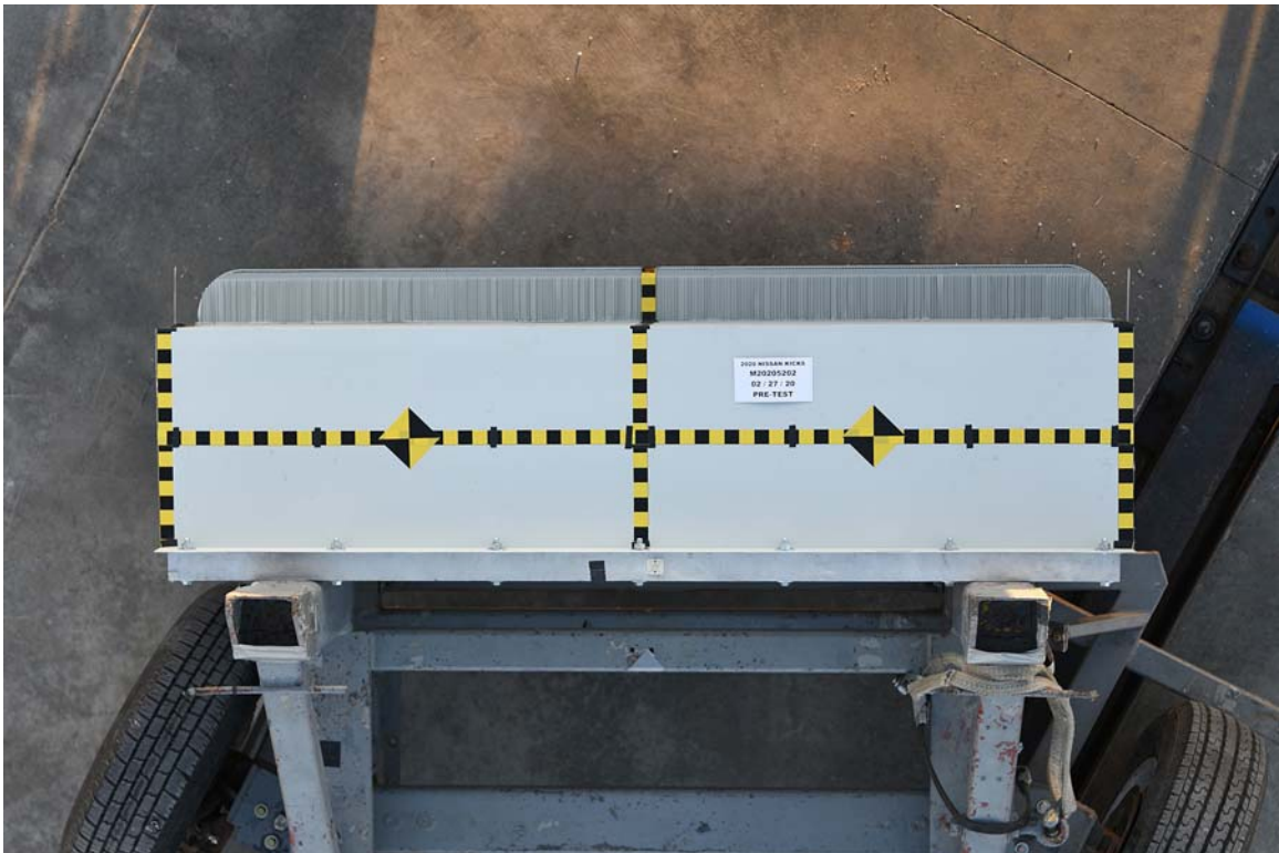
FIGURE 86. Pre-Test Top View of MDB Impactor Face
