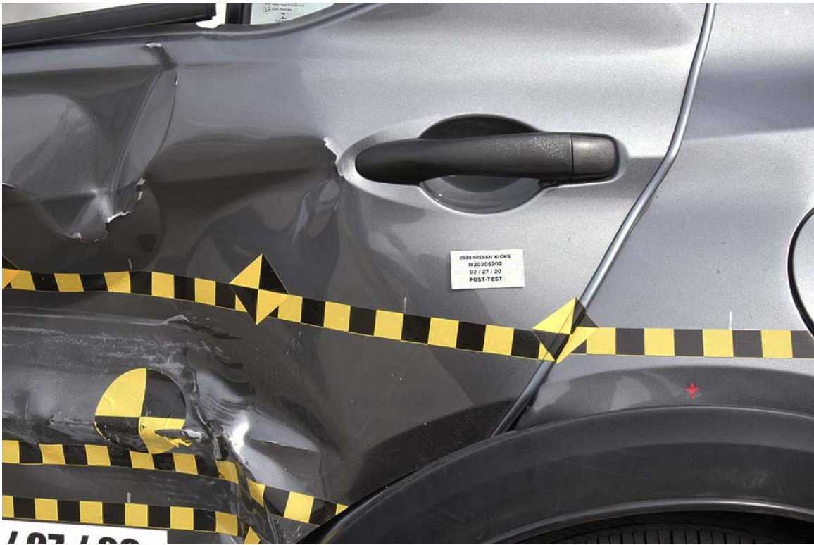
FIGURE 24. Post-Test Left Rear Door Latch Close-Up
