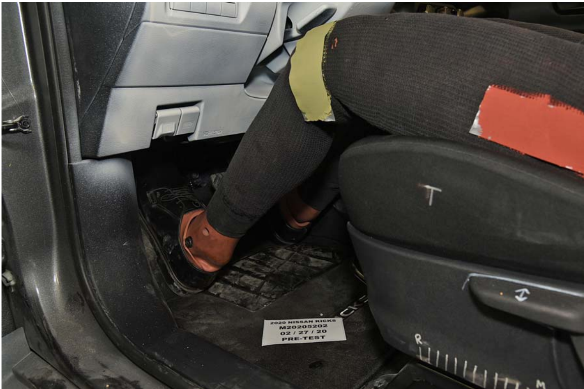
FIGURE 34. Pre-Test Placement of Driver Dummy's Feet
