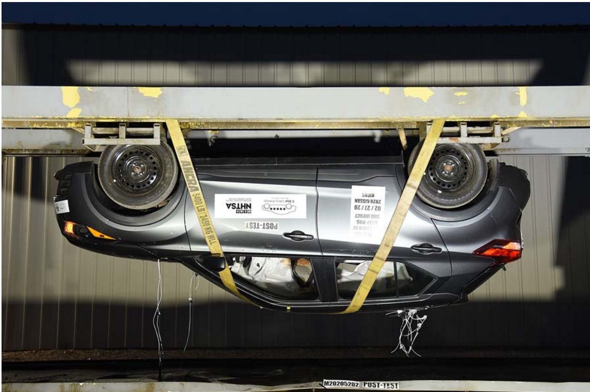
FIGURE 98. FMVSS No. 301 Static Rollover 180 Degrees
