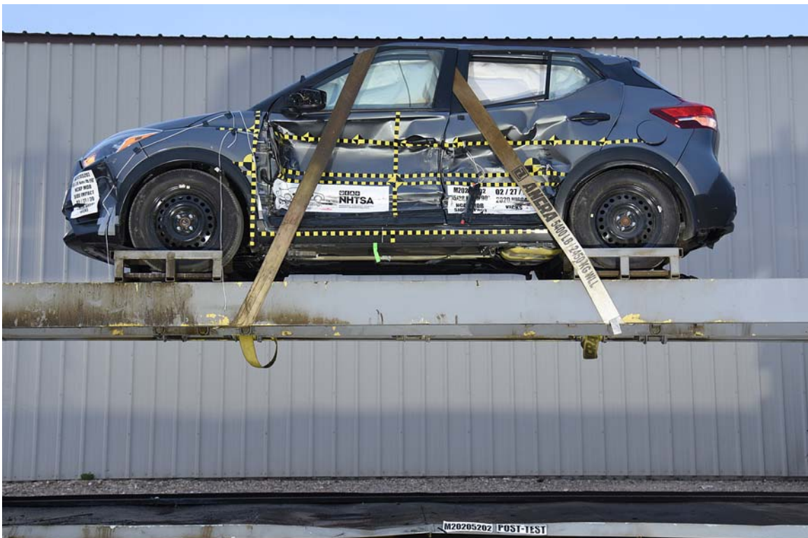
FIGURE 96. FMVSS No. 301 Static Rollover 0 Degrees
