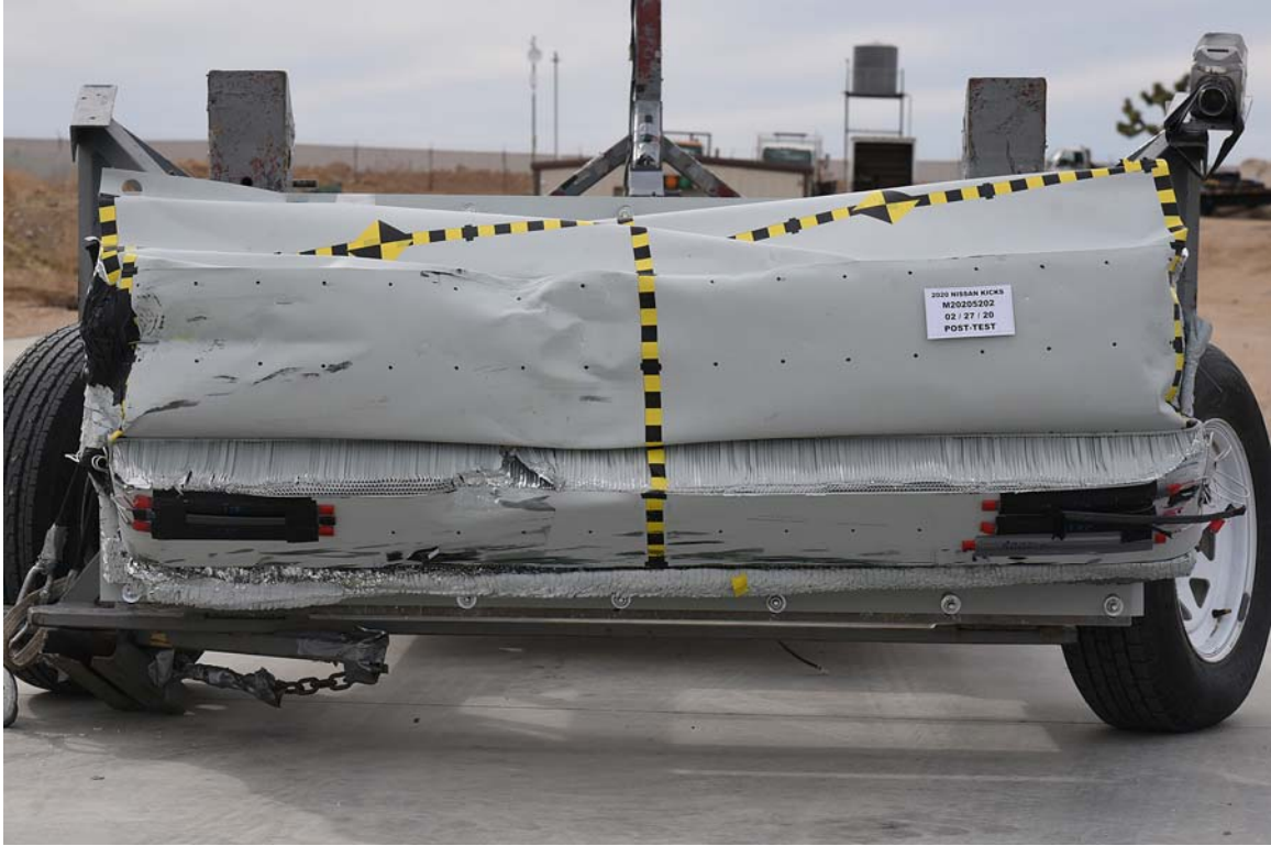
FIGURE 85. Post-Test Front View of MDB Impactor Face
