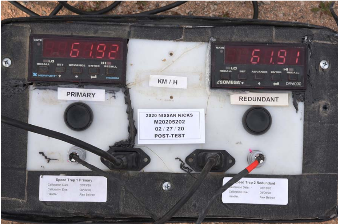
FIGURE 95. Post-Test Primary and Redundant Speed Trap Read-Out
