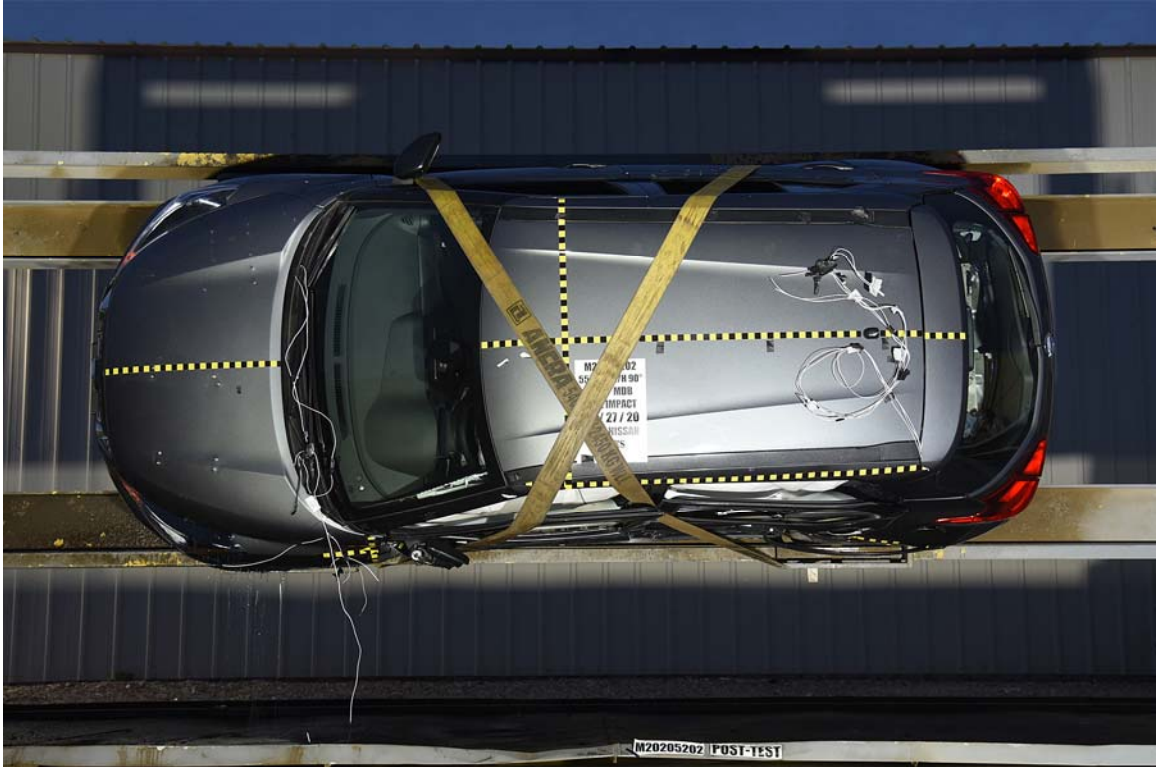
FIGURE 97. FMVSS No. 301 Static Rollover 90 Degrees
