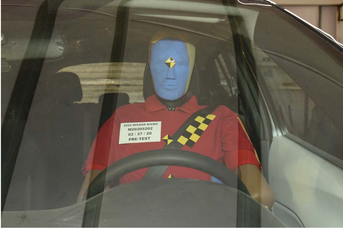
FIGURE 25. Pre-Test Front Close-Up View of Driver Dummy
