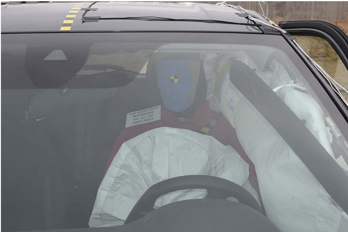
FIGURE 26. Post-Test Front Close-Up View of Driver Dummy
