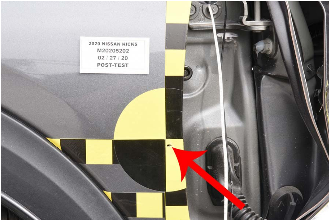
FIGURE 20. Post-Test Close-Up View of Impact Point Target
