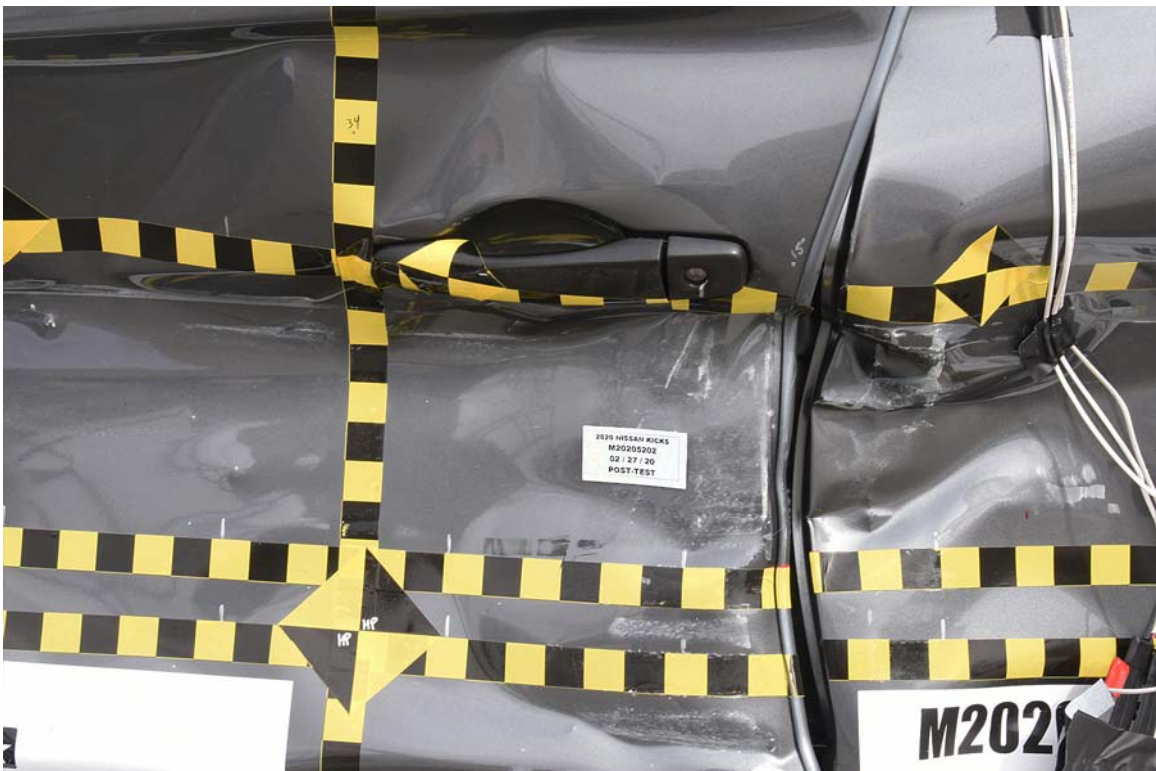
FIGURE 22. Post-Test Left Front Door Latch Close-Up
