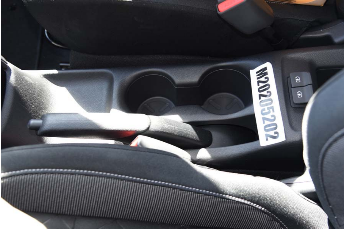
FIGURE 37. View of Disengaged Parking Brake
