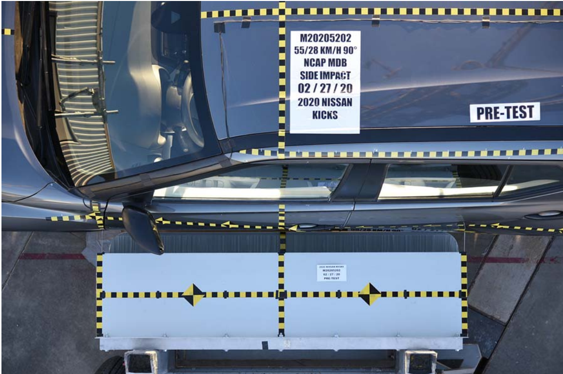
FIGURE 15. Pre-Test Overhead View of Test Area
