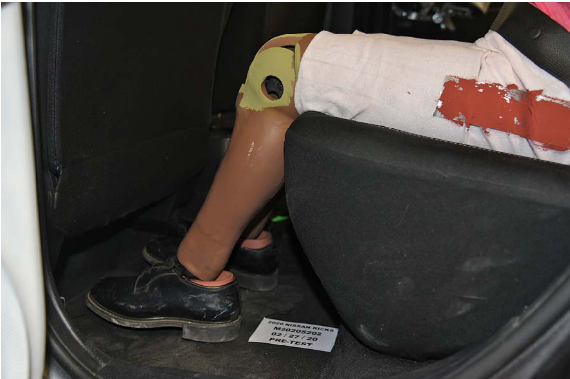
FIGURE 64. Pre-Test Placement of Rear Passenger Dummy's Feet
