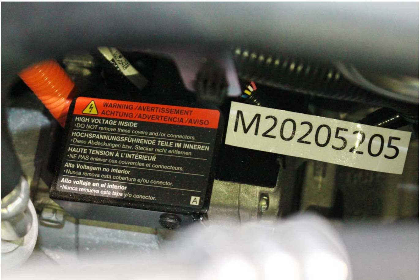
Photo No. 305-01 - Auxiliary Power Module Warning Label
