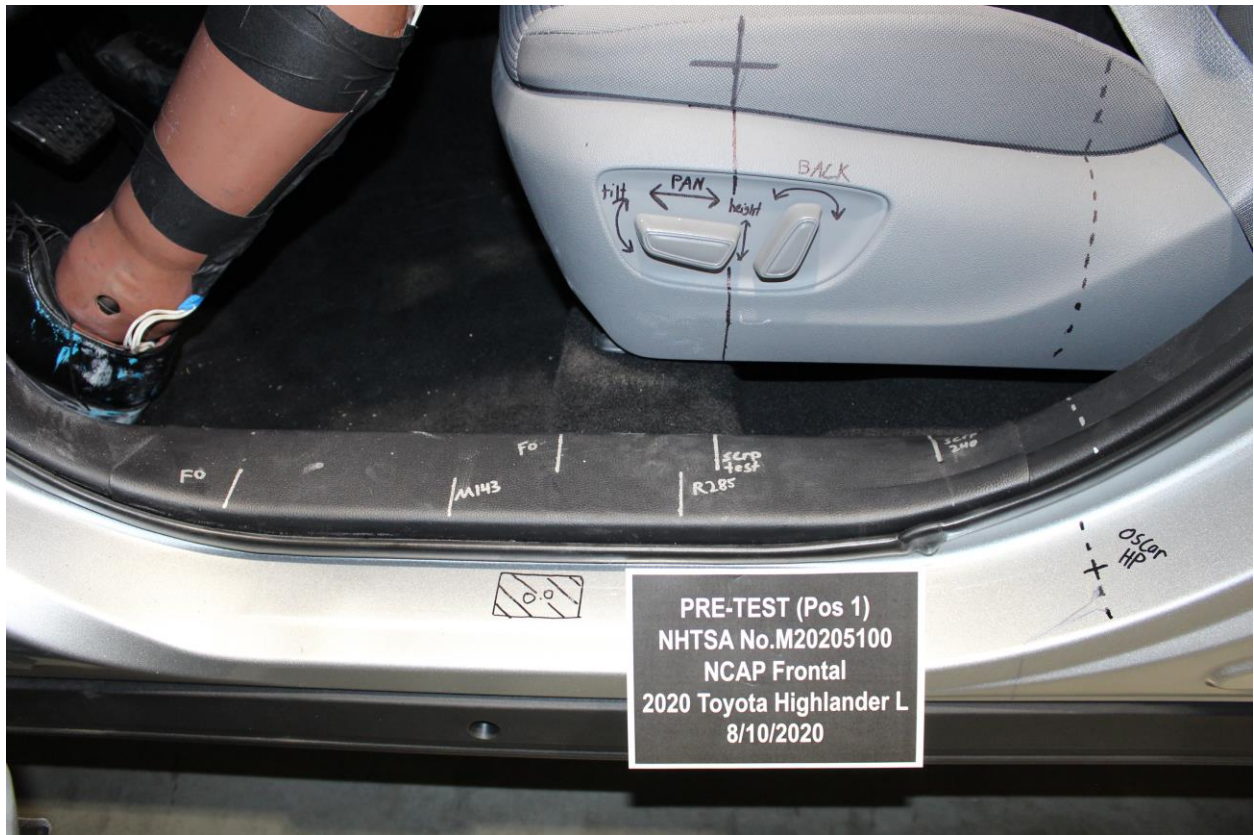
Figure A-36: Pre-Test Driver's Seat Fore-Aft Markings
