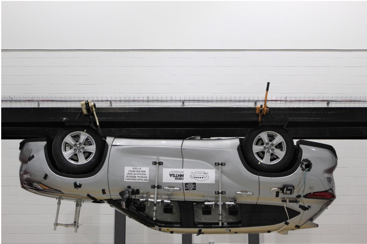
Figure A-98: FMVSS No. 301 Static Rollover 180 Degrees
