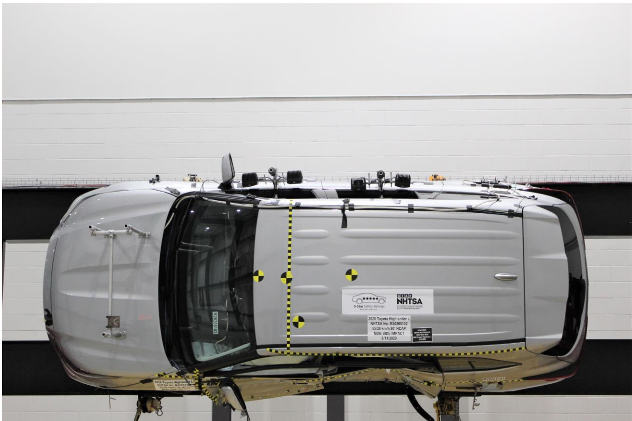
Figure A-97: FMVSS No. 301 Static Rollover 90 Degrees
