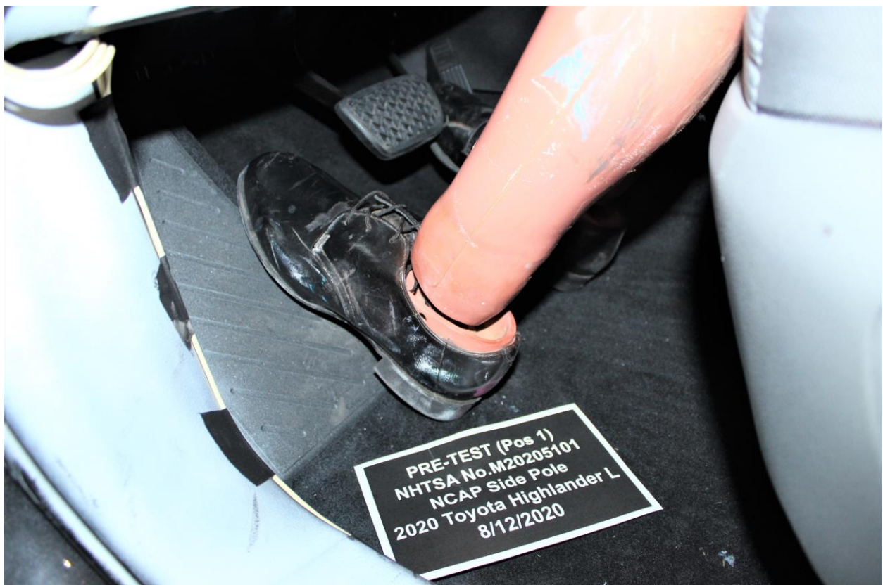
Figure A-32: Pre-Test Placement of Dummy's Feet
