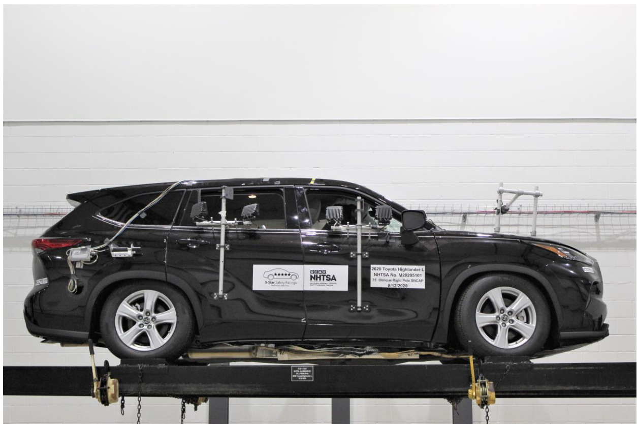
Figure A-63: FMVSS No. 301 Static Rollover 0 Degrees
