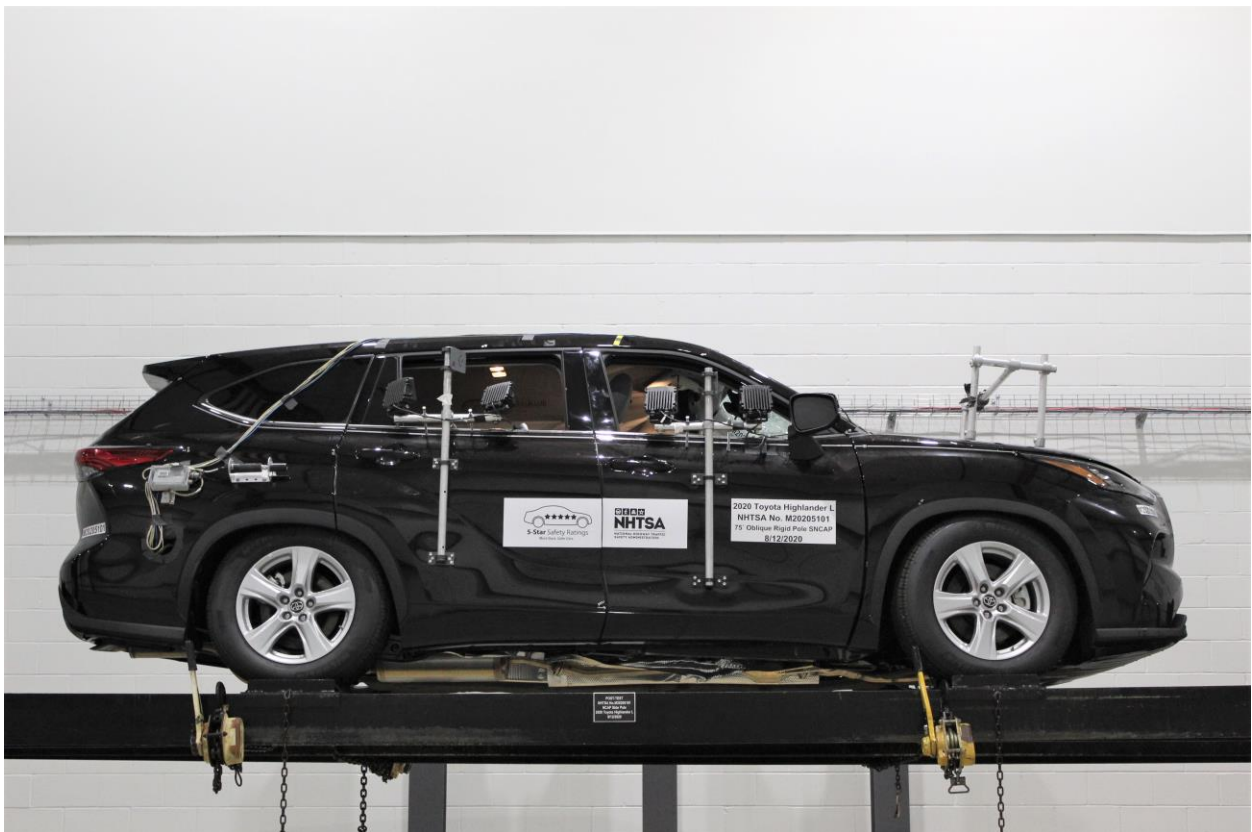
Figure A-67: FMVSS No. 301 Static Rollover 360 Degrees
