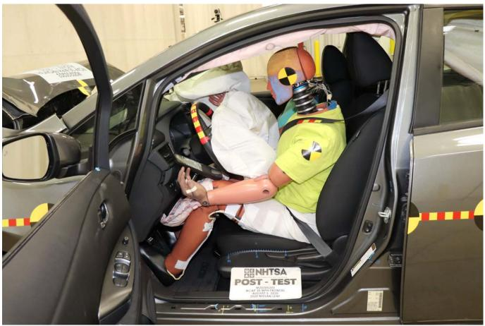
Photo No. 035 - Post-Test Driver Dummy and Vehicle Interior
