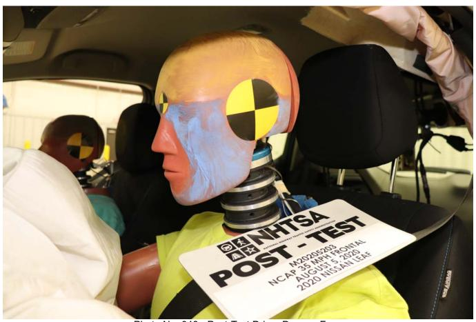
Photo No. 048 - Post-Test Driver Dummy Face
