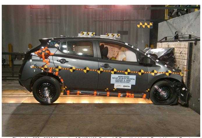
Photo No. 082 - 2020 Nissan Leaf S (40 kWh Battery) 5-Door Hatchback Frontal Impact Event
