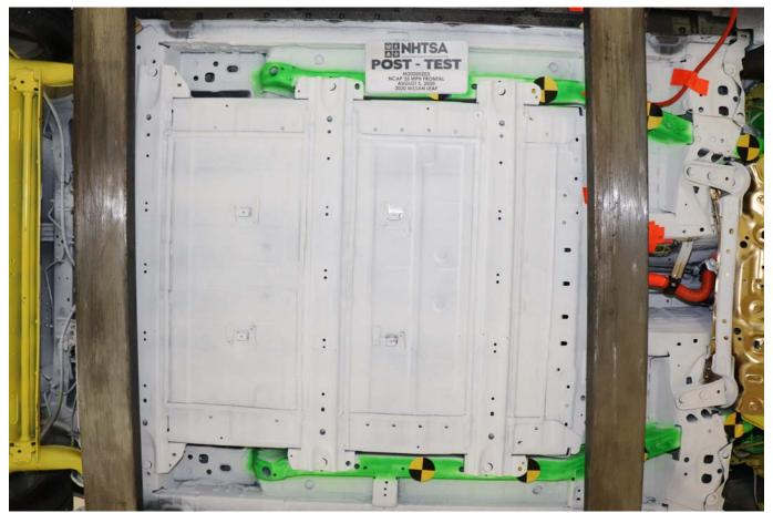
Photo No. 305-36 - Post-Impact View of Battery Module Movement or Retention Loss
