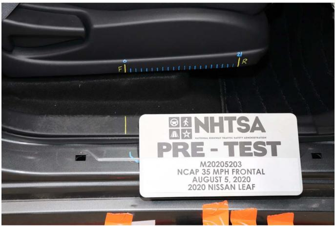
Photo No. 059 - Pre-Test Passenger Seat Fore-Aft Markings
