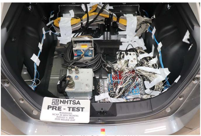
Photo No. 074 - Ballast Installed in Vehicle
