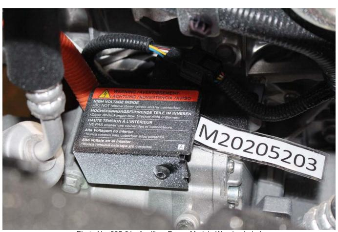
Photo No. 305-01 - Auxiliary Power Module Warning Label
