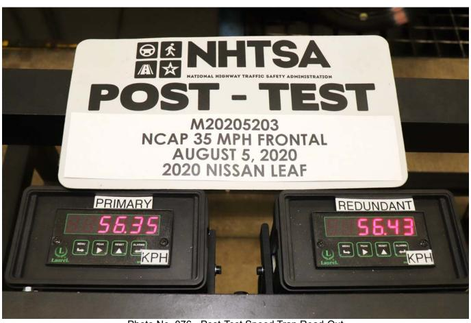
Photo No. 076 - Post-Test Speed Trap Read-Out
