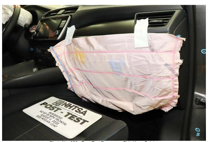
Photo No. 068 - Post-Test Passenger Side Knee Bolster
