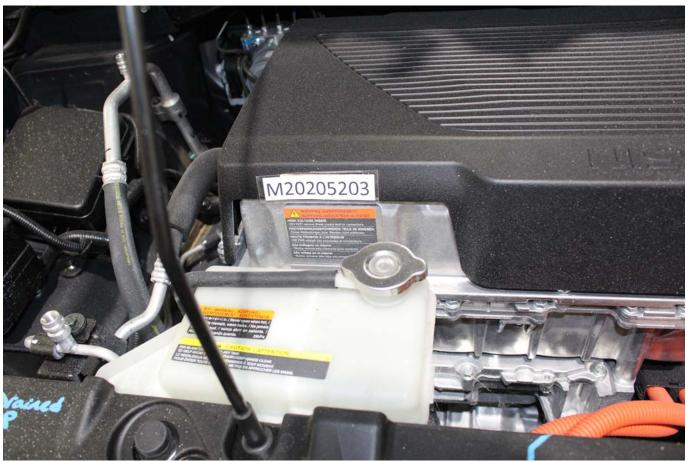
Photo No. 305-02 - Power Inverter Warning Label
