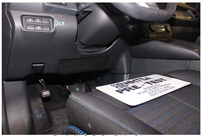
Photo No. 044 - Pre-Test Driver Side Knee Bolster
