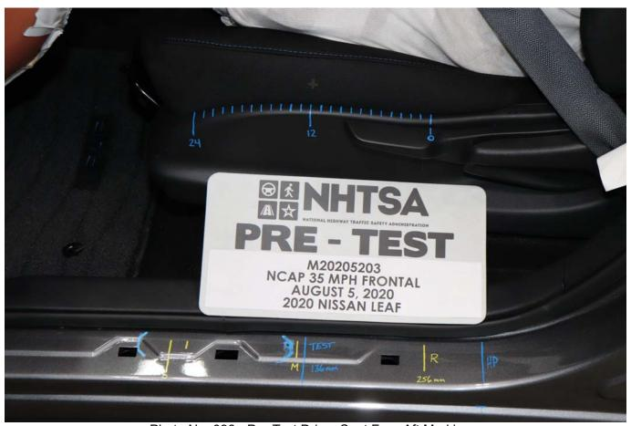
Photo No. 036 - Pre-Test Driver Seat Fore-Aft Markings
