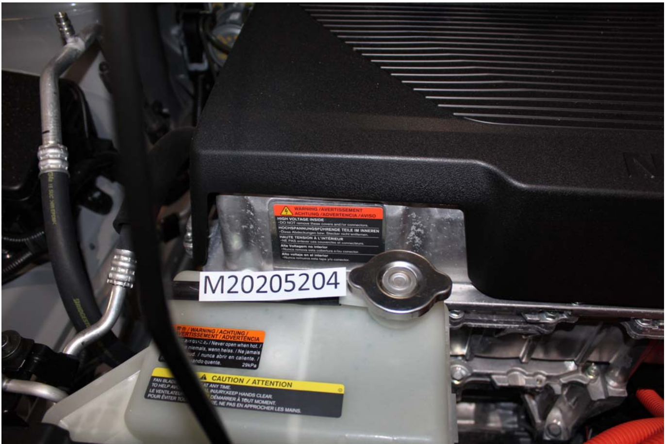
Photo No. 305-02 - Power Inverter Warning Label
