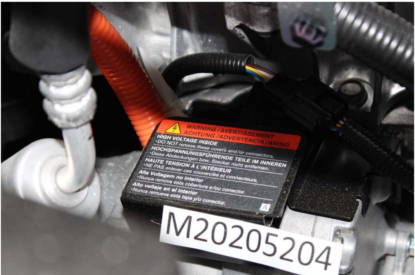
Photo No. 305-01 - Auxiliary Power Module Warning Label
