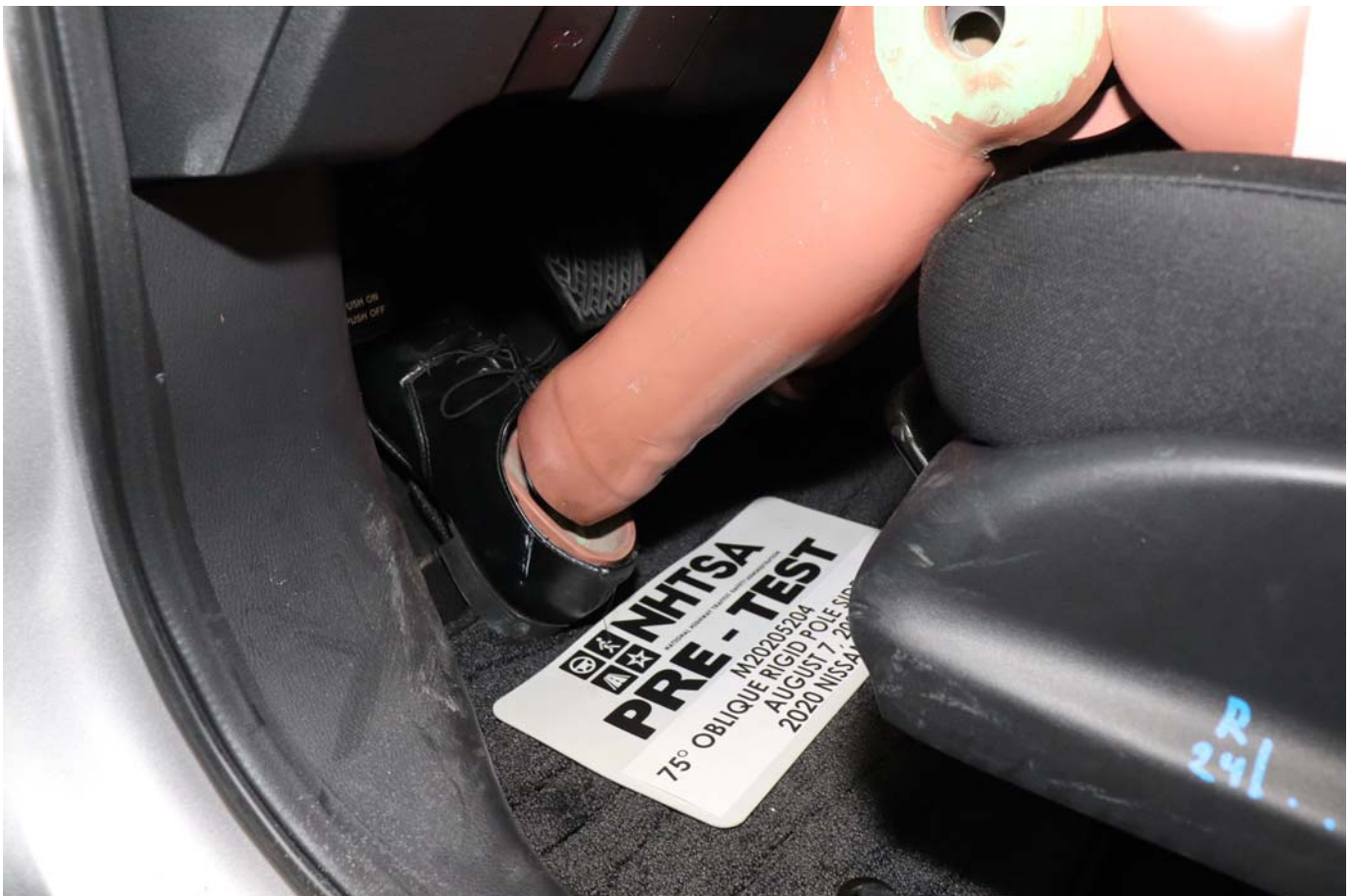
Photo No. 032 - Pre-Test Placement of Dummy Feet
