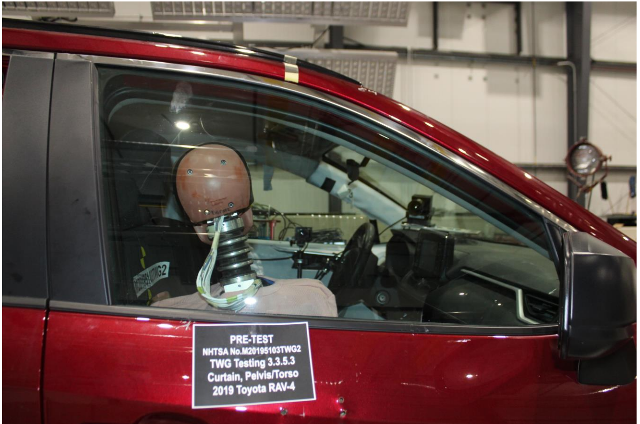
Figure A-11: Pre-Test SID-IIs Right Side View
