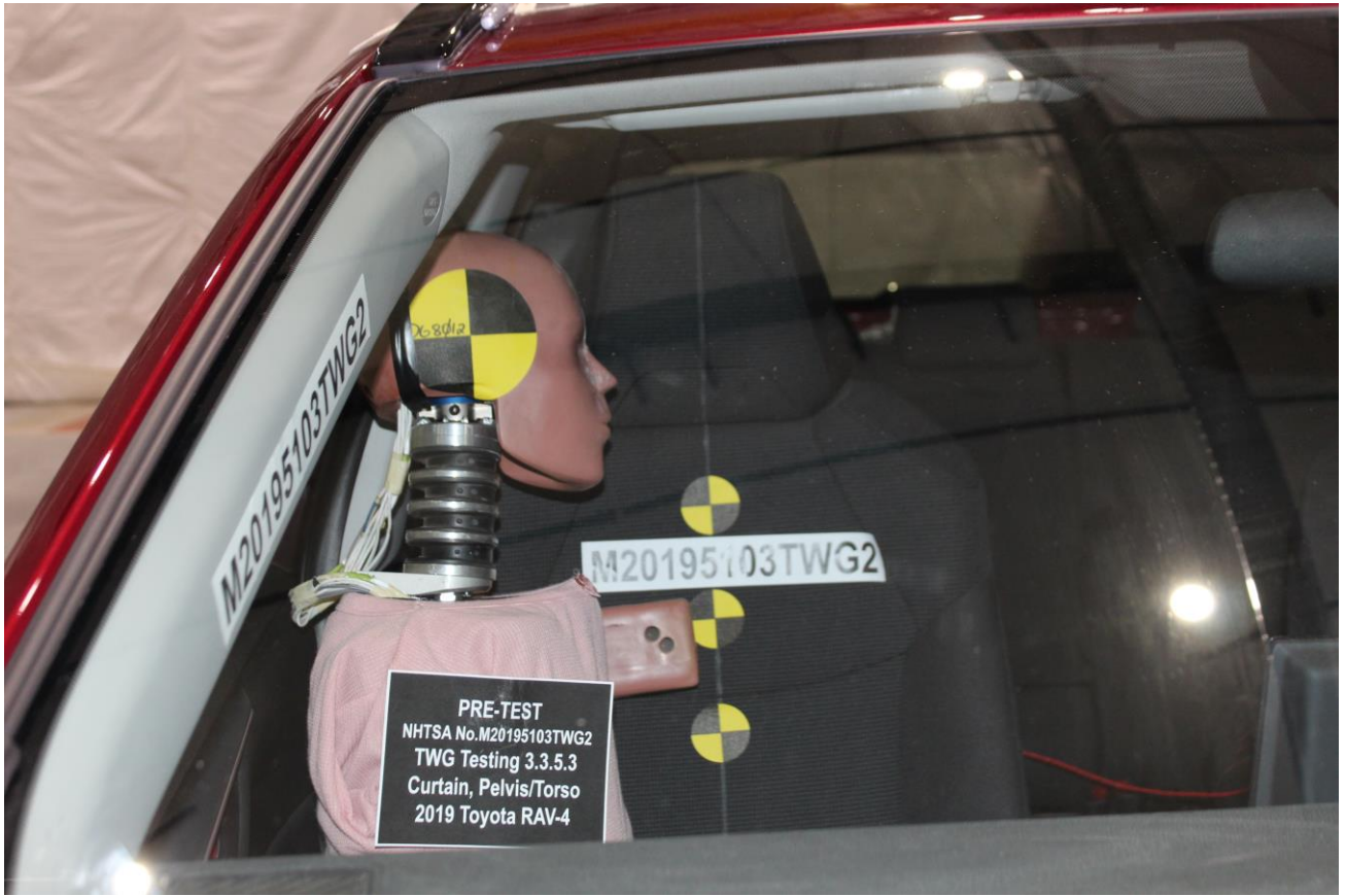
Figure A-7: Pre-Test SID-IIs Front View
