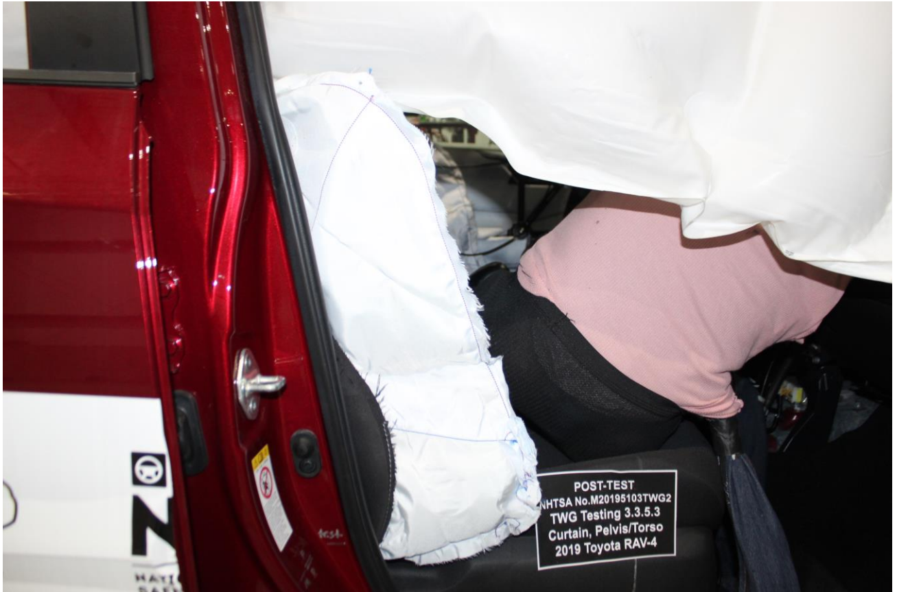
Figure A-14: Post-Test Seat Airbag View
