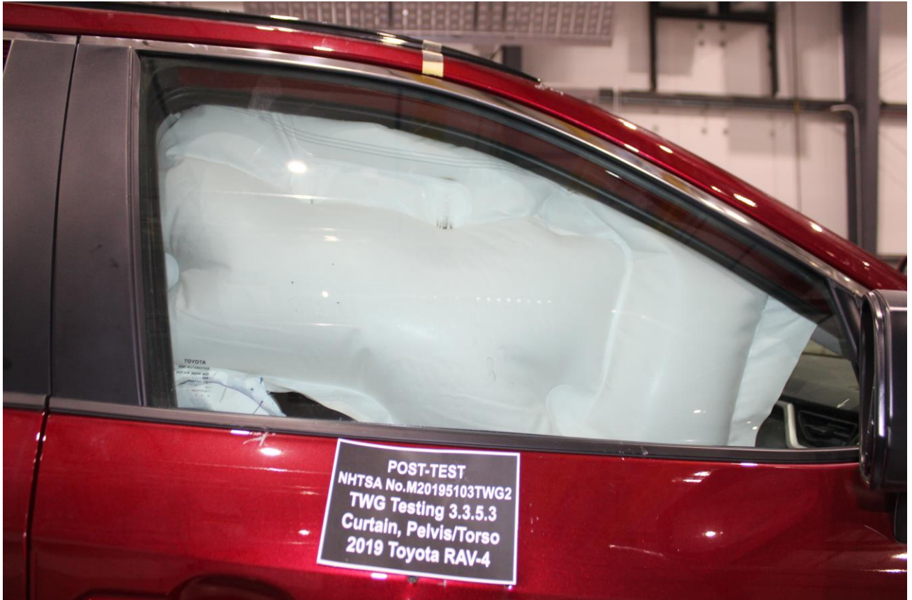
Figure A-12: Post-Test SID-IIs Right Side View
