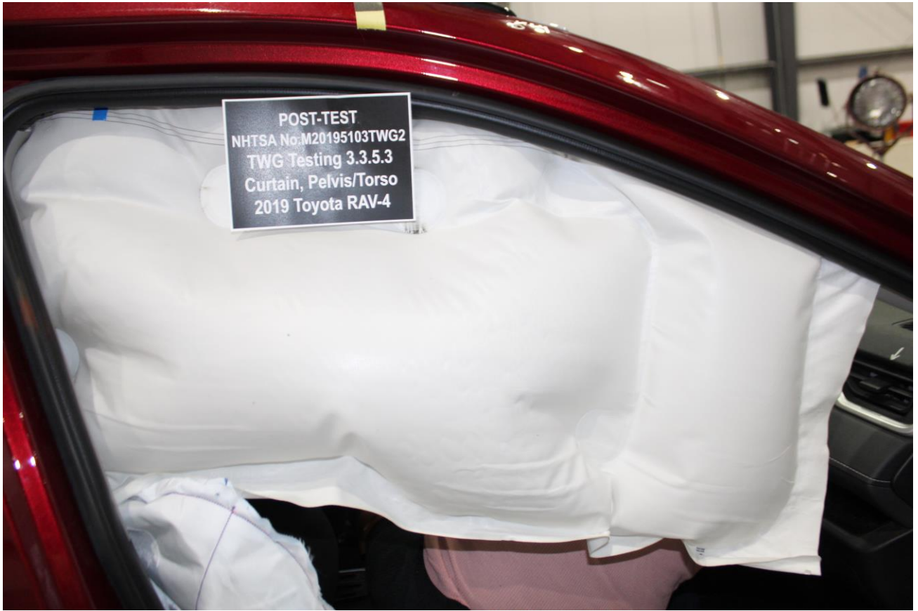
Figure A-13: Post-Test Curtain Airbag View
