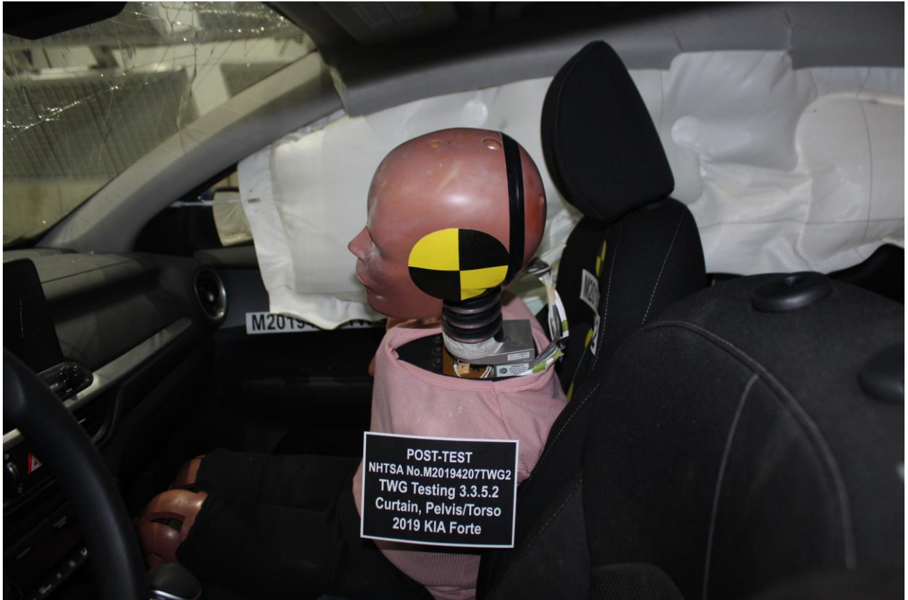
Figure A-4: Post-Test SID-IIs Left Side View
