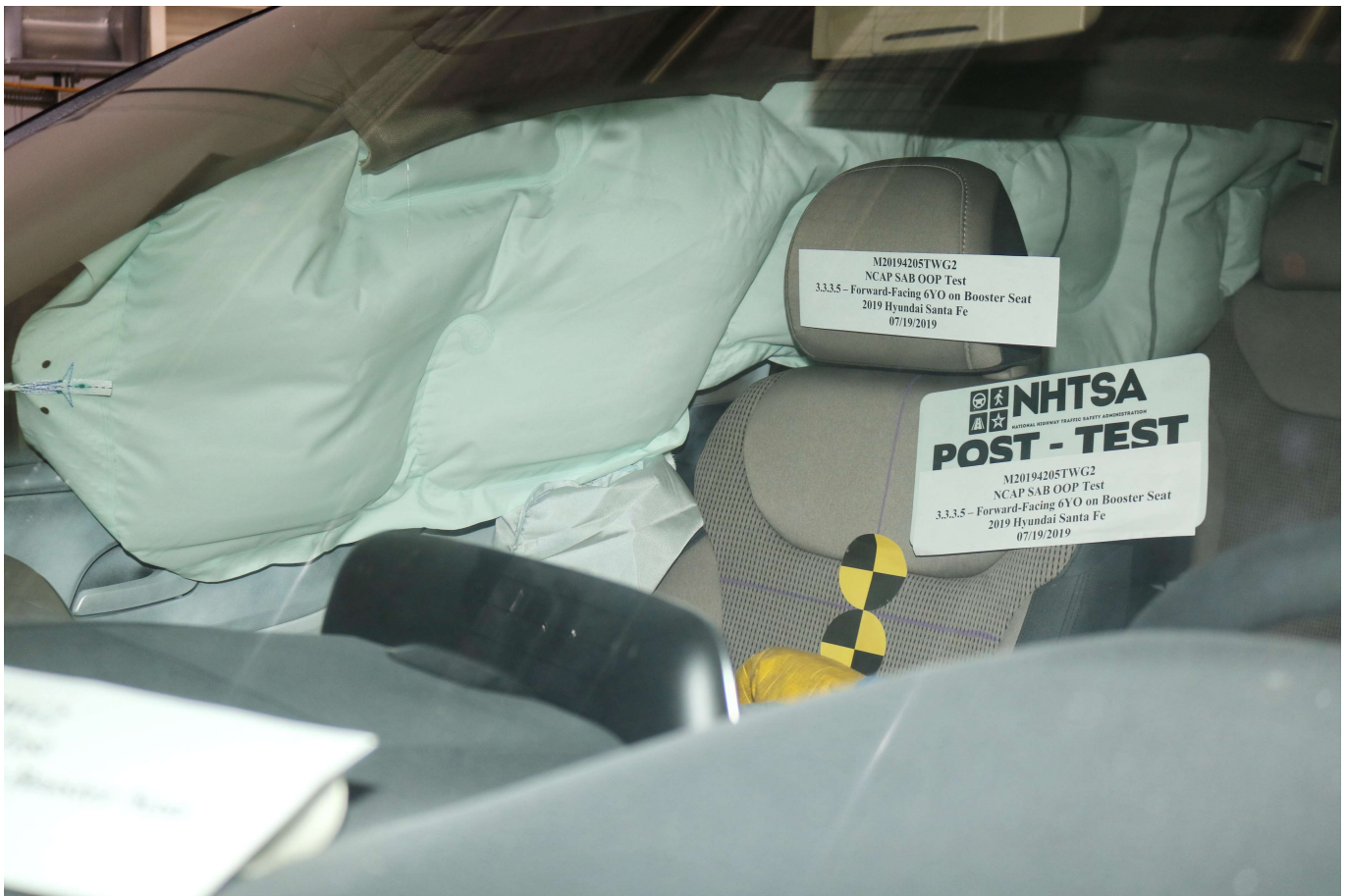
Photo No. 027 - Post-Test Curtain Air Bag Left Three-Quarter Front View
