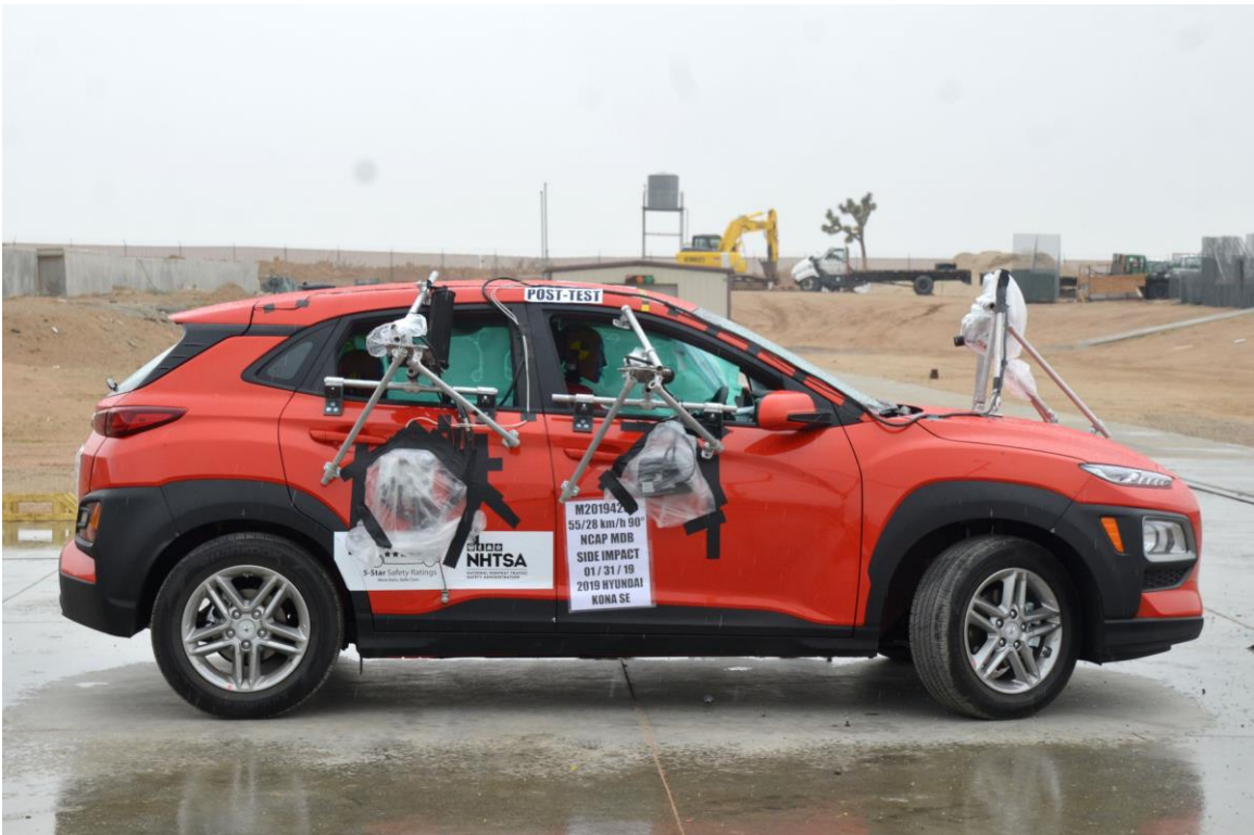
FIGURE 6. Post-Test Right Side View of NCAP Side MDB Impact Test
