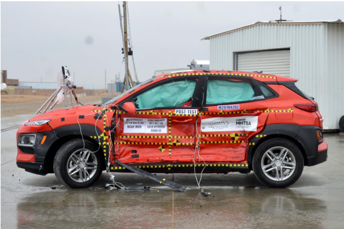
FIGURE 4. Post-Test Left Side View of NCAP Side MDB Impact Test
