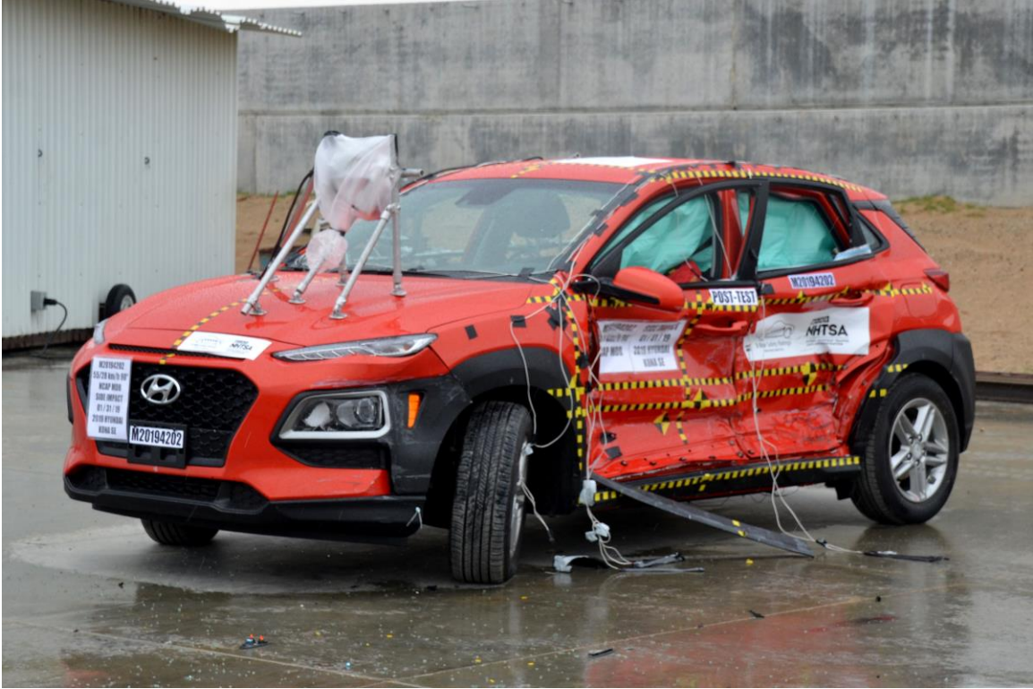
FIGURE 3. Post-Test Left Front 3/4 View of NCAP Side MDB Impact Test
