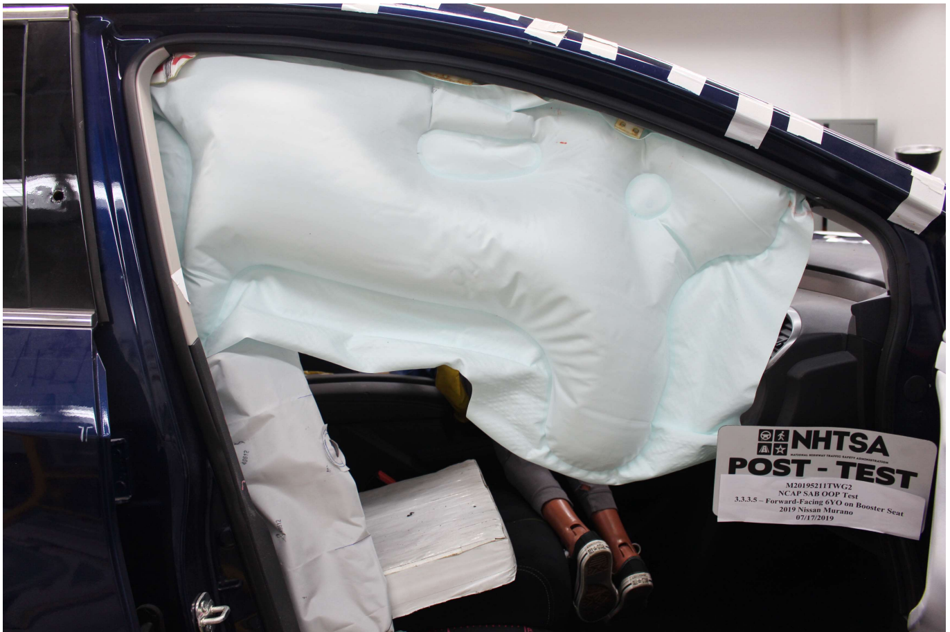
Photo No. 029 - Post-Test Curtain Air Bag Right Side View (Door Open)
