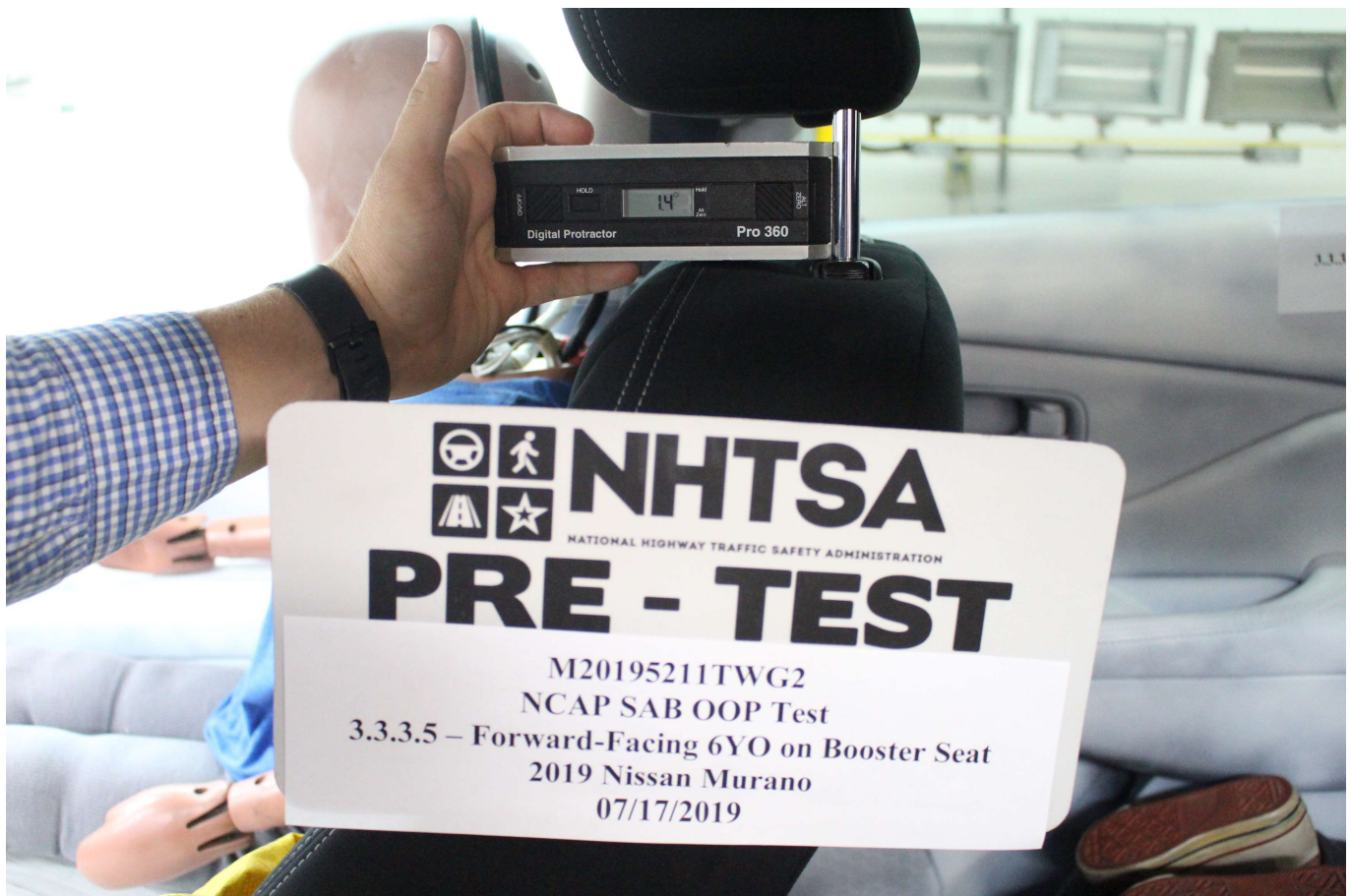
Photo No. 008 - Pre-Test Vehicle Seat Back Angle
