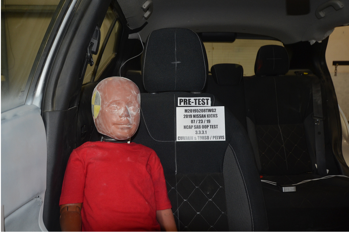
FIGURE 13. Pre-Test Dummy Position, Close-Up Front View
