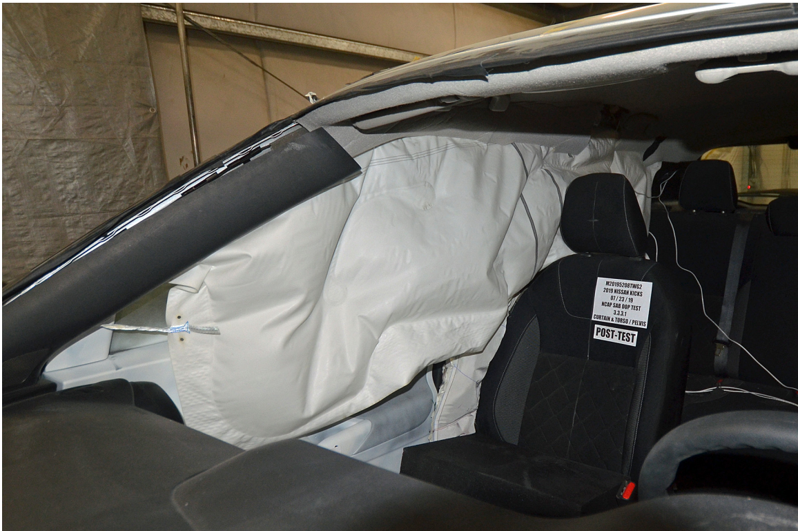
FIGURE 18. Post-Test Airbags, Left Front \frac{3}{4} View
