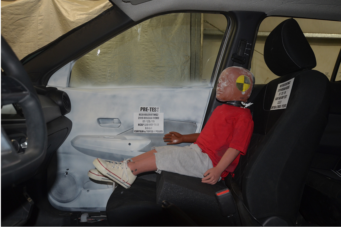
FIGURE 7. Pre-Test Dummy Position, Left View
