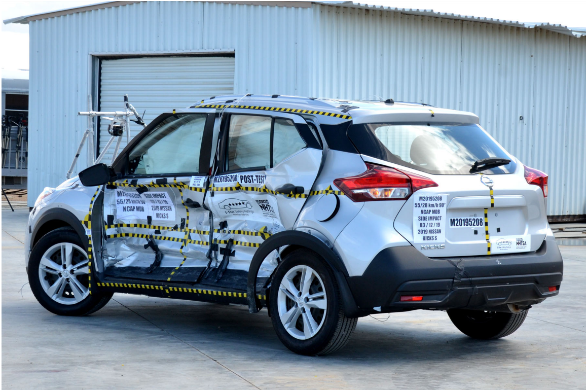
FIGURE 5. Post-Test Left Rear \frac{3}{4} View of NCAP Side MDB Impact Test
