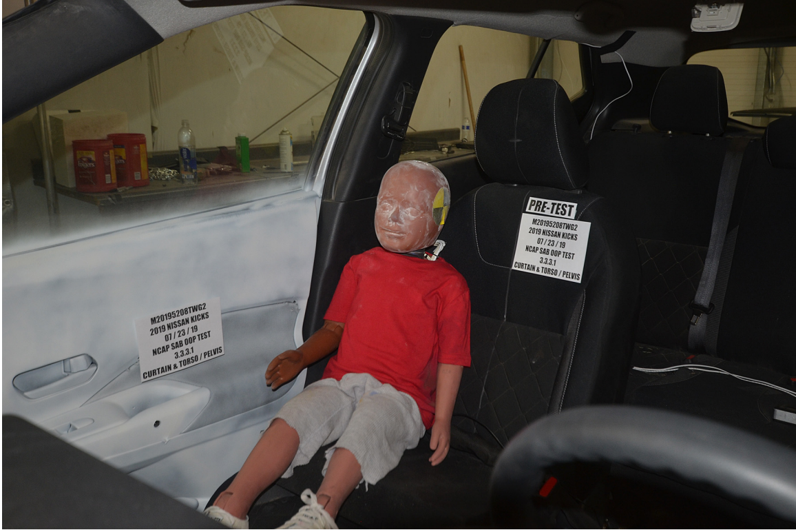
FIGURE 9. Pre-Test Dummy Position, \frac{3}{4} View
