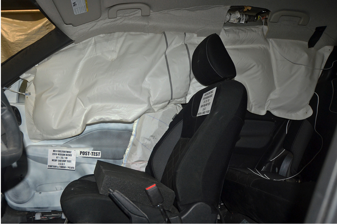
FIGURE 17. Post-Test Airbags, Left Side View
