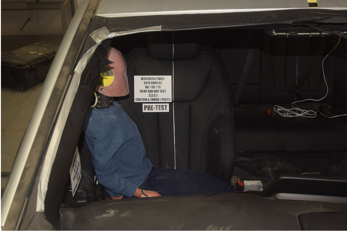
FIGURE 13. Pre-Test Dummy Position, Close-Up Front View
