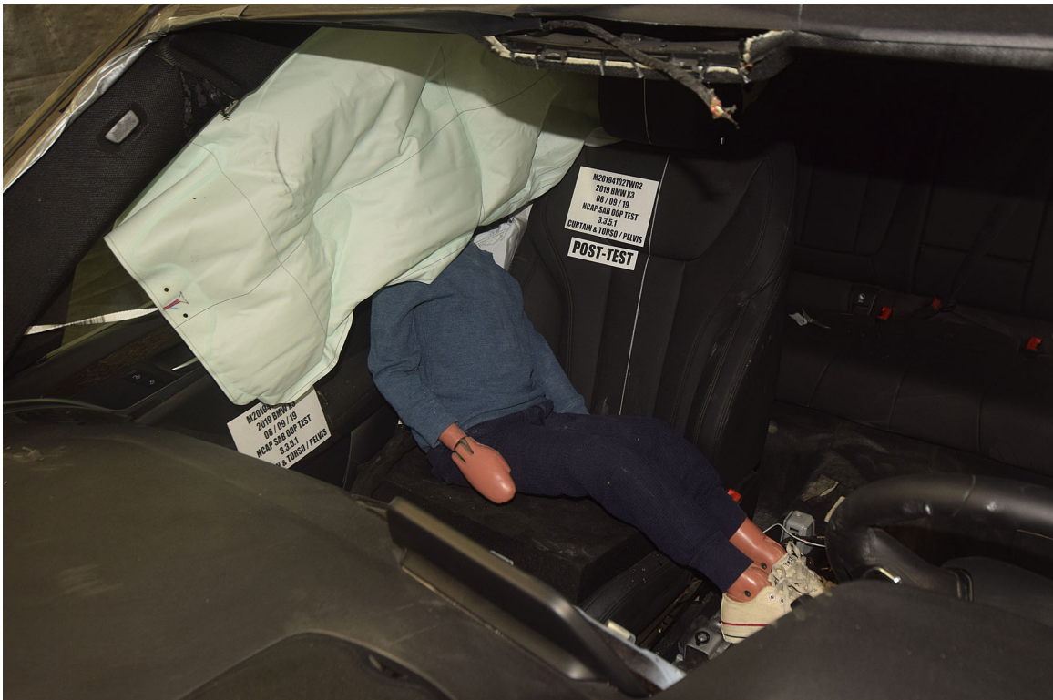
FIGURE 10. Post-Test Dummy Position, \frac{3}{4} View
