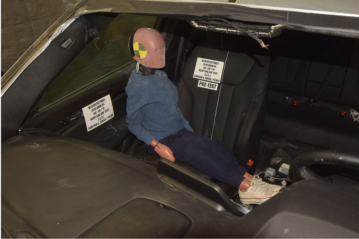
FIGURE 9. Pre-Test Dummy Position, \frac{3}{4} View
