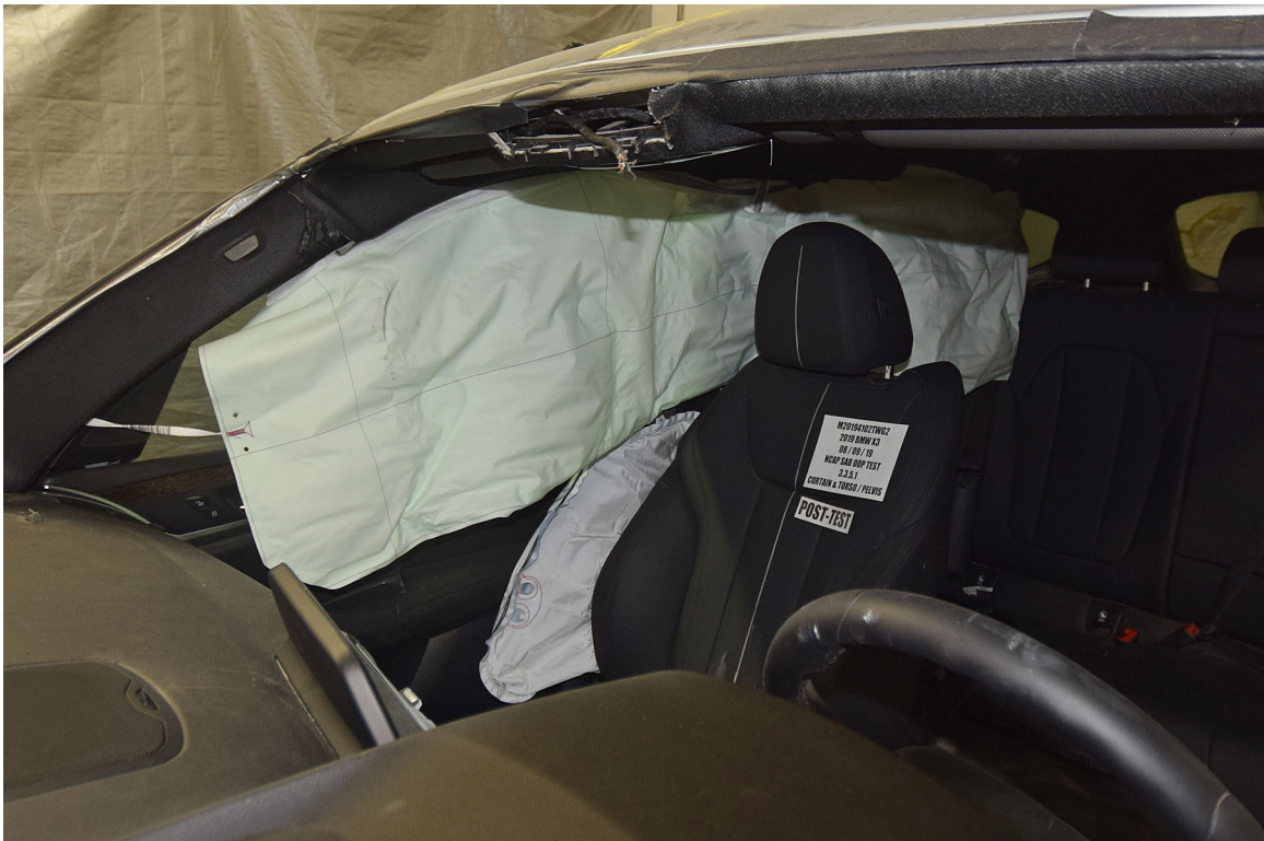
FIGURE 18. Post-Test Airbags, Left Front \frac{3}{4} View
