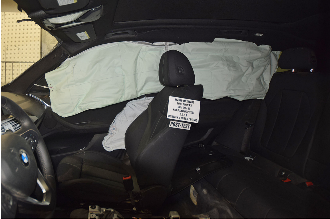
FIGURE 17. Post-Test Airbags, Left Side View
