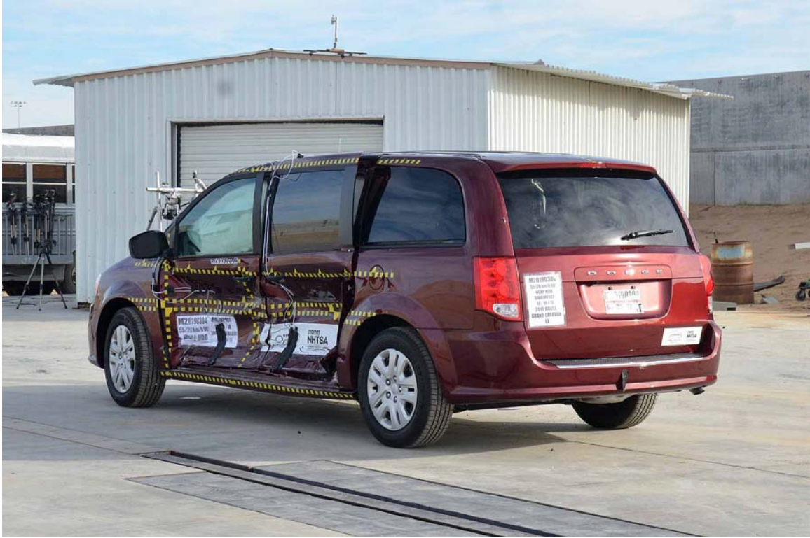
FIGURE 5. Post-Test Left Rear 3/4 View of NCAP Side MDB Impact Test
