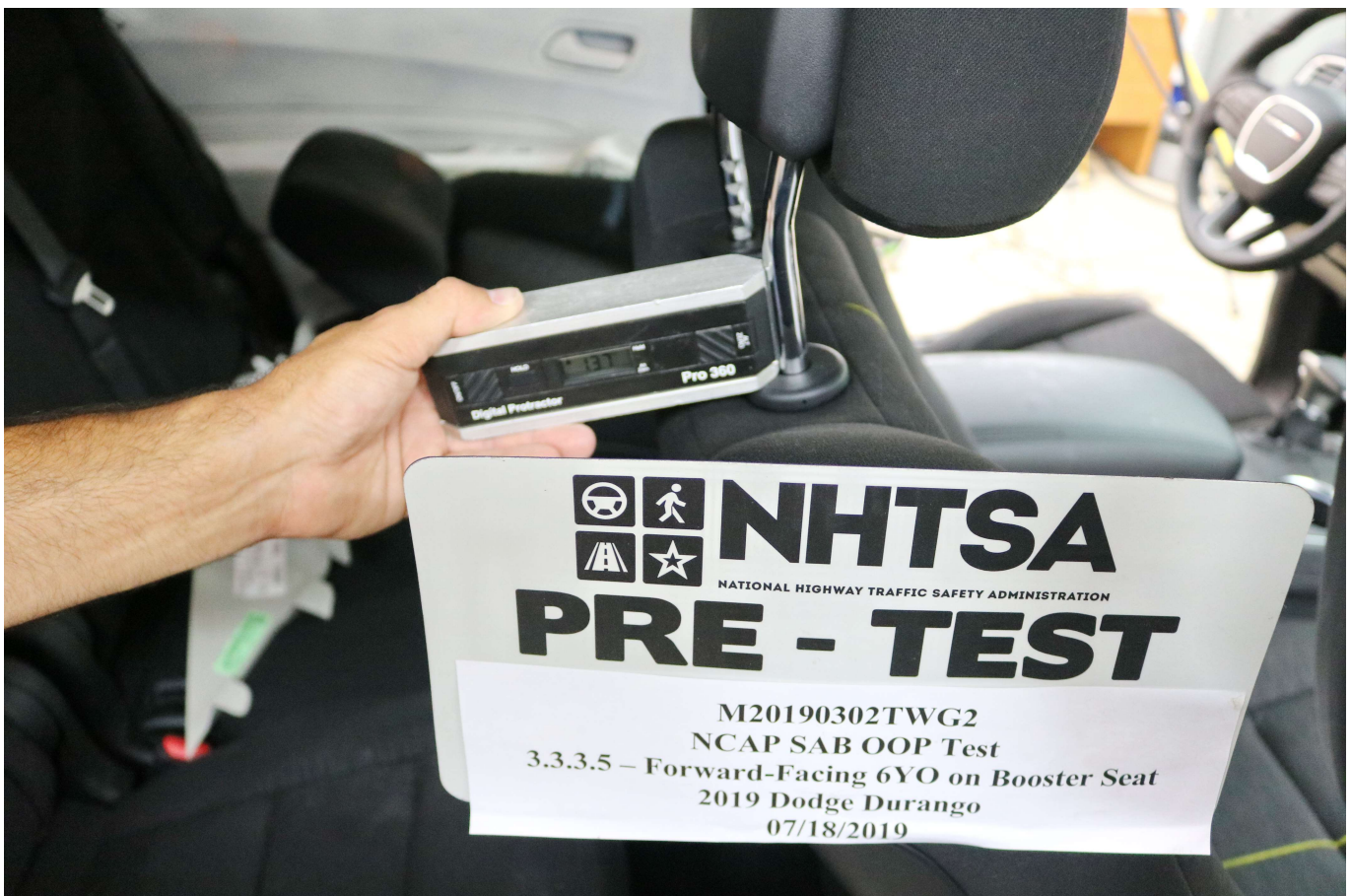
Photo No. 008 - Pre-Test Vehicle Seat Back Angle
