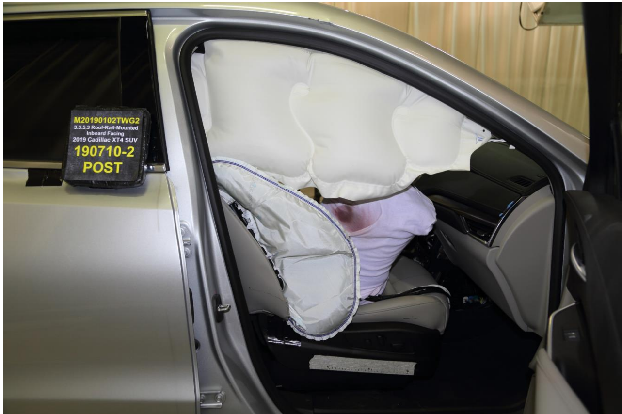
Figure A-25 Post-Test Dummy Right Side Front View
