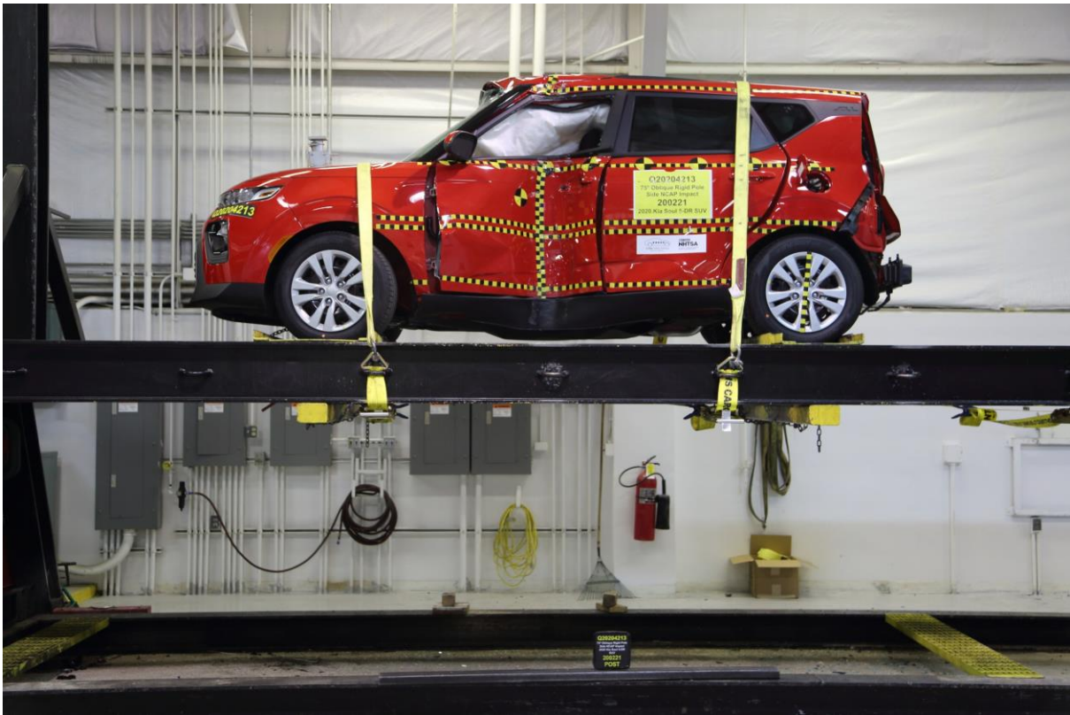
No. 067 FMVSS No. 301 Static Rollover 360 Degrees
