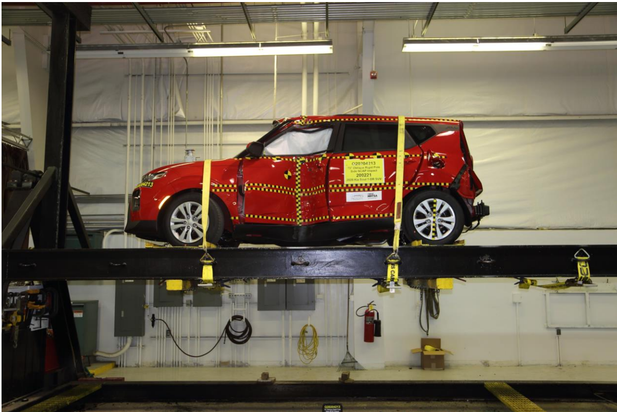
No. 063 FMVSS No. 301 Static Rollover 0 Degrees
