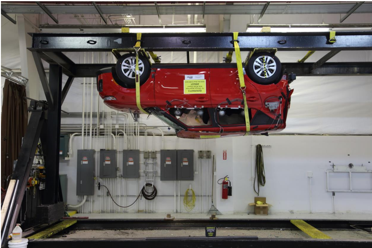
No. 065 FMVSS No. 301 Static Rollover 180 Degrees
