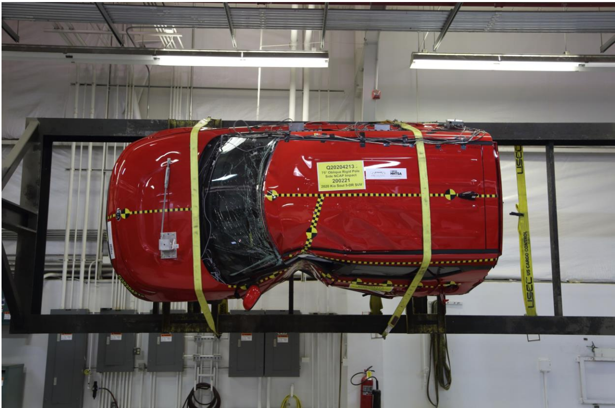
No. 064 FMVSS No. 301 Static Rollover 90 Degrees
