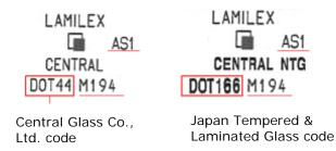
As such, the windshield glass panes produced with a valid, but incorrect manufacturer certification code mark do not meet the requirements of Paragraph S6.2 of FMVSS no. 205: Glazing materials. The subject windshield glass panes meet all other requirements of FMVSS no. 205.
