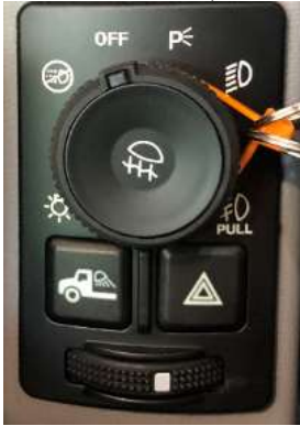
Illustration 2: (Incorrect symbol used for marker lamp position)
