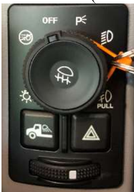
Illustration 2: (Incorrect symbol used for marker lamp position)
