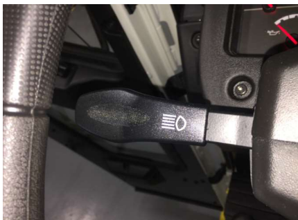
Illustration 4: (Turn signal switch not identified with required symbol)
