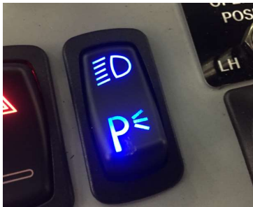
Illustration 4: (Turn signal switch not identified with required symbol)
