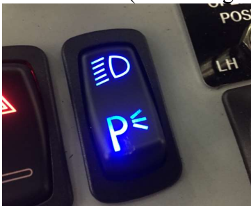
Illustration 3: (Master Lighting Switch not identified with required symbol or word).
