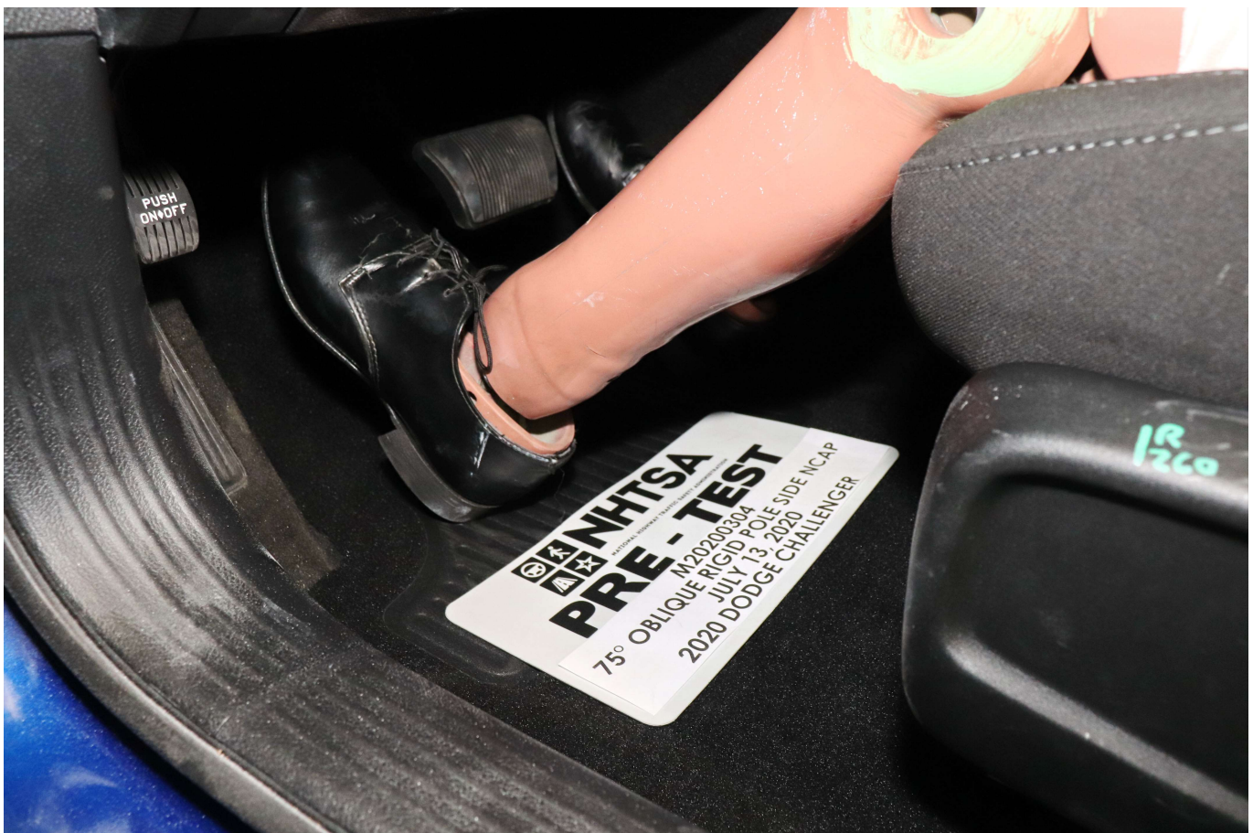
Photo No. 032 - Pre-Test Placement of Dummy Feet
